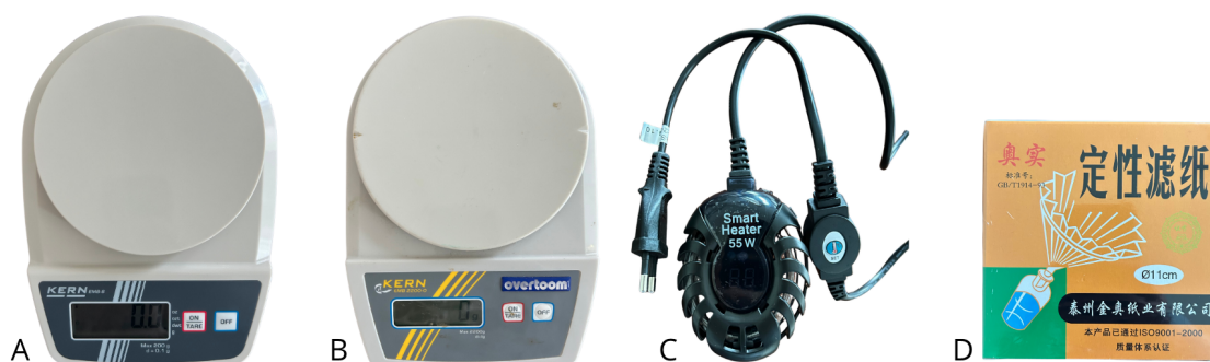
Figure 22: Overview of the equipment used for the absorption and rewet testing protocol. A: Digital precision scale (KERN EMB-S, \pm 0.1 g) used for blotting paper measurements, B: Digital scale (KERN EMB 2200-0, \pm 1 g) used for weighing dry and wet materials, C: Submersible Smart Heater (55 W) used to maintain a constant fluid temperature during testing, D: Ø11 cm qualitative filter paper (medium retention) used for assessing surface rewetting after fluid absorption.
