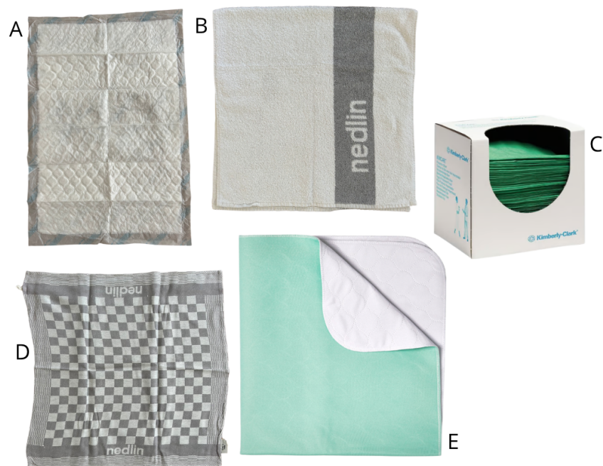
Figure 21: Materials tested for fluid absorption and rewetting properties. A: Disposable absorbent pad (40x60 cm), B: Towel (Nedlin), C: Kimberly-Clark Kleenex 7093 hygiene wipe, D: Tea towel (Nedlin), E: Washable absorbent underpad (85x90 cm, Nedlin).
