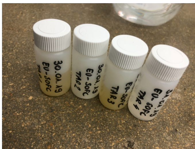
Figure 32 Tar samples taken upstream and downstream the GCU. The colors of the liquids indicate lower tar components after the GCU.
