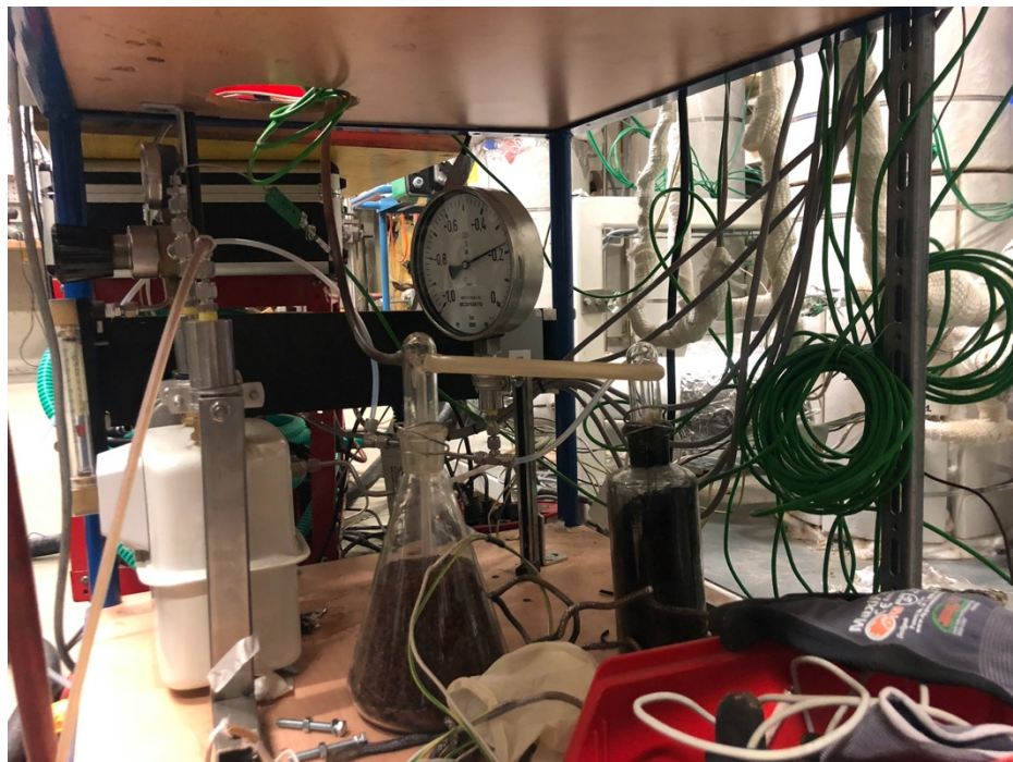
Figure 27 Lower level of the sampling train setup. Shown are the activated carbon filter, the silica gel, pressure gauge, flow totalizer and exhaust line
