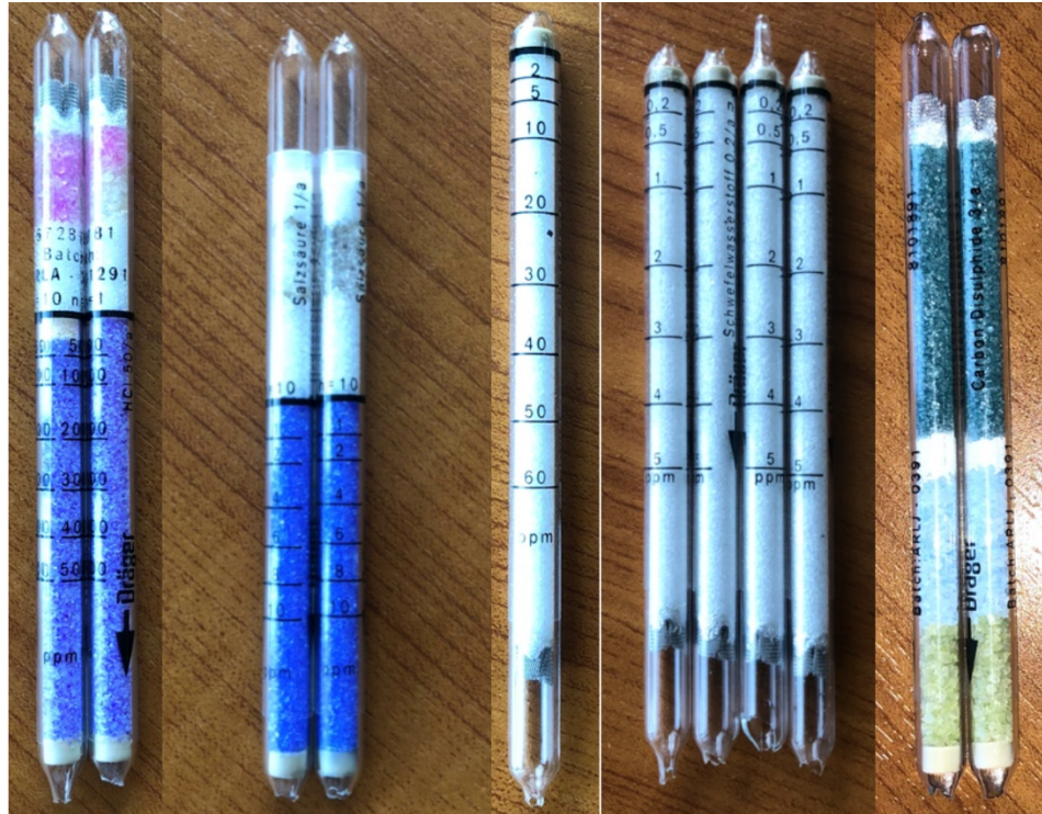
Figure 36 HCl and H 2 S Dräger tubes. From left to right: 2x HCl 500-5000 ppm, 2x HCl 1-10 ppm, 1x HCl 2-60 ppm, 4x H 2 S 0.2-5 ppm, 2x C 2 S 3-95 ppm.
