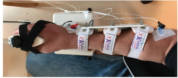
Figure 2 The experimental setup of the experiment. Participants were attached with Velcro to the forearm support and handle of a single axis wrist manipulator (Wristalyzer, MOOG FCS, Nieuw Vennep, the Netherlands), which applied multisine torque perturbations to the wrist. The resulting wrist torque and angle were measured, as well as the muscle activation of the FCR and ECR muscle.
