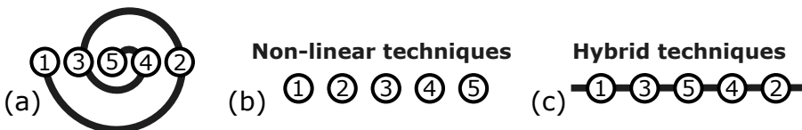
Figure 6.1: Dimensionality reduction with landmarks. In non-linear embedding techniques the underlying manifold (a) is respected (b). In hybrid approaches, landmarks are placed without considering the underlying manifold (c) and data points are placed by interpolating the landmark positions (grey line in c). The layout quality thus relates to the used number of landmarks.
