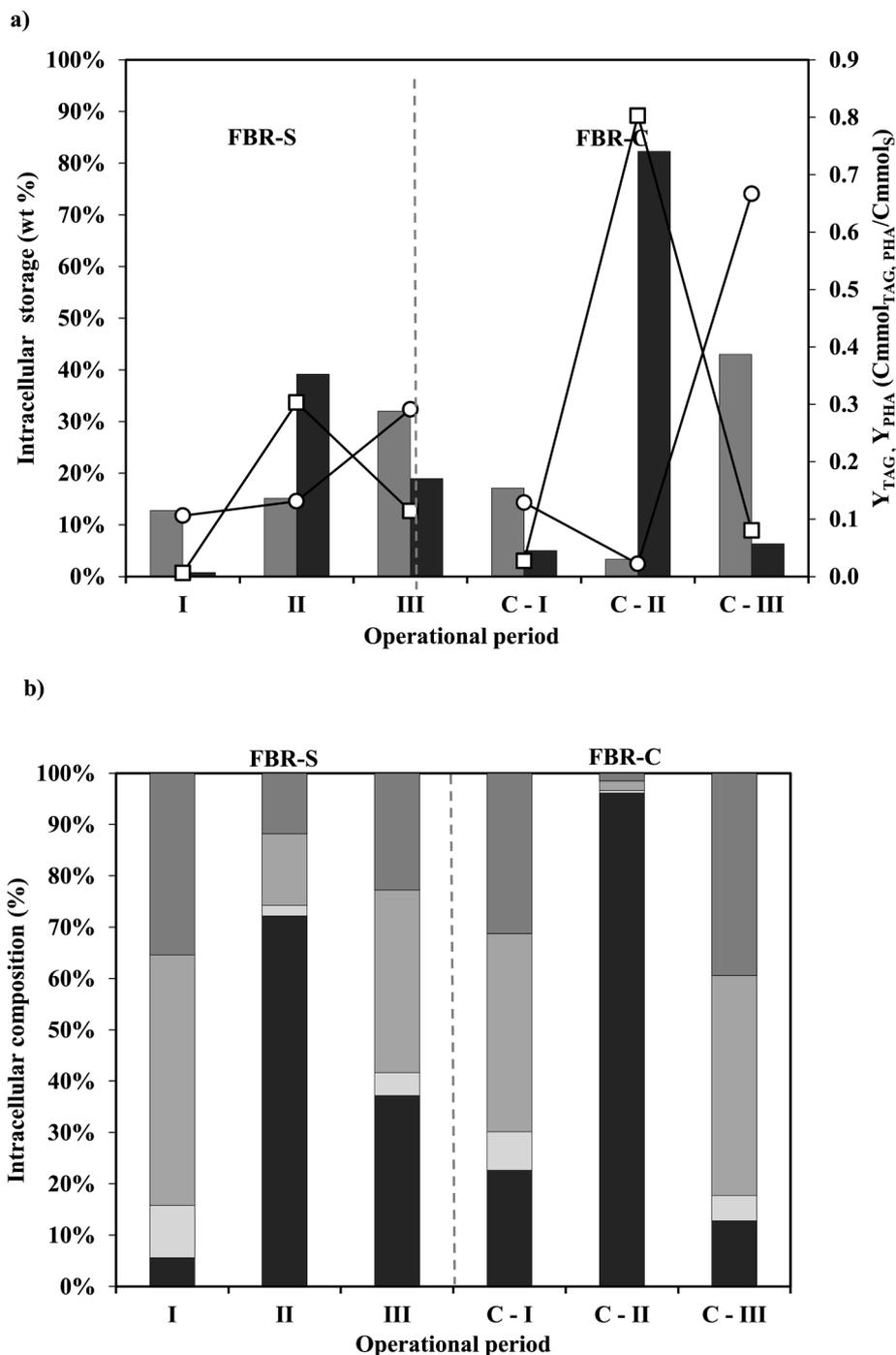
**Fig. 3.** Comparison between FBR-S and FBR-C considering analogous operational periods (I, II, III vs C-I, C-II, C-III). a) Maximum intracellular TAG (■) and PHA (■) storage and production yields ( $Y_{TAG}$  (○),  $Y_{PHA}$  (■)), b) Intracellular compounds composition (palmitic (□), oleic (▨), linoleic (▩), PHB (■)).
