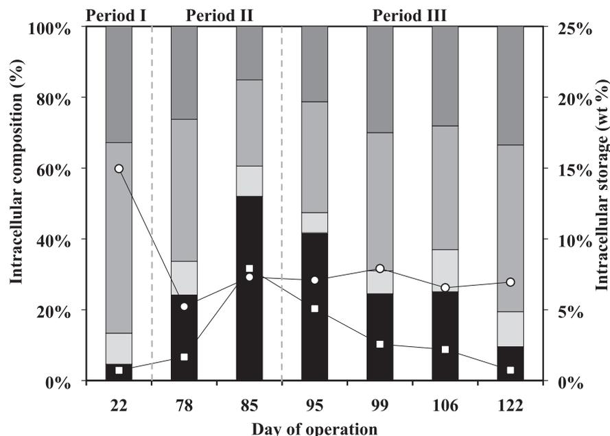
**Fig. 2.** Percentages of intracellular compounds accumulated (TAG (○) and PHA (■)), and composition (palmitic (□), oleic (▨), linoleic (▩), PHB (■)) measured at the end of the feast phase in different SBR-S cycles throughout periods I – III.
