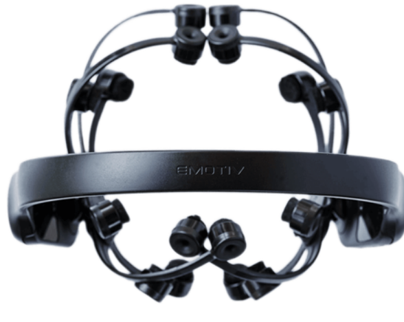
Figure 4.5: Emotiv Epoc X EEG headset (Emotiv, 2023b)
