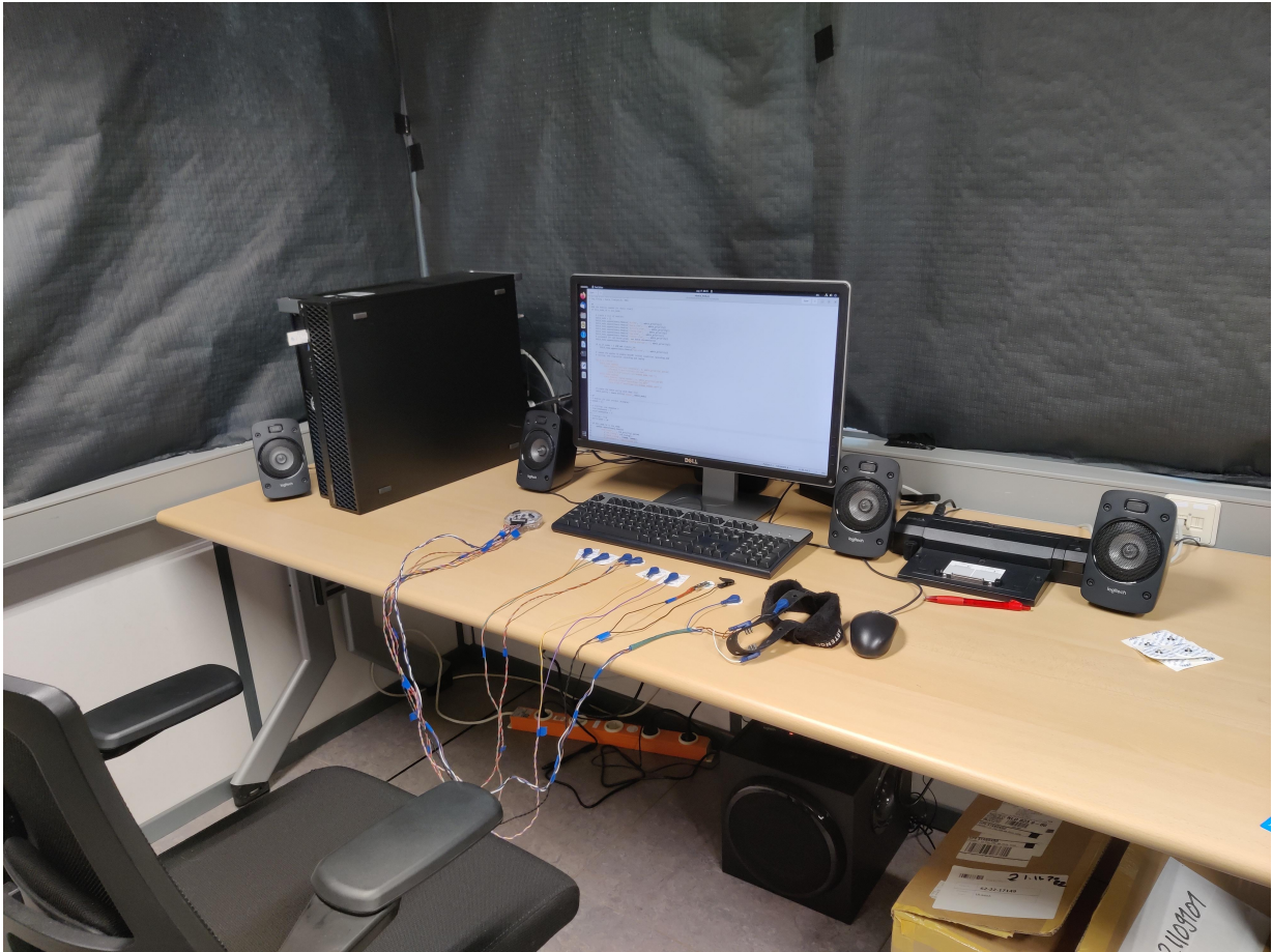
Figure G.1: Experiment set-up. Stimuli were presented on the computer display and via the stereo 5.0 system in a darkened room.
