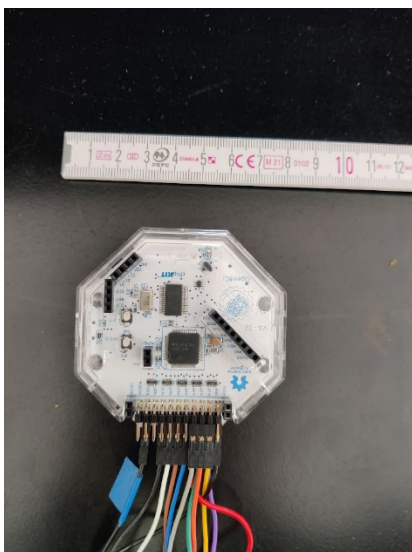
Figure 1: OpenBCI Cyton front view, in plastic casing with electrode wires attached
