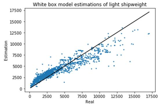
Figure 5.3: White box model results - General cargo ship
