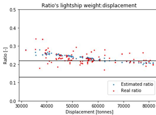
Figure 5.35: Oil tanker - Deadweight tonnage [25000, 120000]
