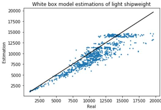
Figure 5.2: White box model results - Bulk carrier
