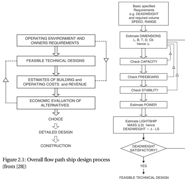
Figure 2.1: Overall flow path ship design process (from [28])
