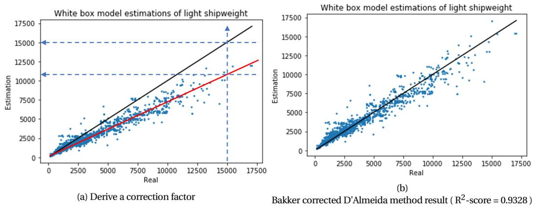
Figure 5.30: Correcting the D'Almeida method
