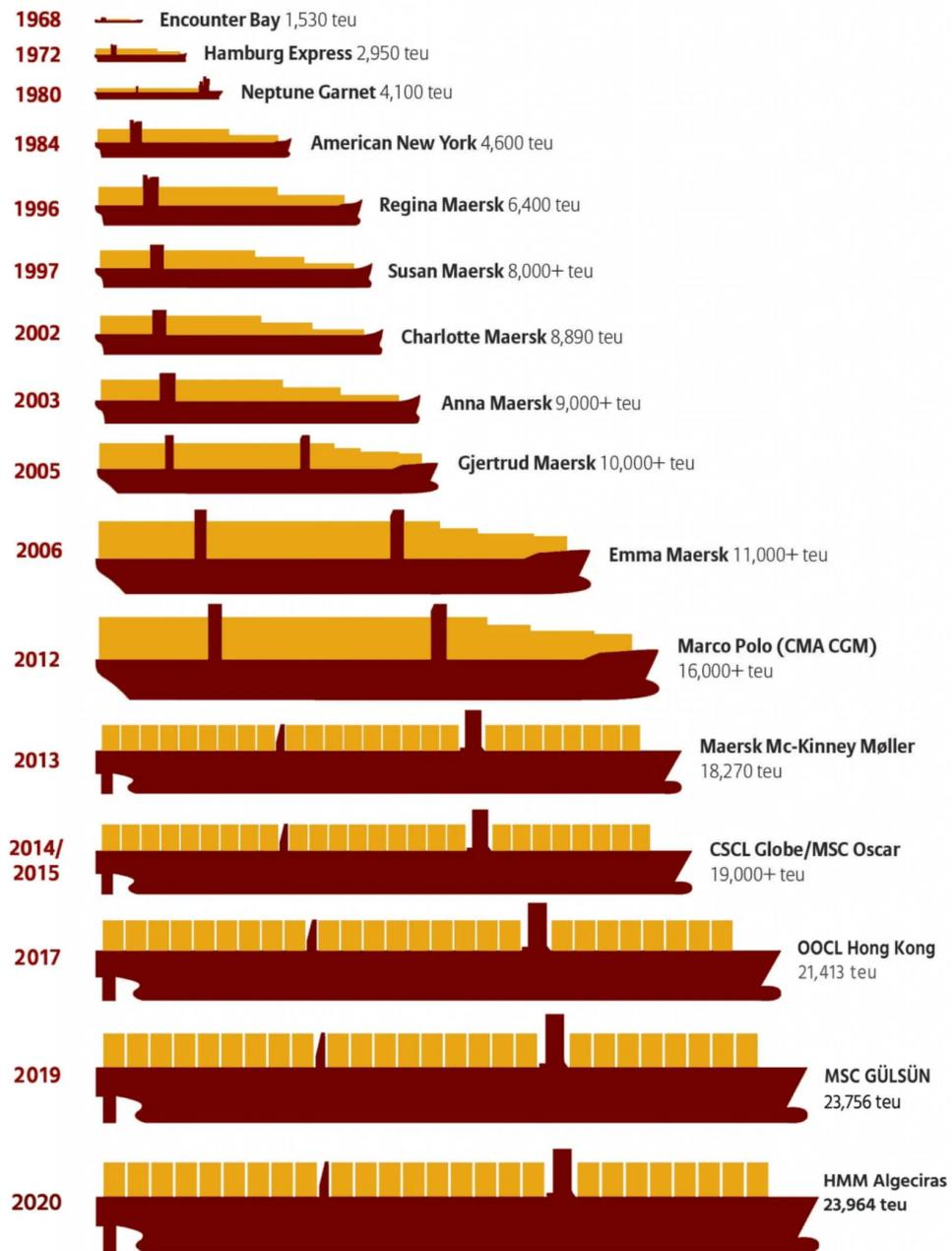
Figure 5.1: Development of container ship size (from Shipping and Freight Resource, 2021)
