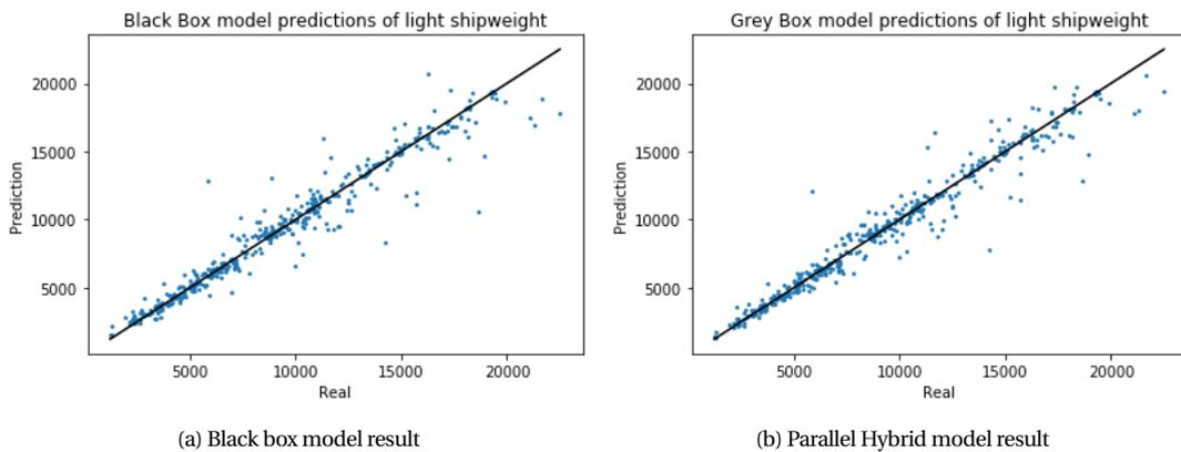
Figure 5.10: Lightship weight predictions - Container ship
