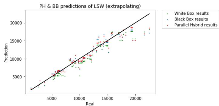
Figure 5.32: Predicting the lightship weight of future ships- Container
