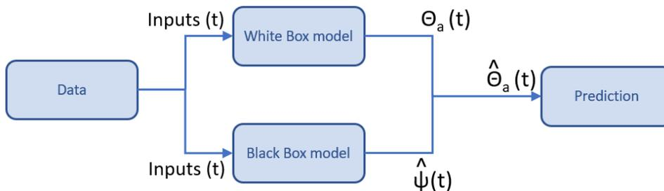
Figure 4.2: General description of a Parallel Hybrid model - Prediction phase
