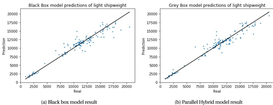
Figure 5.9: Lightship weight predictions - Oil tanker
