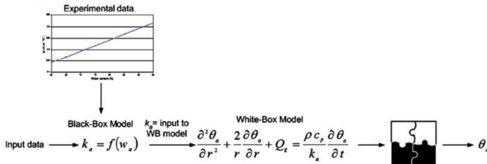
Figure 3.1: Serial hybrid modelling approach 1 (from [16])
