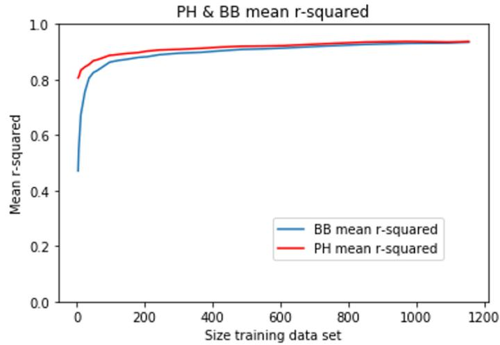
Figure 5.12: Increasing the  $N_{\text{Train}}$  of the bulk carrier
