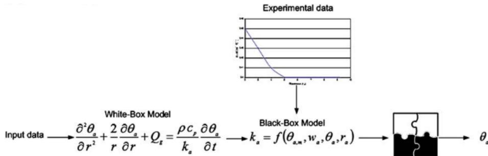
Figure 3.2: Serial hybrid modelling approach 2 (from [16])
