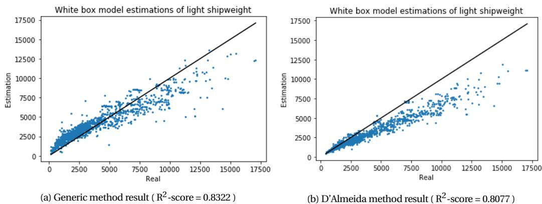
Figure 5.29: Deeper look into the white box model performance for the general cargo ship
