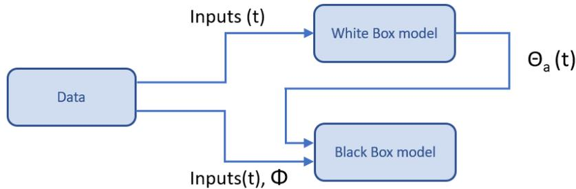
Figure 4.1: General description of a Parallel Hybrid model - Training phase
