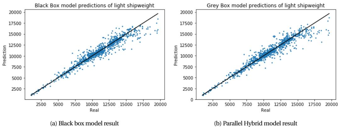
Figure 5.7: Lightship weight predictions - Bulk carrier
