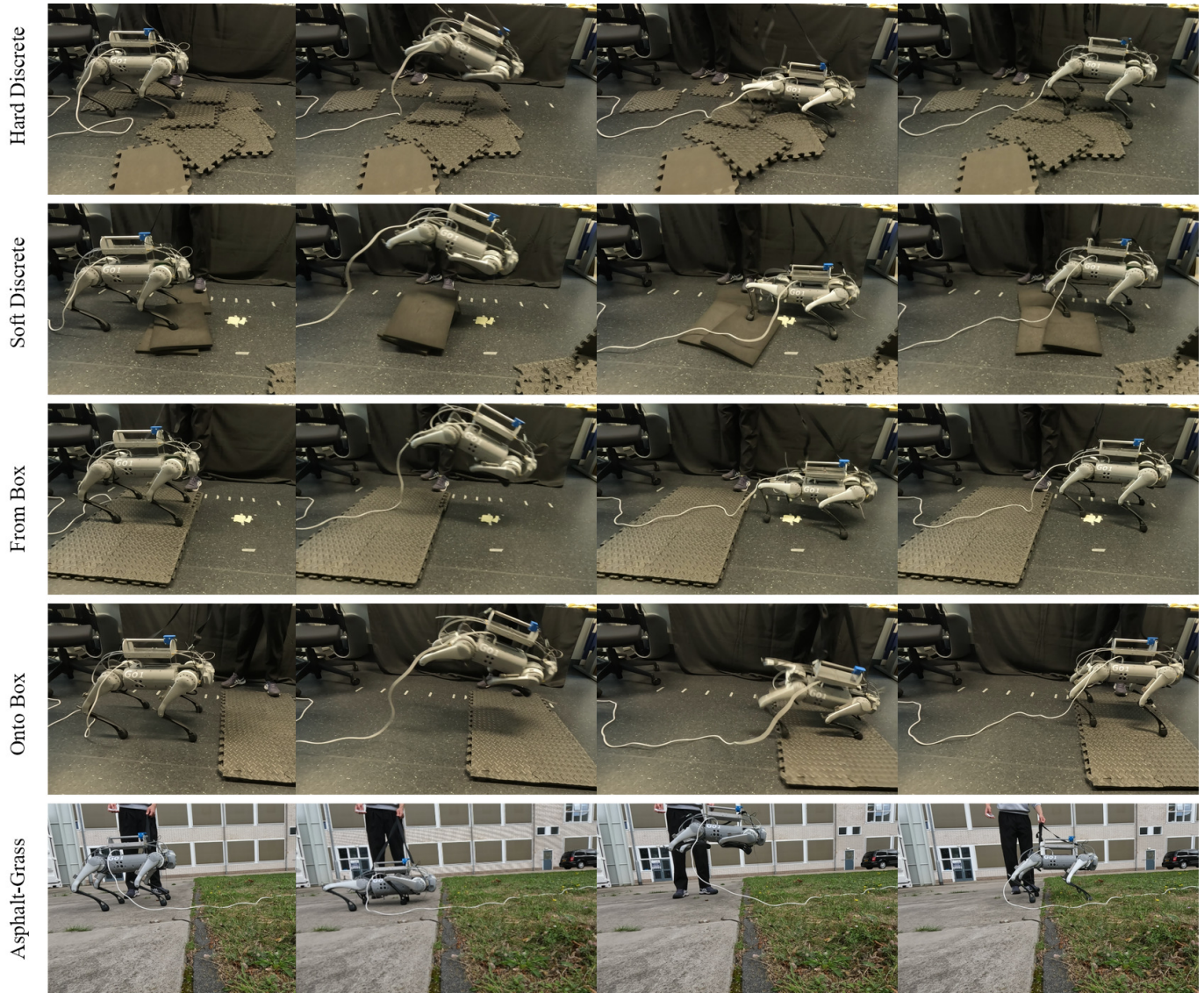
Fig. 17. Several experiments showcasing the robustness of the policy \pi_{II} to variations in the terrain: jumping across discrete hard and soft objects (rows 1 and 2), blindly jumping from and onto a small box (rows 3 and 4), and asphalt-to-grass jump (row 5).
