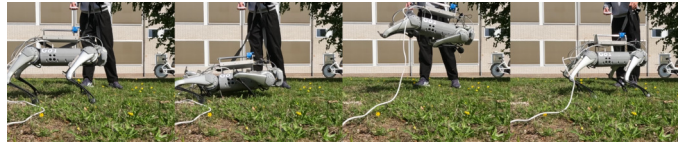
Fig. 1. The Go1 performing an outdoors 50cm long jump across soft grassy terrain under our proposed method.
