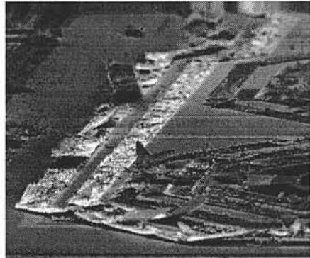
Figure 3. Peeling of the aluminium interconnect due to poor adhesion of the resist.
