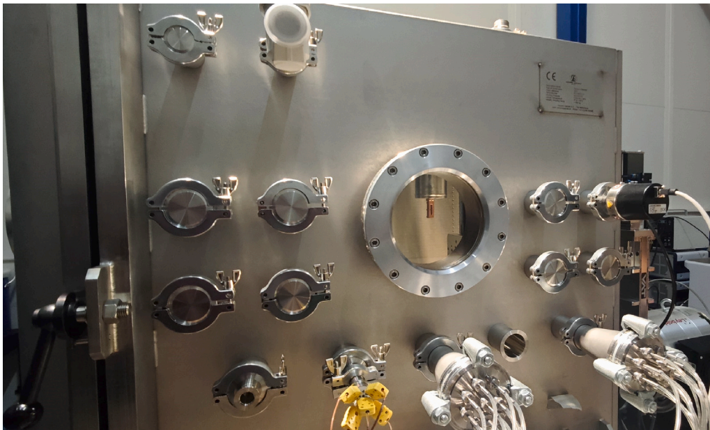
Fig. 3. Close-up view of the DN40 KF flanges for the feedthroughs on the side of the PISCES platform.
