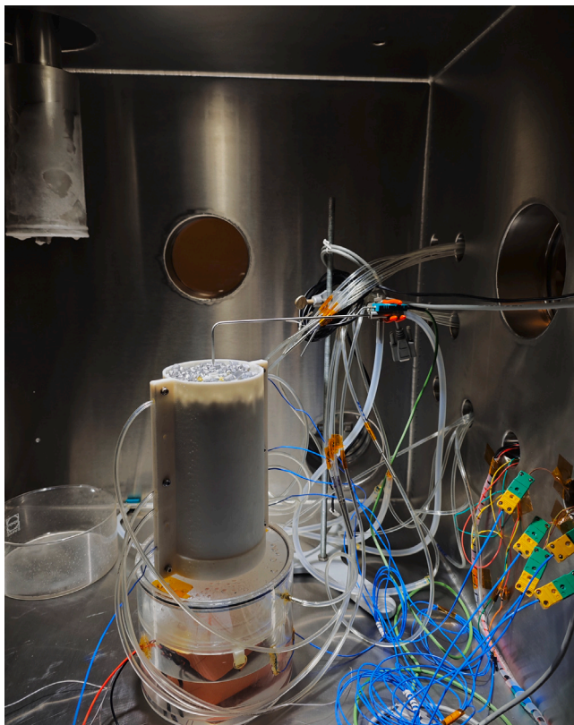
Fig. 6. Photo of a CLAM setup cooled with aluminium pellet to 215 K and hooked to PISCES.
