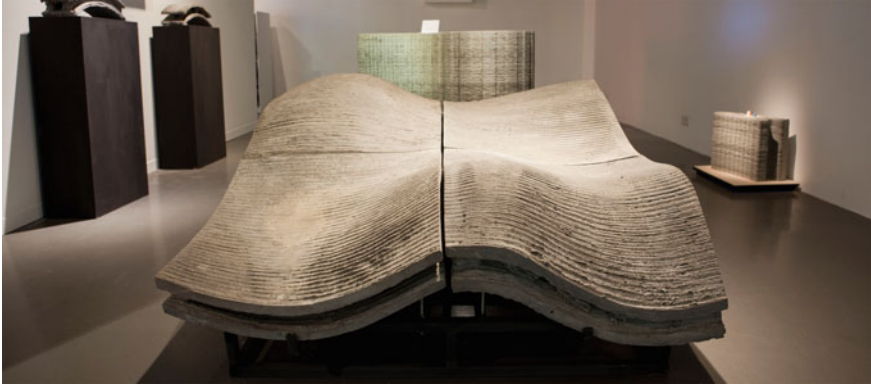
Fig. 2.7 Double-curved panels printed with conformal voids
