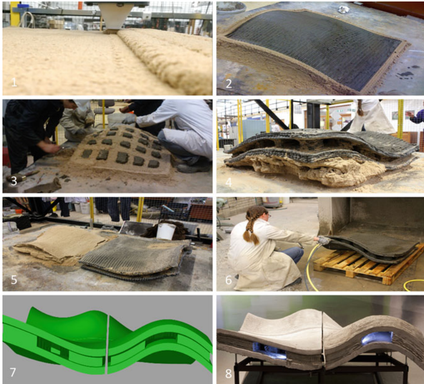
Fig. 2.10 Six stages of manufacturing one of the panels and the CAD model compared to the finished parts
