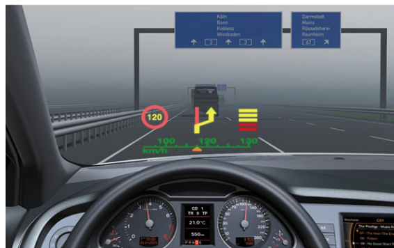
Figure 5.1.: An application of augmented reality; a head up display with laser projection in an unclassified Audi.
