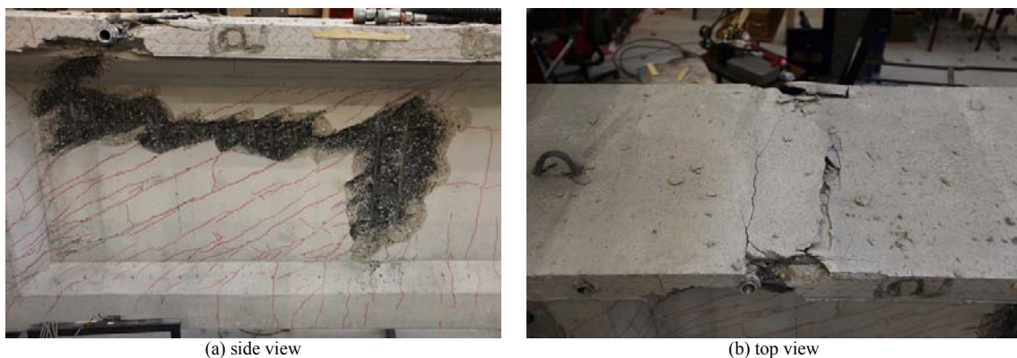
Fig. 15. Failure of beam 401 (first test)
