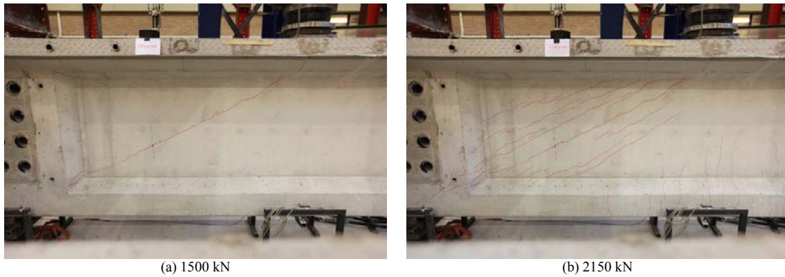
Fig. 13. Crack development beam 401 (first test) narrow flange side
