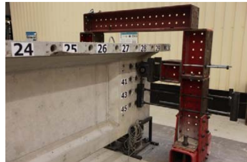
Fig. 7. Horizontal support at end of beam
