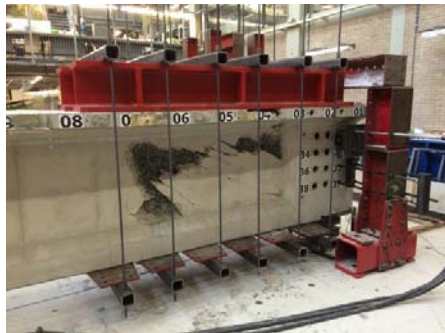
Fig. 6. Support frame with vertical prestressing
