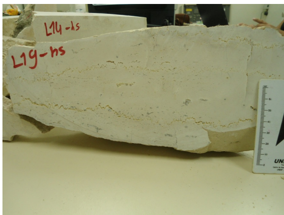
(a) Horizontal stylolites from sample L19 that were used for Fourier transform analysis.
