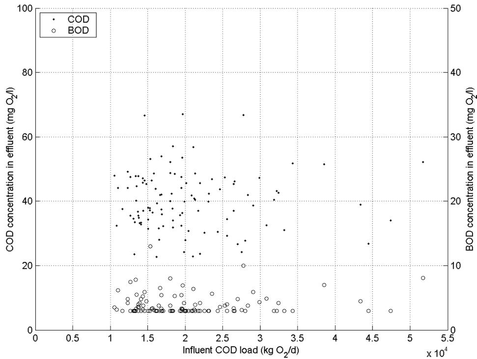
**Figure I.1** Wwtp Wervershoof. Influent COD load vs effluent COD and BOD concentration. Average dwf loading is 17,000 kg COD/d.
