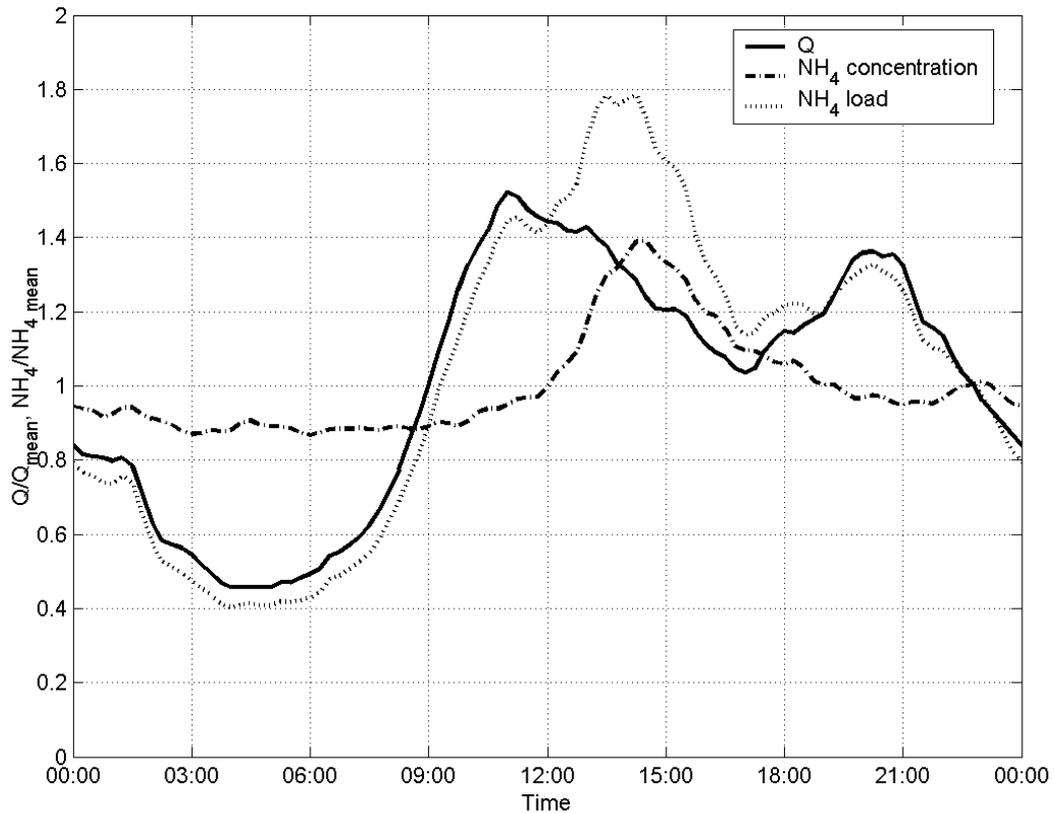
**Figure 6.4** Dwf profile for Katwoede: influent flow, ammonium concentration and ammonium load. The peak in ammonium load arrives almost 3 hours later than the peak in the influent flow due to the transport through the pressure mains.
