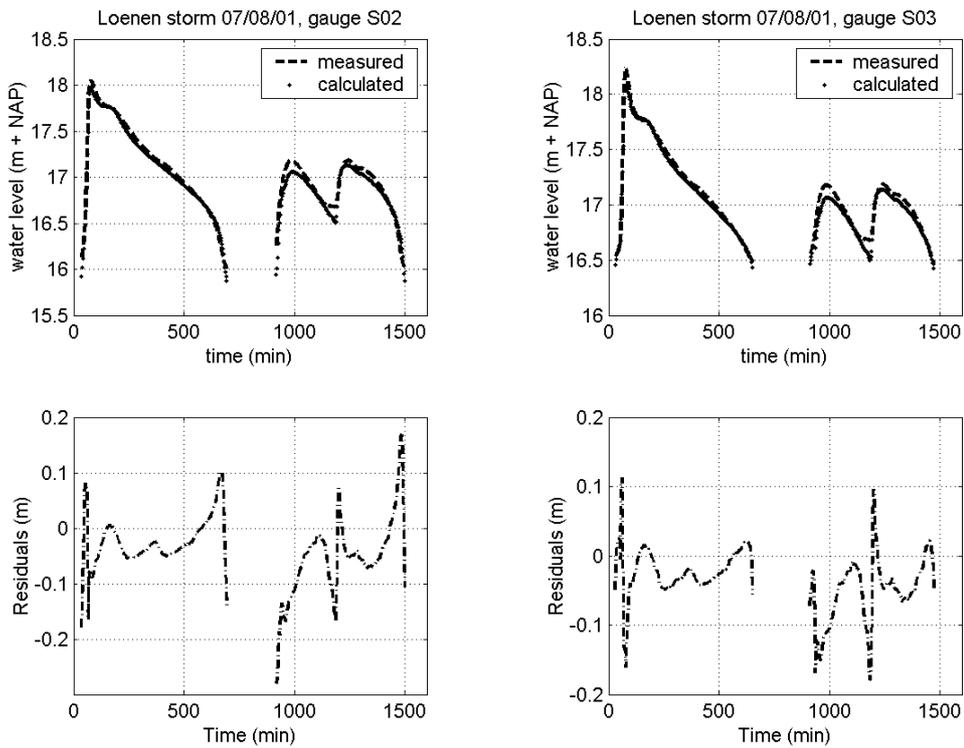
Figure X.16 Residuals storm 07/08/01, gauge S02 (left) and gauge S03 (right).
