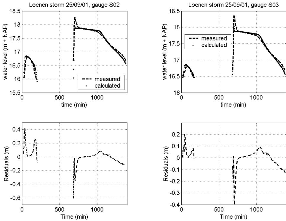
**Figure X.31** Residuals storm 25/09/01, gauge S02 (left) and gauge S03 (right).
