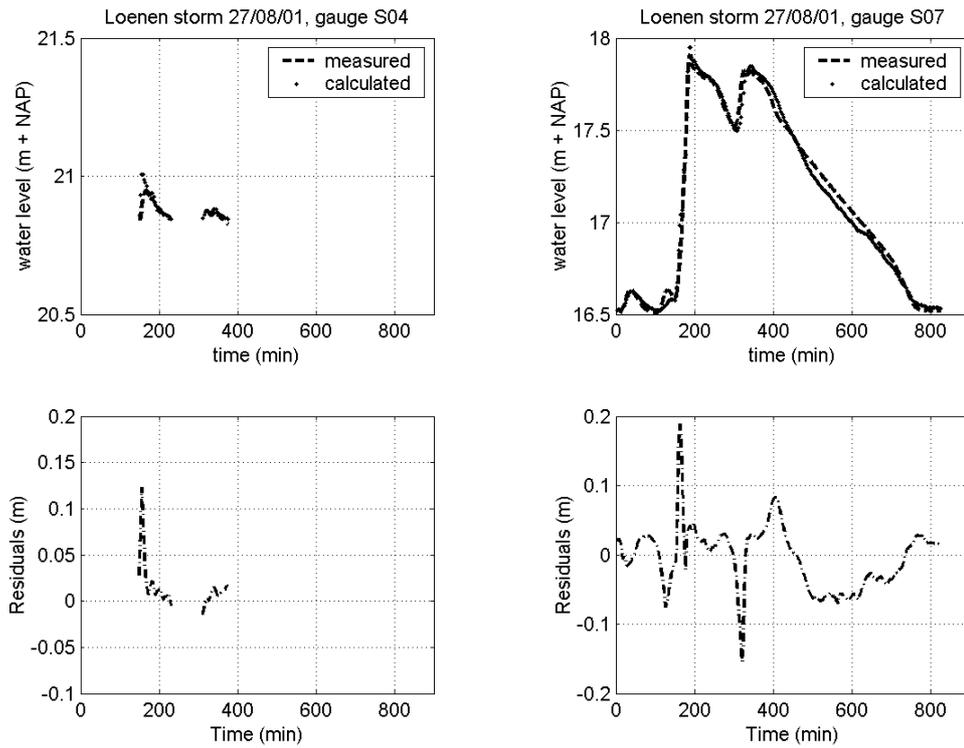
**Figure X.24** Residuals storm 27/08/01, gauge S04 (left) and gauge S07 (right).
