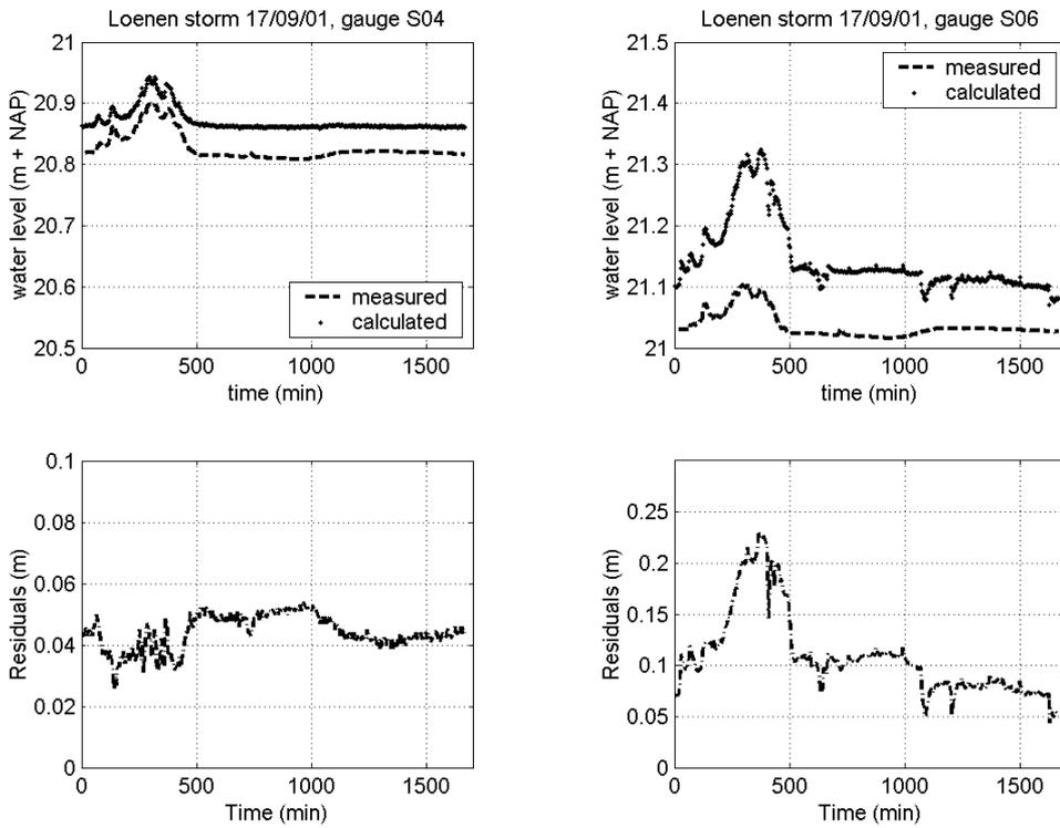
**Figure X.28** Residuals storm 17/09/01, gauge S04 (left) and gauge S06 (right).
