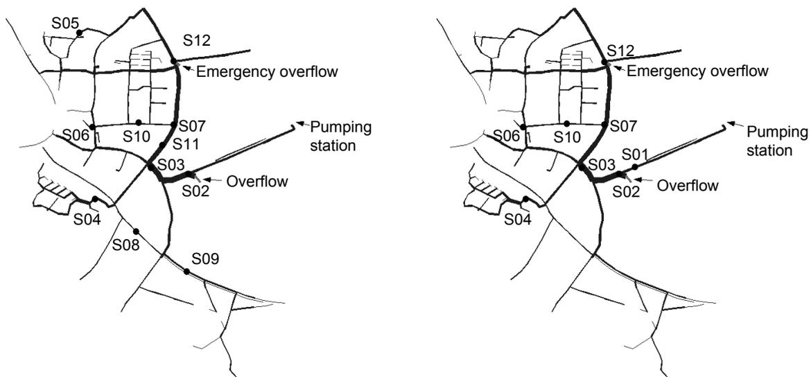
**Figure 4.34** Monitoring network Loenen (schematic). Left hand side: locations of water level gauges. Right hand side: locations of turbidity sensors.
