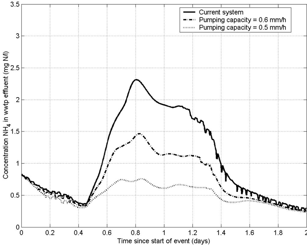
**Figure 6.21** Effect of decreasing the pumping capacity on ammonium concentration in wwtp effluent. Storm event B, ( $T = 0.1 \text{ y}^{-1}$ ).
