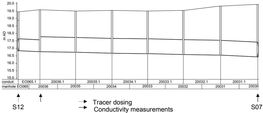
**Figure 4.17** Loenen, 233 m reach (distance between measuring locations),  $\varnothing$  1 m. The numbers of the gauges refer to figure 4.1.
