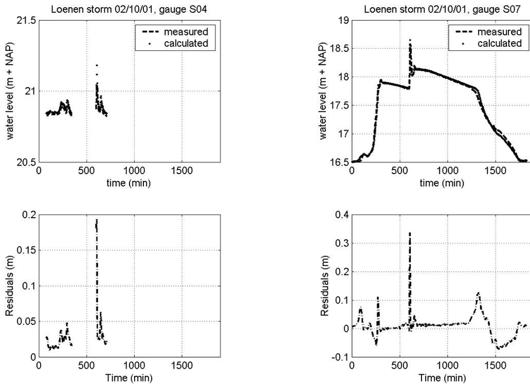
**Figure X.36** Residuals storm 02/10/01, gauge S04 (left) and gauge S07 (right)
