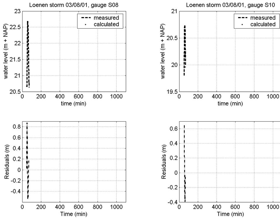
**Figure X.14** Residuals storm 03/08/01, gauge S08 (left) and gauge S10 (right).
