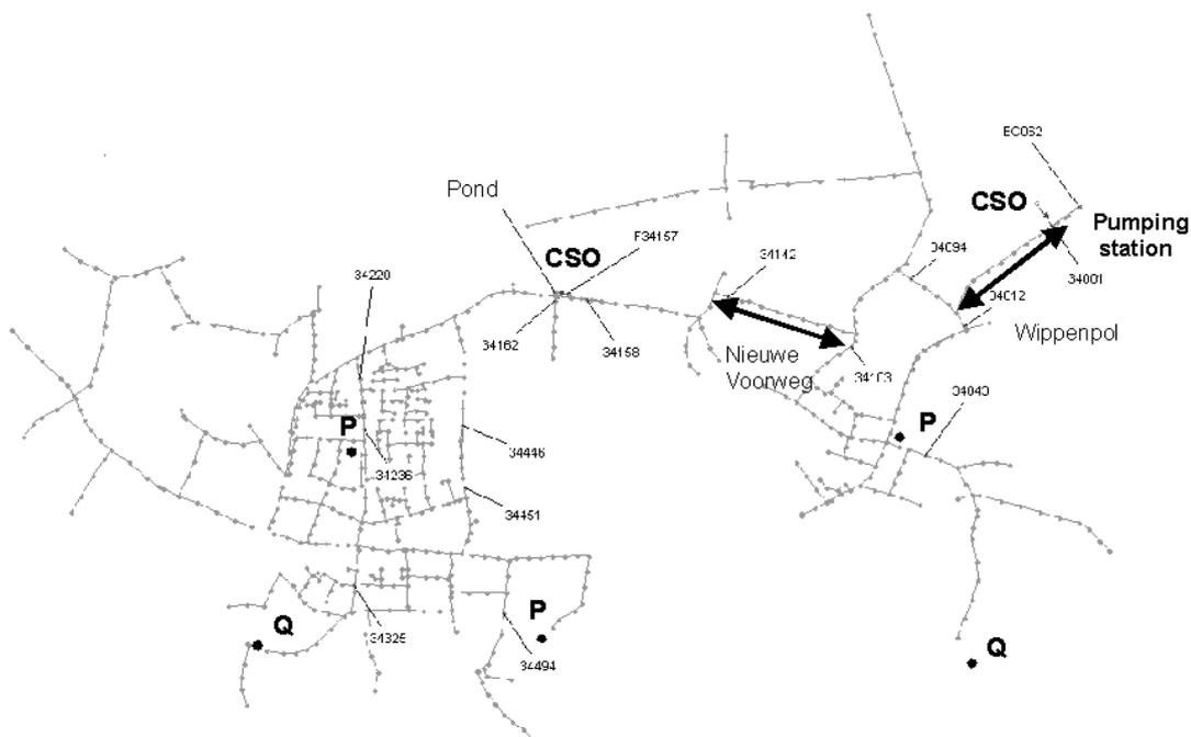
**Figure 4.19** Sewer system 'Beekbergen' (schematic). The indicated manholes have been equipped with a level sensor. The **Q** indicates measurement of the flow from an injecting pressure main, the **P** indicates measuring locations for precipitation. The arrows indicate the two reaches for the tracer experiments, Nieuwe Voorweg and Wippenpol.
