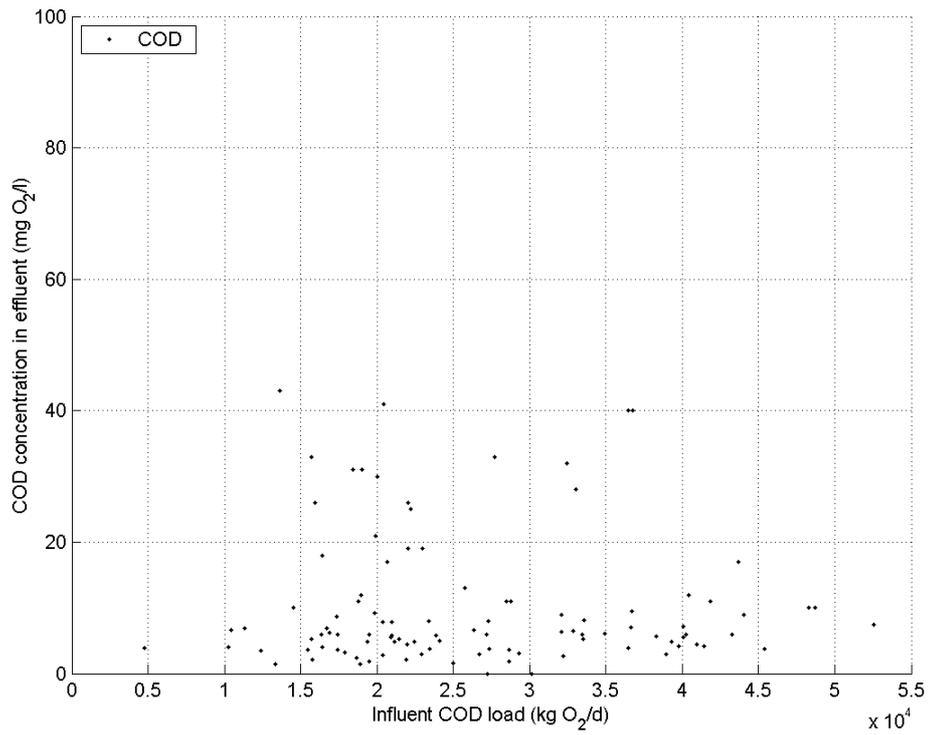
**Figure I.6** Wwtp Utrecht. Influent COD load vs effluent COD and BOD concentration. Average dwf loading is 21,000 kg COD/d.
