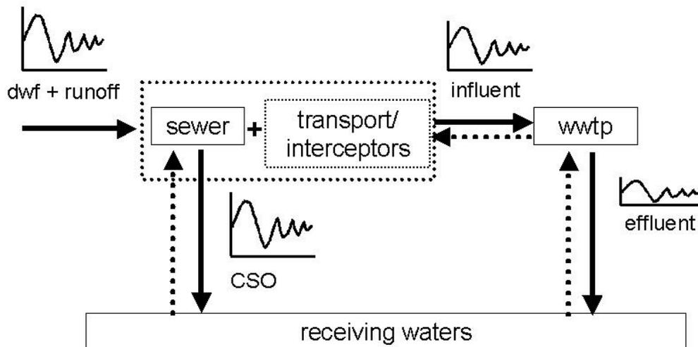
**Figure 1.1** Components of the urban wastewater system and their interactions. These interactions may be physical (a flow of water and its components) or non-physical (a flow of data or information) in both directions. (dwf = dry weather flow, CSO = combined sewer overflow, wwtp = wastewater treatment plant).
