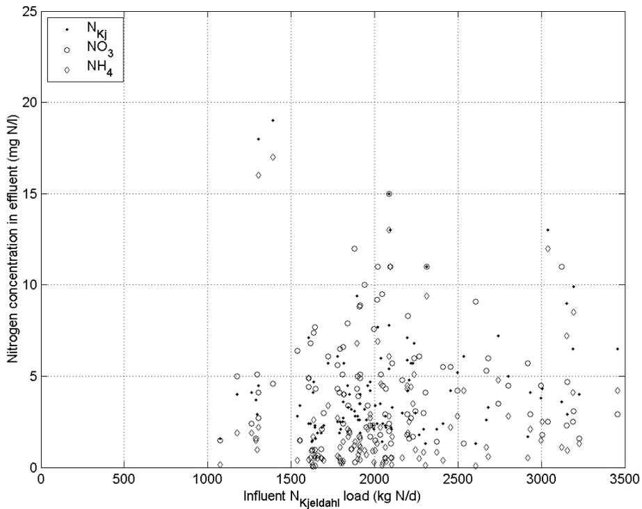
**Figure I.5** Wwtp Wervershoof. Influent nitrogen load flow vs effluent nitrogen concentration. Average dwf loading is 1,700 kg N/d.
