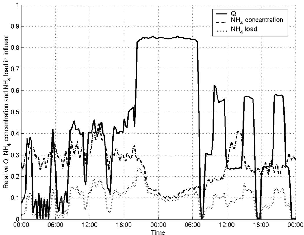
**Figure 6.5** Typical wwf profile for Katwoude: influent flow, ammonium concentration and ammonium load. The pressure mains cause a noticeable peak in the influent load of ammonium. The  $\text{NH}_4$  concentration is normalised by dividing by 100 mg N/l and the flow by dividing by the installed pumping capacity. The plotted  $\text{NH}_4$  load in the graph is the normalised flow times the normalised  $\text{NH}_4$  concentration.
