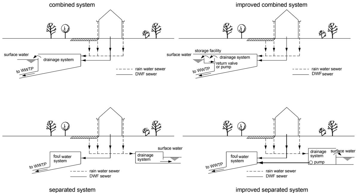
**Figure 1.3** Types of gravity sewer systems (reproduced with permission) [Clemens (2001a)].
