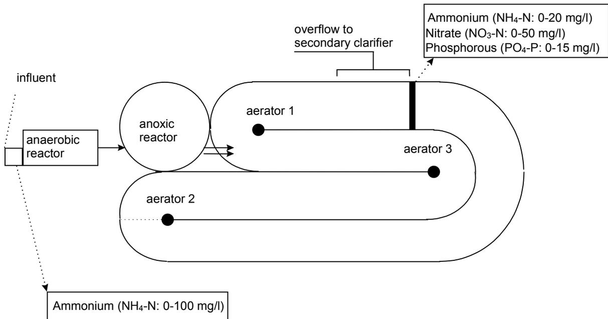
**Figure 3.4** Positioning of sensors at wwtp 'Katwoude'.
