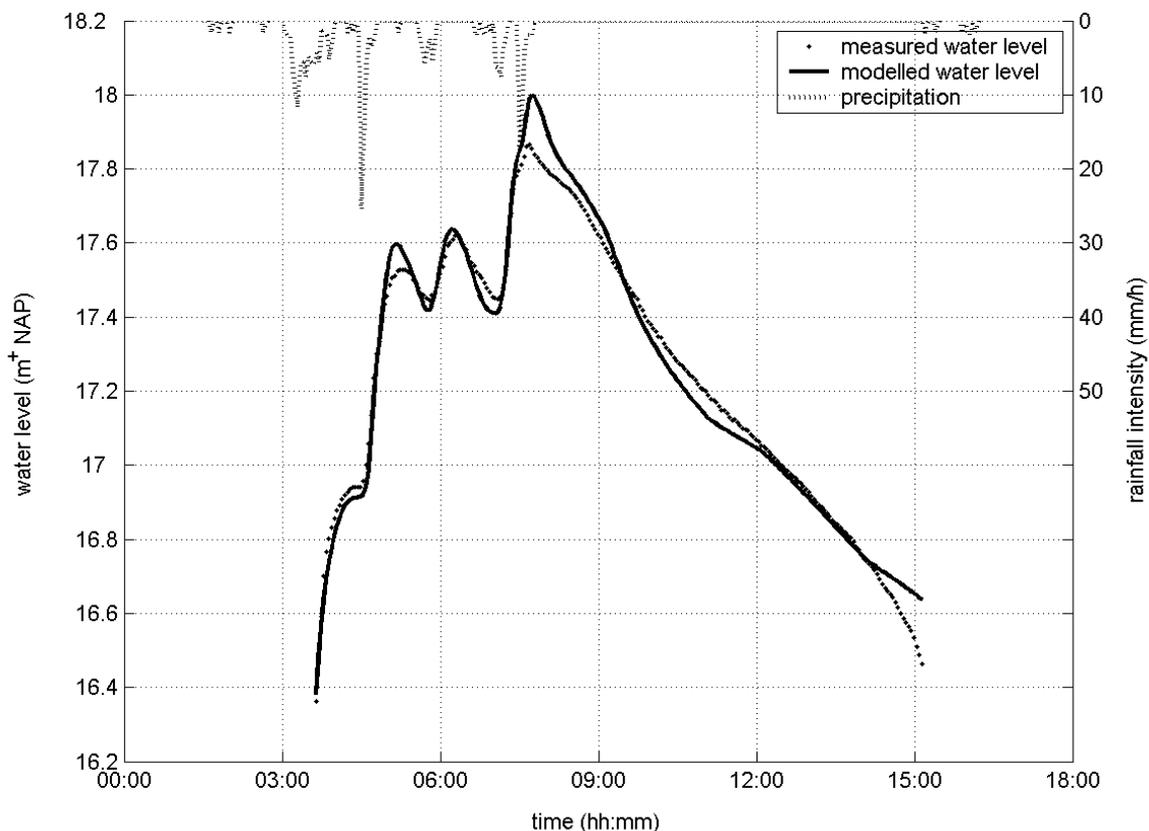
**Figure 4.2** Modelling results with incorrect crest level of overflow weir. Loenen, storm event 18 July 2001, location S02.
