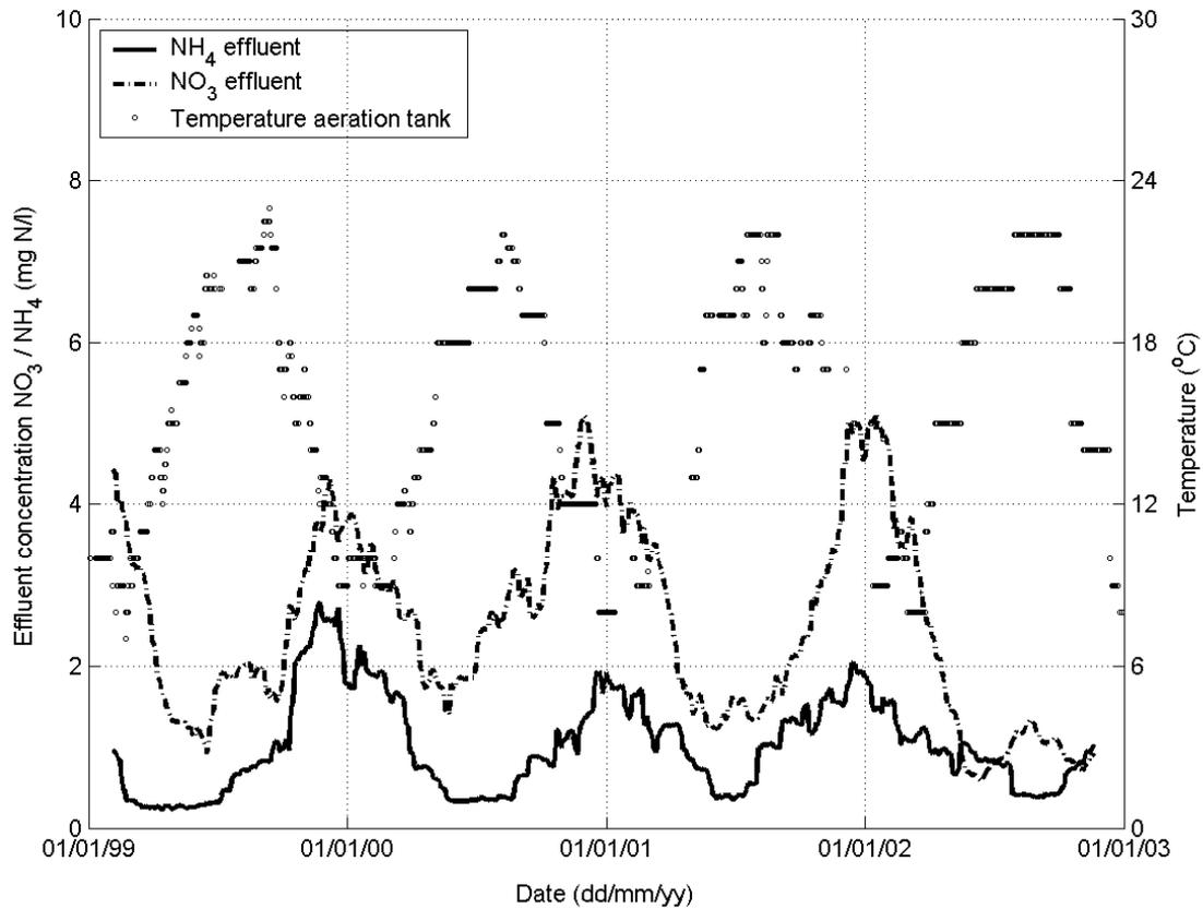
**Figure 3.9** Temperature of activated sludge and the moving average of the nitrate and ammonium concentration in the effluent of wwtp 'Katwoude' from 1999 to 2002.
