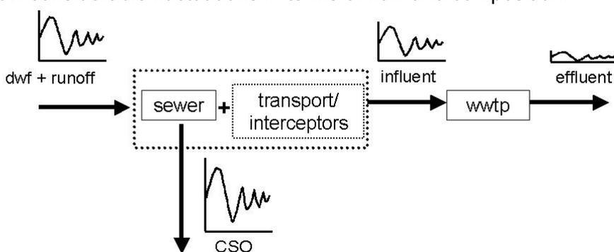
**Figure 2.2** Fluctuations of flows and substances through the wastewater system.
