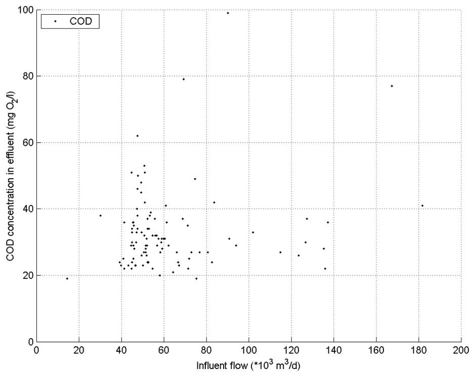
**Figure I.7** Wwtp Utrecht. Influent flow vs effluent COD and BOD concentration. Average dwf is 45,000 m<sup>3</sup>/d
