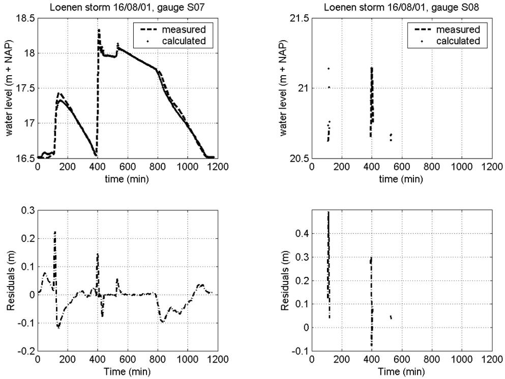
Figure X.21 Residuals storm 16/08/01, gauge S07 (left) and gauge S08 (right).
