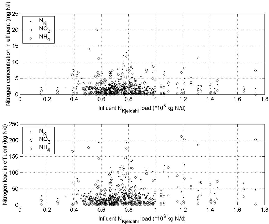
**Figure 3.7** Influent  $N_{\text{Kjeldahl}}$  load vs. effluent nitrogen concentrations (upper graph) and effluent nitrogen loads (lower graph). Concentrations are measured as 24 hour flow proportional composite samples. Like in figure 3.6, high nitrogen concentrations in the effluent do not seem to be related to a high influent load.
