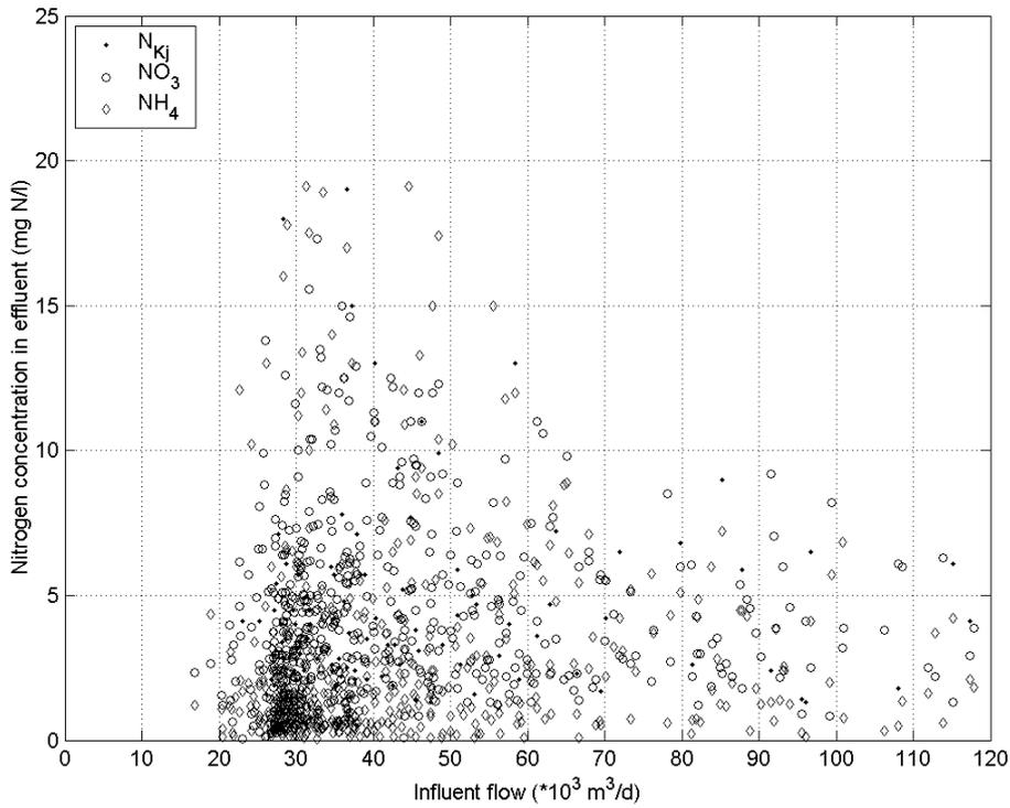
**Figure I.4** Wwtp Wervershoof. Influent flow vs effluent nitrogen concentration. Average dwf is 35,000 m<sup>3</sup>/d.
