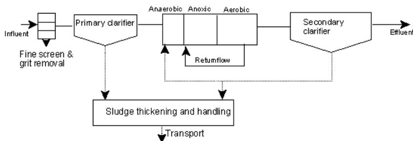
**Figure 2.10** General process scheme of a wwtp (after: [Nieuwenhuijzen, van (2002)]).
