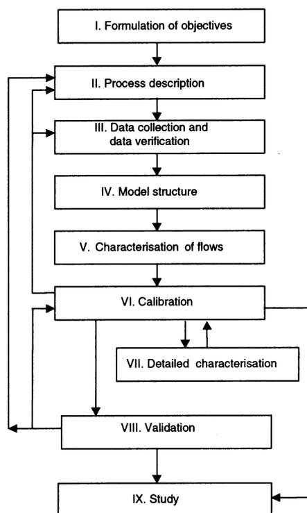
**Figure 3.16** Structure of SIMBA protocol (reproduced with permission from [Hulsbeek *et al.* (2002)]).
