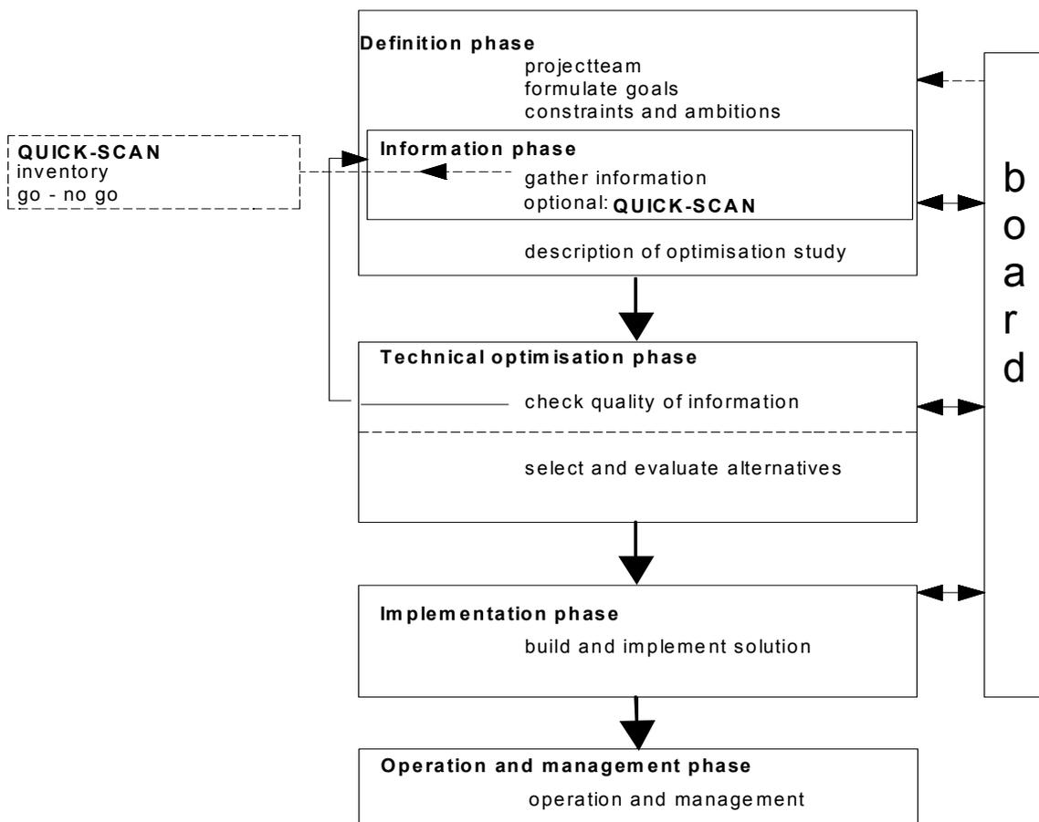
**Figure XI.1.** Process chart for wastewater system optimisation [Stichting RIONED (2003b)]. In this thesis the focus is on the technical optimisation phase. The board represents the local authorities, i.e. the water boards and municipalities.
