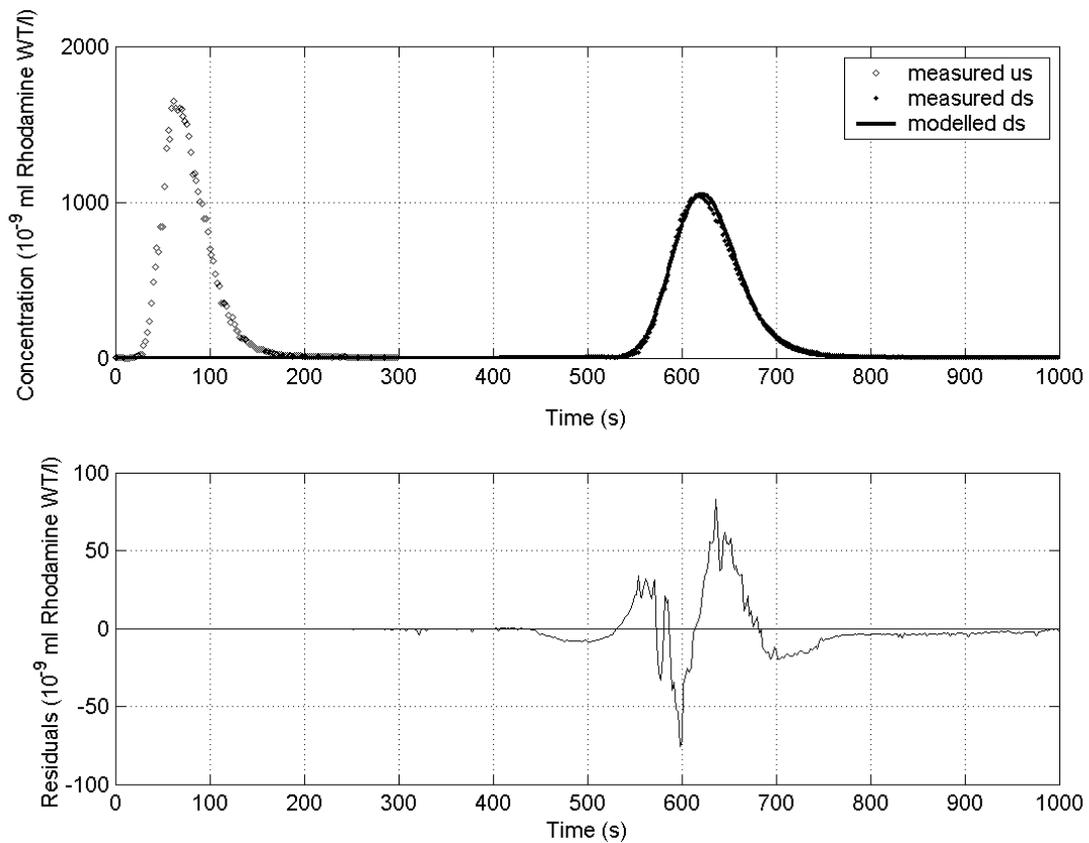
**Figure 4.29** Tracer experiment 1, 16/09/03. Beekbergen, reach Wippenpol, dispersion coefficient =  $0.13 \text{ m}^2/\text{s}$ .
