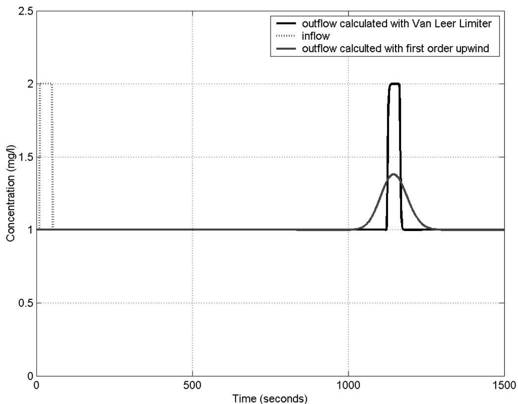
**Figure XIII.2** Example of calculation results using the Van Leer Limiter coded in Matlab, compared with a first order upwind scheme. A block shaped influent was simulated for a sewer reach of 454 m long with a flow velocity of 0.4 m/s.
