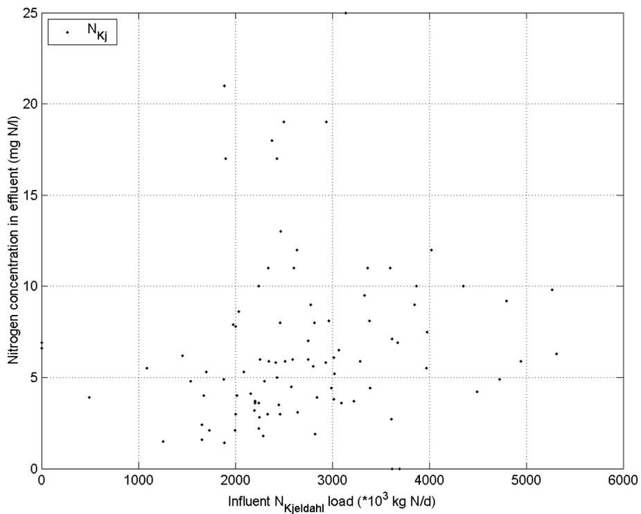
**Figure I.10** Wwtp Utrecht. Influent nitrogen load flow vs effluent nitrogen concentration. Average dwf loading is 2,000 kg N/d.
