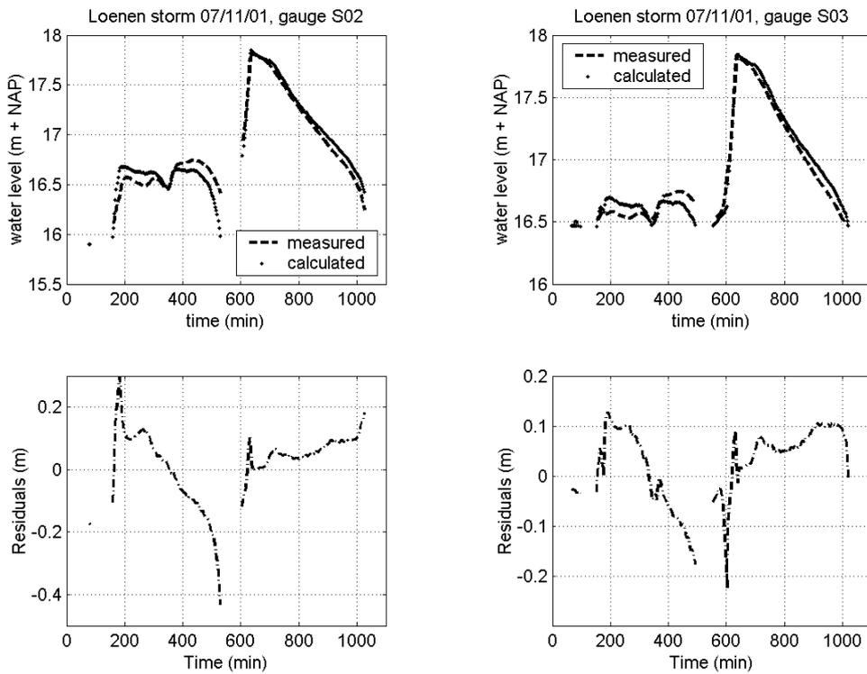
**Figure X.46** Residuals storm 07/11/01, gauge S02 (left) and gauge S03 (right).
