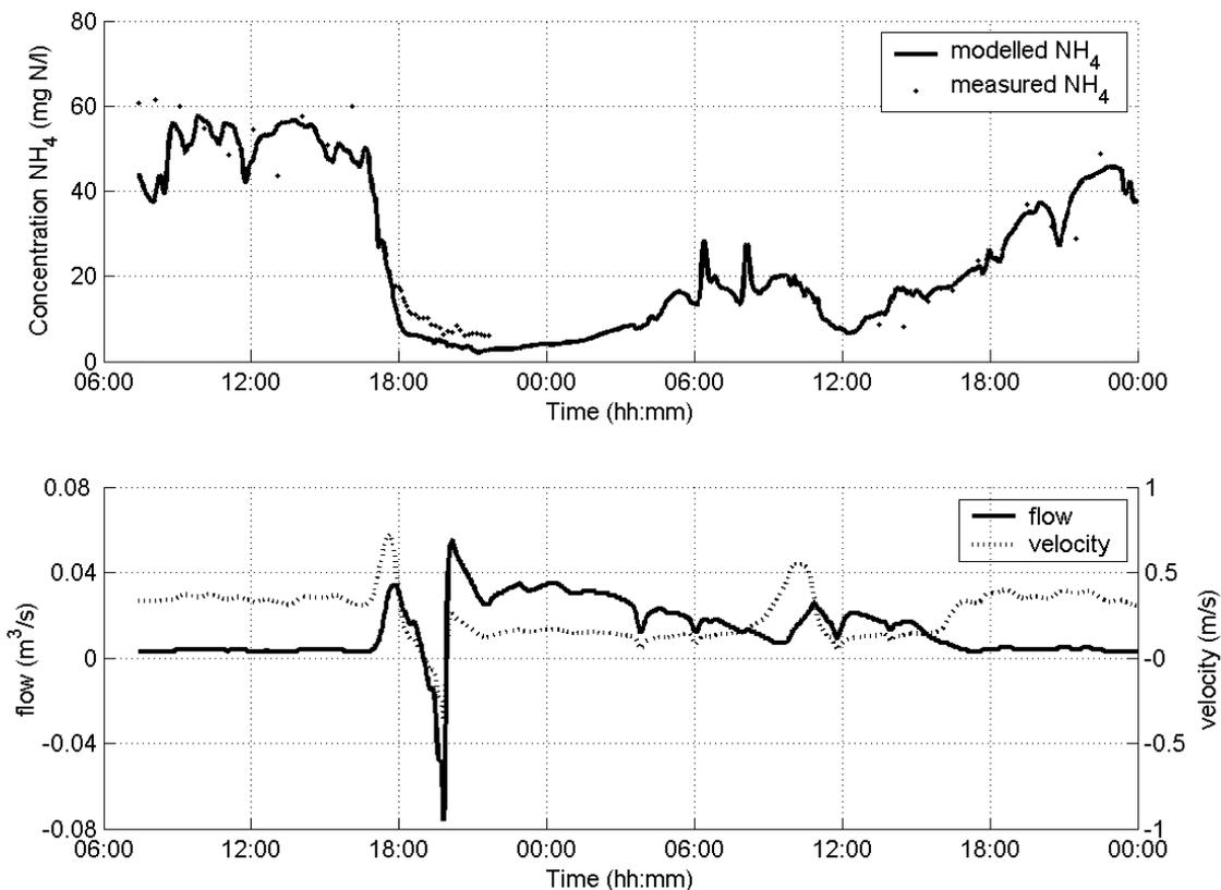
**Figure 4.32** Storm 01/04/03, Ulvenhout. Measured and modelled ammonium concentration (upper graph) and flow and velocity (lower graph). It is interesting to note that during the storm event the flow reversed towards the nearest CSO, see figure 4.24. The measured and calculated water levels for this storm event are given in figure 4.25.
