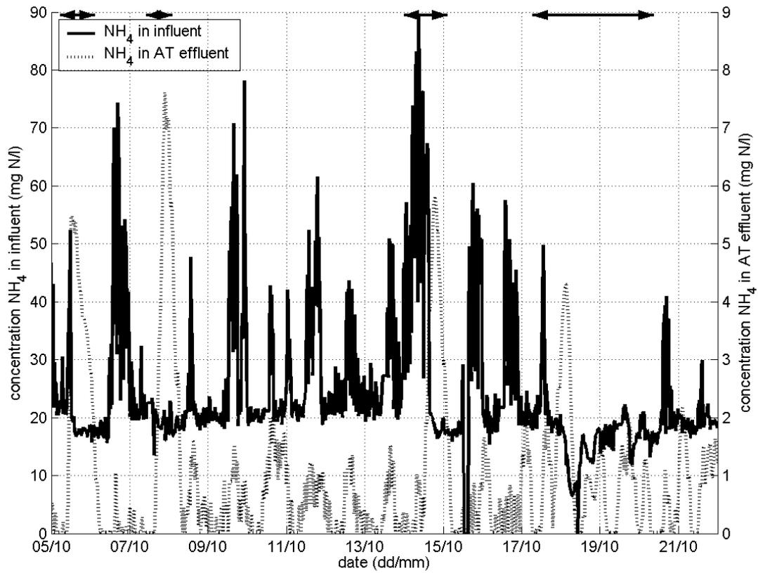
**Figure 3.11** Ammonium concentration in the influent and ammonium concentration (mg N/l) in the effluent of the aeration tank (AT). The arrows indicate storm events. The impact of the storm events on the ammonium concentration in the AT effluent (5, 7, 14 and 18 October) is clearly visible. Especially the higher peaks in ammonium concentration of the AT effluent do not seem to correlate with peaks in the ammonium concentration of the influent.
