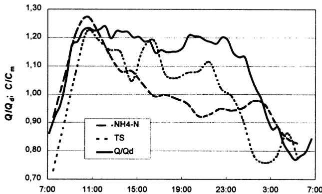
**Figure 2.4** Diurnal variations of flow rate, ammonia and TSS concentration normalised with daily averages. Measured at inlet wwtp Dresden, 500.000 p.e. [reproduced with permission from: Krebs *et al.* (1999)].  $Q$  = flow,  $Q_d$  = mean dwf,  $C$  = concentration,  $C_m$  = mean concentration
