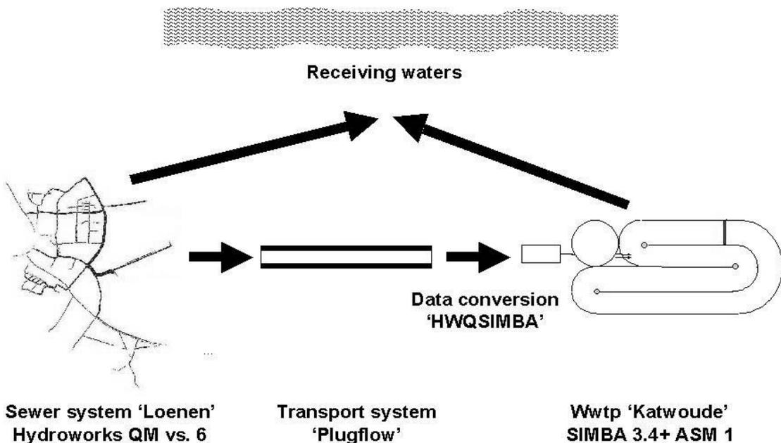
**Figure 6.7** Semi-hypothetical urban water system. The program HWQSIMBA was developed together with Marcel Boomgaard and the program plugflow was developed during the research project.
