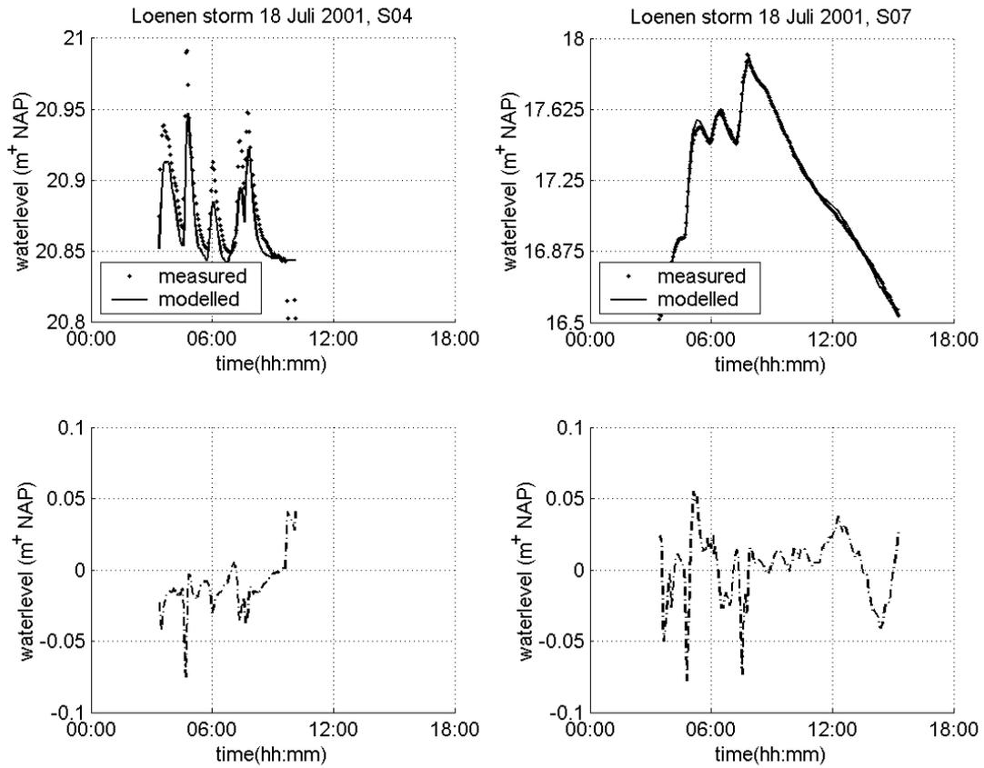
**Figure 4.5** Measured and modelled water levels during the storm of 18/07/01 in Loenen. The numbers of the measuring locations refer to the sites shown in figure 4.1.
