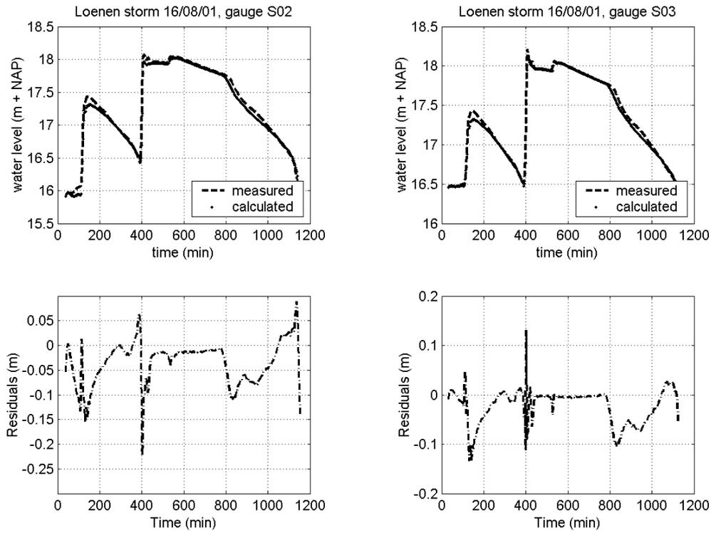
**Figure X.19** Residuals storm 16/08/01, gauge S02 (left) and gauge S03 (right).
