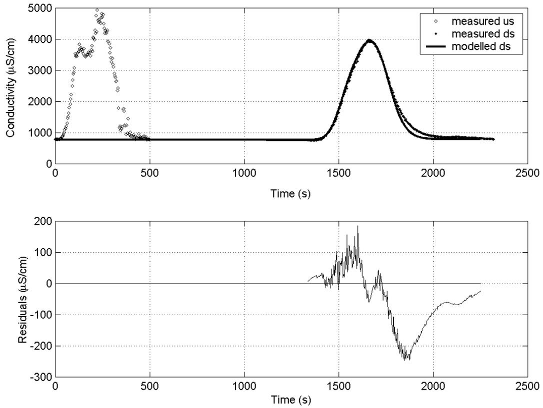
**Figure 4.28** Tracer experiment 4, 14/12/01. Loenen, 233 m sewer reach, dispersion coefficient =  $0.04 \text{ m}^2/\text{s}$ .
