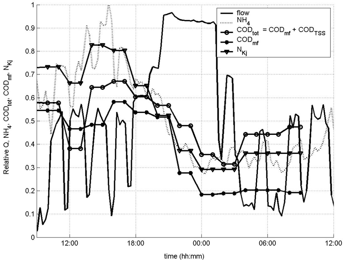
**Figure 3.18** Measured profiles of COD and N fractions. Influent measurements wwtp Katwoude, 1 and 2 December 2002. The concentrations are normalised:  $\text{NH}_4$  divided by 70 mg N/l,  $\text{N}_{\text{Kj}}$  divided by 90 mg N/l,  $\text{COD}_{\text{tot}}$  divided by 1000 mg  $\text{O}_2$ /l,  $\text{COD}_{\text{mf}}$  divided by 400 mg  $\text{O}_2$ /l. The flow is normalised by the maximum pumping capacity.
