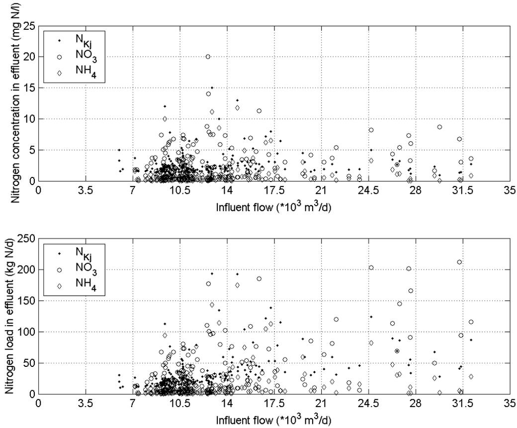
**Figure 3.5** Influent flow vs. effluent nitrogen concentrations (upper graph) and effluent nitrogen loads (lower graph). None of the nitrogen concentrations is clearly affected by the influent flow, although a large range is observed. Concentrations are measured as 24 hour flow proportional composite samples.
