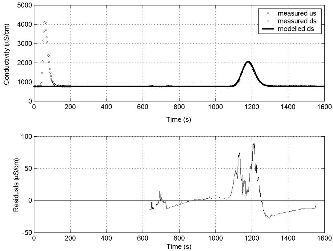
**Figure 4.27** Tracer experiment 1, 14/12/01. Loenen, 454 m sewer reach, dispersion coefficient =  $0.15 \text{ m}^2/\text{s}$ .
