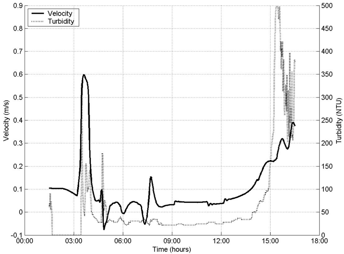
**Figure 4.38** Turbidity and flow velocity. The flow direction reversed two times: at 04:30 and 07:30 hour. Loenen, storm 18 July 2001, location S07.
