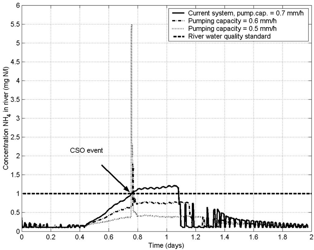
**Figure XII.2** Effect of pumping capacity on ammonium concentration in the river. Storm event B, T = 10°C.
