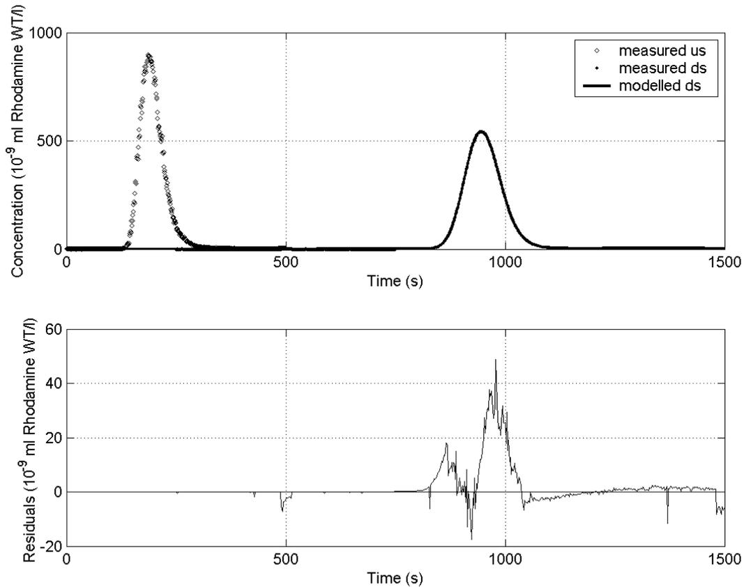
**Figure 4.30** Tracer experiment 5, Beekbergen, 16/09/03. Reach Nieuwe Voorweg, dispersion coefficient =  $0.145 \text{ m}^2/\text{s}$ .
