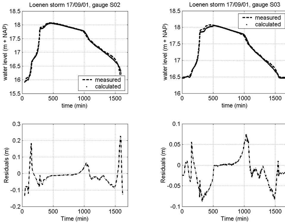
**Figure X.27** Residuals storm 17/09/01, gauge S02 (left) and gauge S03 (right).
