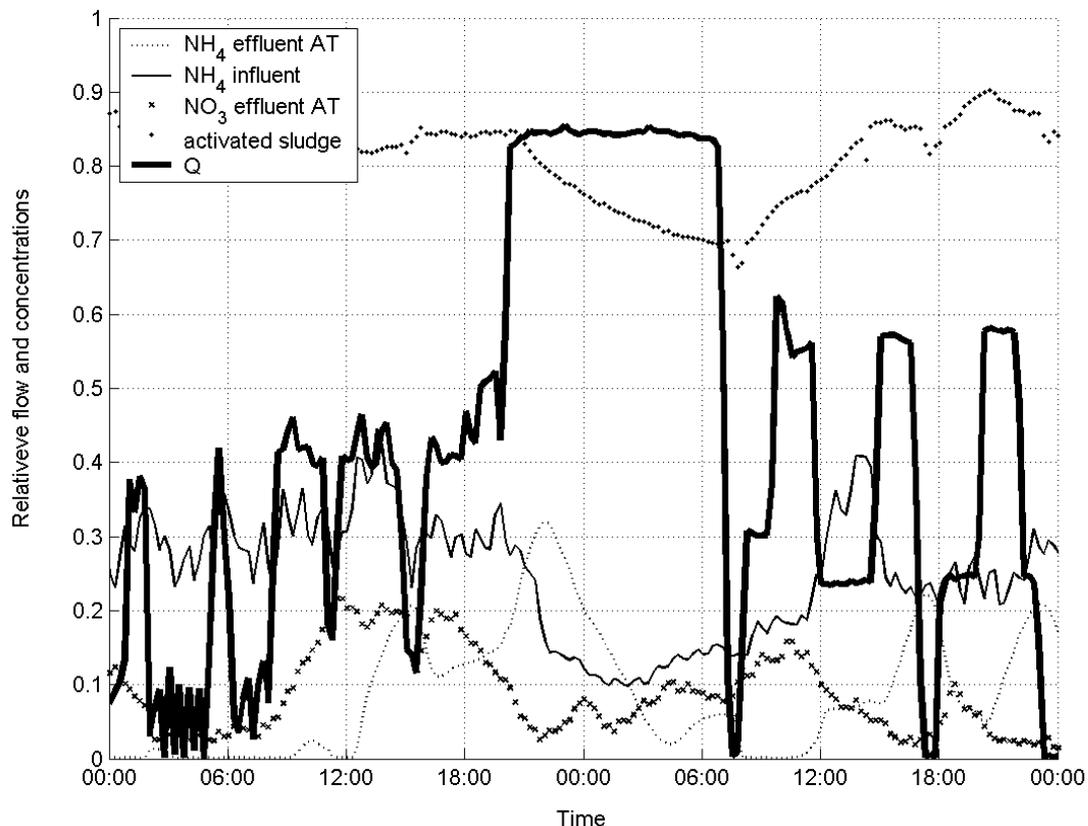
**Figure 3.10** Measurements at wwtp 'Katwoude'. Storm event 25-26 November 2002 (9.7 mm). The flow is plotted relative to the maximum pumping capacity. The concentrations are normalised as follows:  $\text{NH}_4$  effluent AT divided by 10 mg N/l,  $\text{NH}_4$  influent divided by 100 mg N/l,  $\text{NO}_3$  effluent AT divided by 10 mg N/l and activated sludge concentration divided by 5 g MLSS/l.
