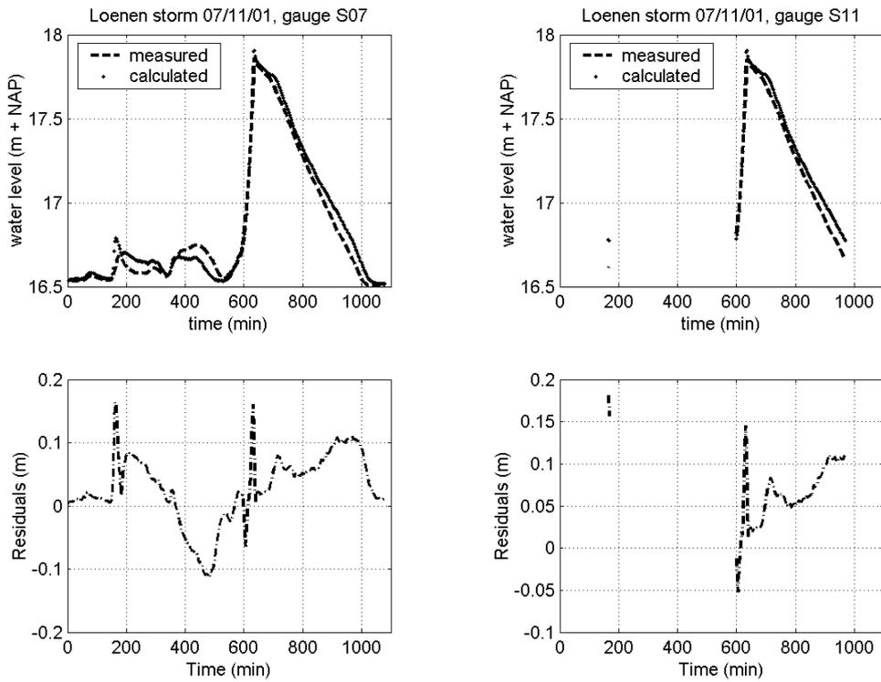
**Figure X.48** Residuals storm 07/11/01, gauge S07 (left) and gauge S11 (right).
