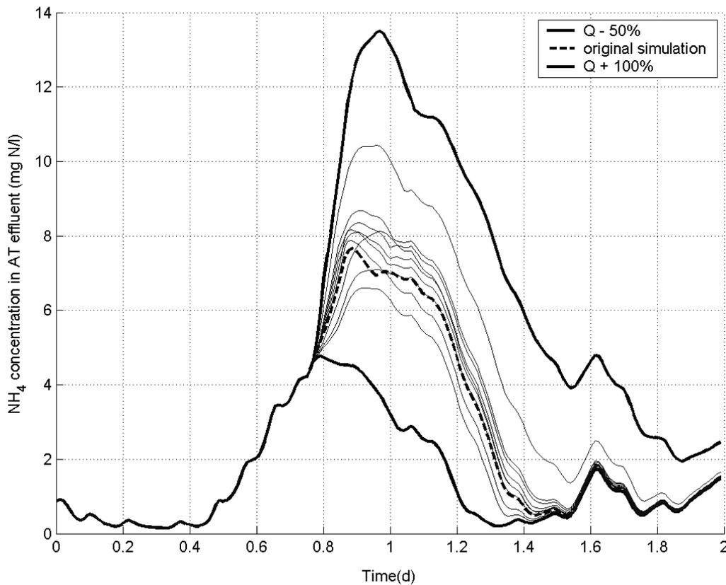
**Figure 3.28** Effect of systematic errors in influent flow during the dilution phase of the storm event (time from 0.77 to 1.03) on ammonium concentration in the AT effluent. The thick lines represent the outer ranges (-50% and + 100% respectively), the thin lines represent simulation results for systematic errors within this interval.
