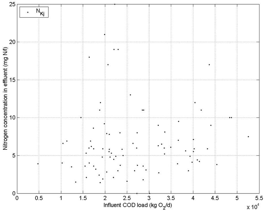
**Figure I.8** Wwtp Utrecht. Influent COD load vs effluent nitrogen concentrations. Average dwf loading is 21,000 kg COD/d.
