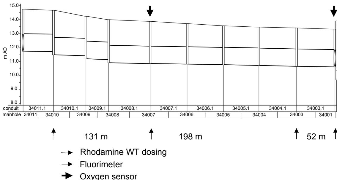
**Figure 4.43** Measuring locations sewer system Beekbergen, reach 'Wippenpol'.
