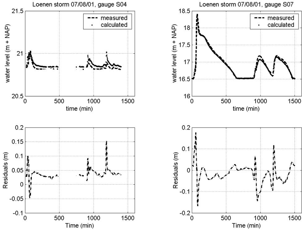
Figure X.17 Residuals storm 07/08/01, gauge S04 (left) and gauge S07 (right).
