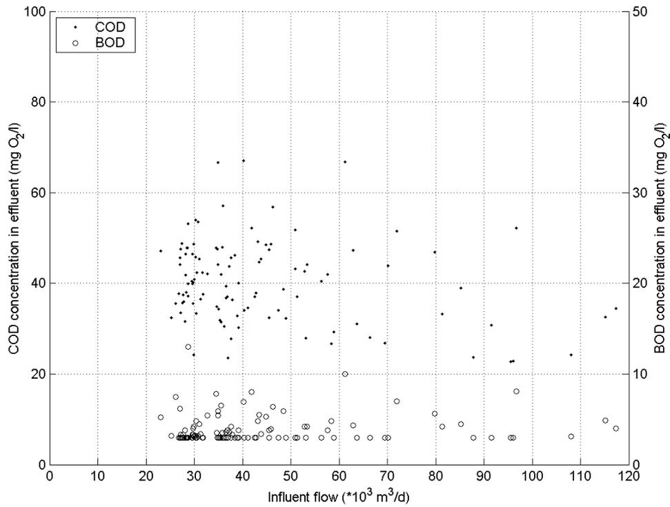
**Figure I.2** Wwtp Wervershoof. Influent flow vs effluent COD and BOD concentration. Average dwf is  $35,000 \text{ m}^3/\text{d}$ .
