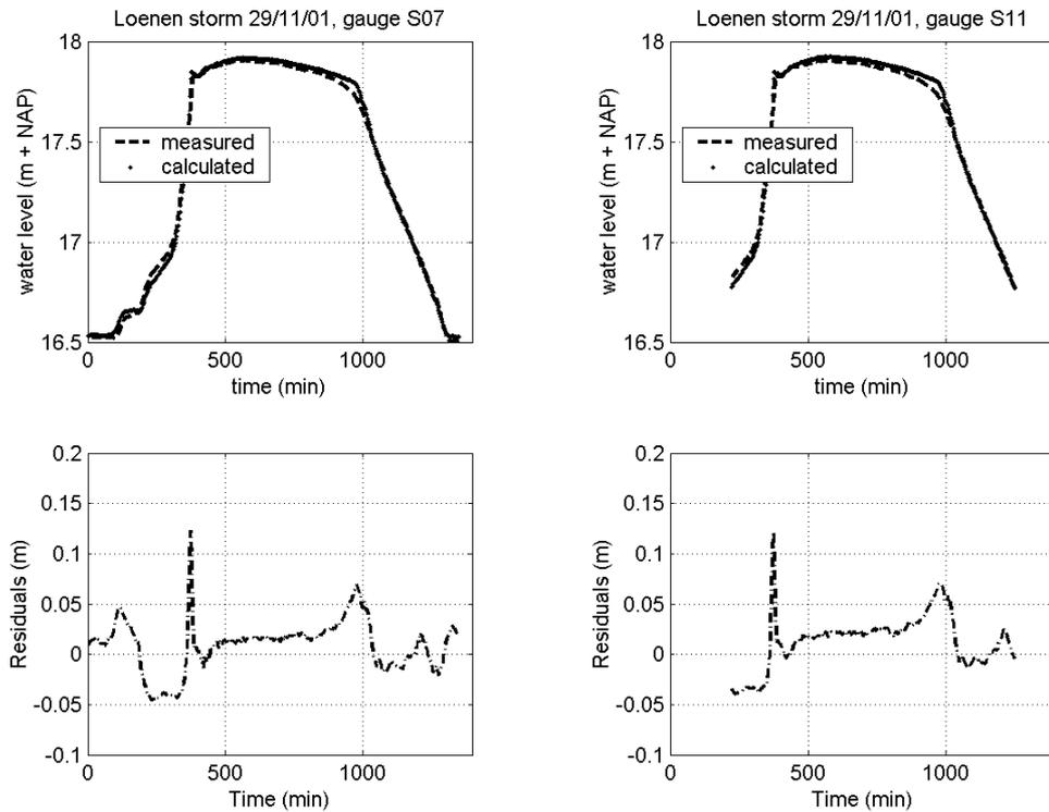
**Figure X.52** Residuals storm 29/11/01, gauge S07 (left) and gauge S11 (right).
