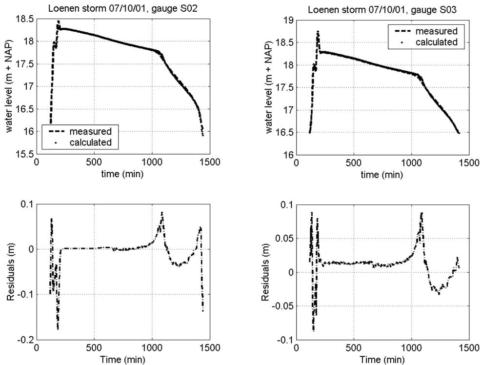
Figure X.38 Residuals storm 07/10/01, gauge S02 (left) and gauge S03 (right)
