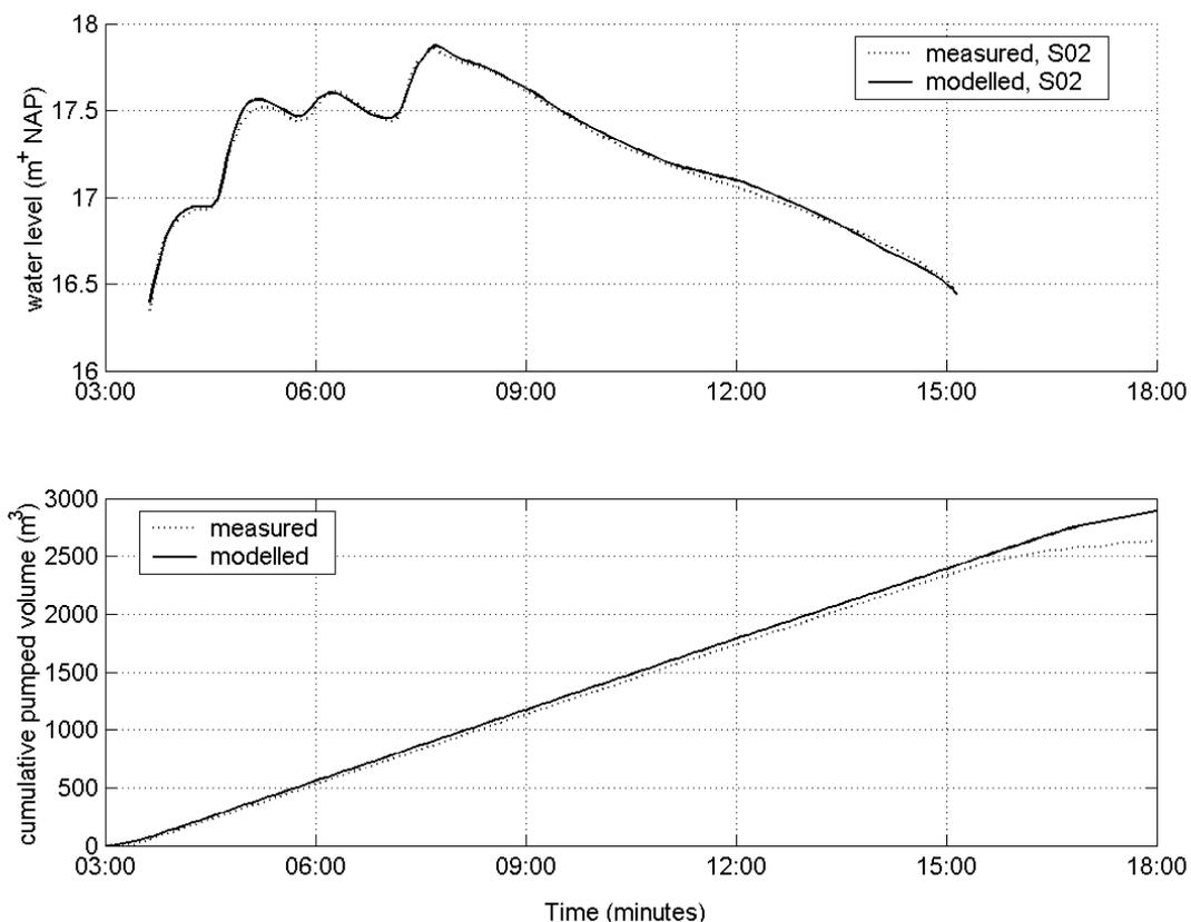
**Figure 4.12** Cumulative pumped volumes for storm 18/07/01. The upper graph shows the measured and simulated water levels for gauge S02, the level gauge nearest to the pumping station. Just after 15:00 hour, the water level dropped below the level gauge. The lower graph shows the measured and modelled pumped volumes.
