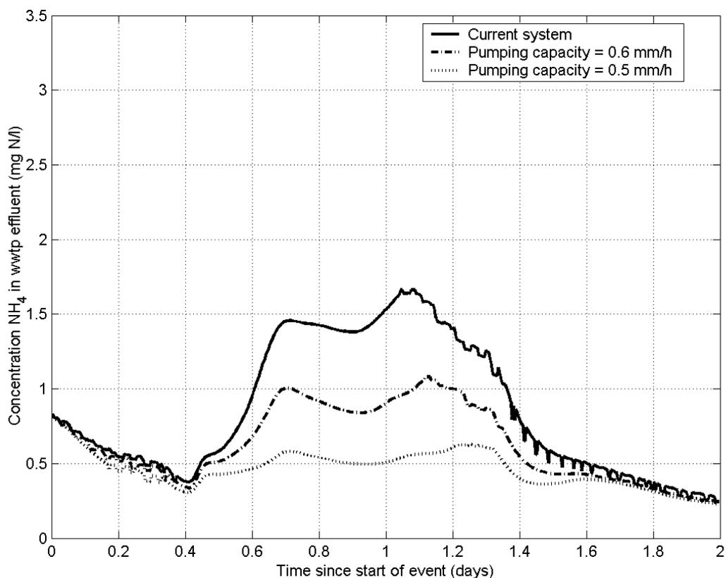
**Figure 6.20** Effect of decreasing the pumping capacity on ammonium concentration in wwtp effluent. Storm event A, ( $T = 1 \text{ y}^{-1}$ ), starting time of storm event 08:00 hour.
