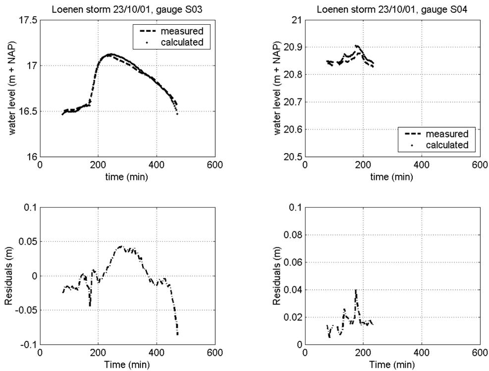
Figure X.42 Residuals storm 23/10/01, gauge S03 (left) and gauge S04 (right).
