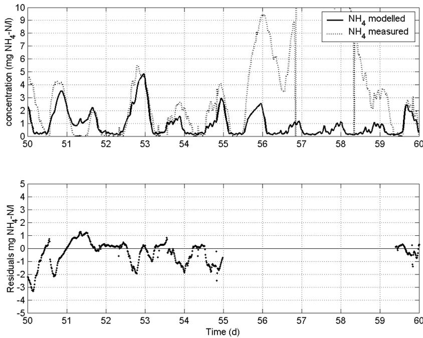
**Figure VI.6** Modelled vs measured ammonium concentration in AT effluent. Day 50 to 60 (8 November to 18 November). From day 55 to day 59 the aeration and controls were under repair, resulting in an extremely high (up to 10 mg N/l) ammonium concentration in the AT effluent.
