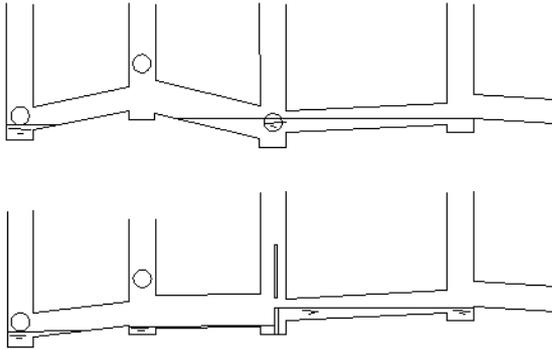
**Figure 6.1** 'Lost storage' in sewer systems due to subsidence (top) and control structures (bottom) (reproduced with permission from [Clemens (2001a)]).
