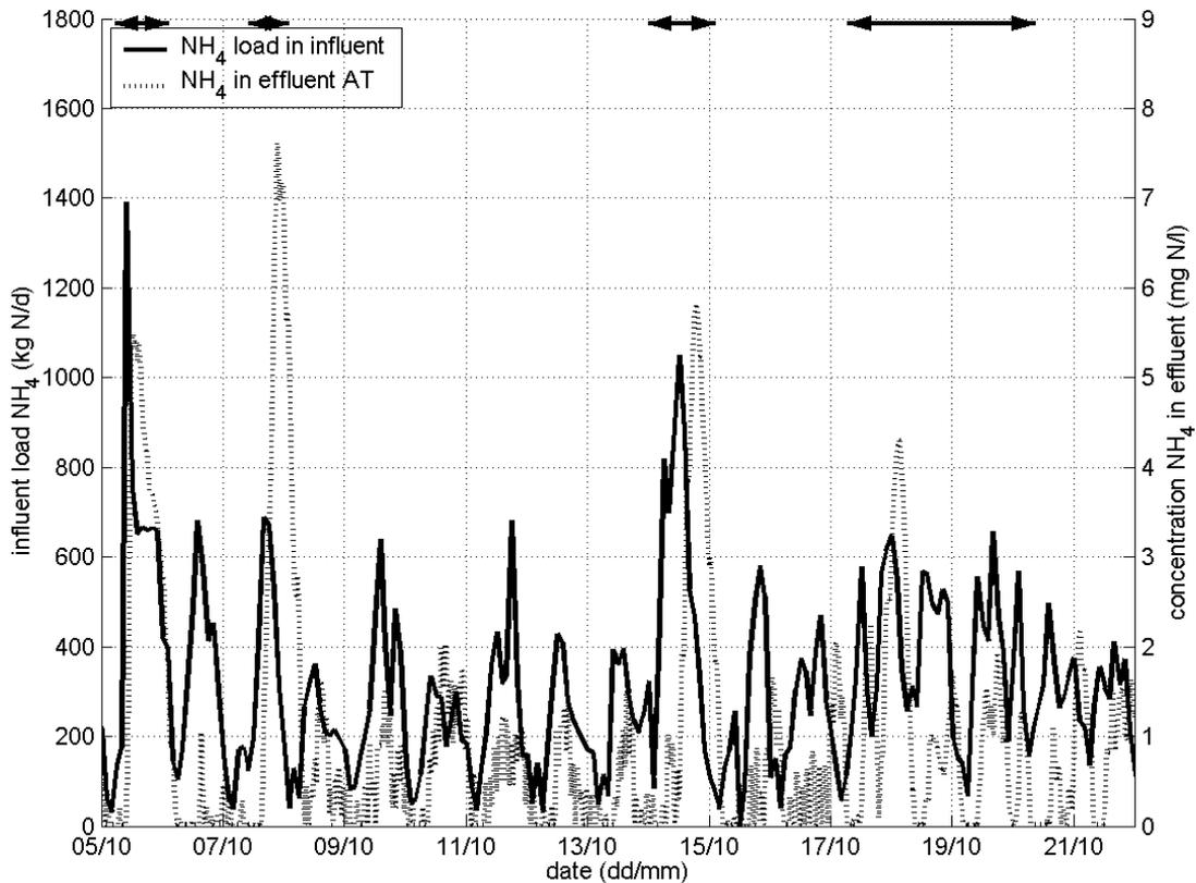
**Figure 3.13** Ammonium load in influent (kg N/d) and ammonium concentration (mg N/l) in effluent aeration tank (AT). The arrows indicate storm events. Peaks in ammonium concentration in AT effluent do coincide with peaks in influent ammonium load. However, on some occasions, a high observed peak in the influent load, e.g. on 06/10, apparently does not cause the effluent quality to decrease. This peak in the influent may be due to low quality sensor readings from the ammonium influent sensor.
