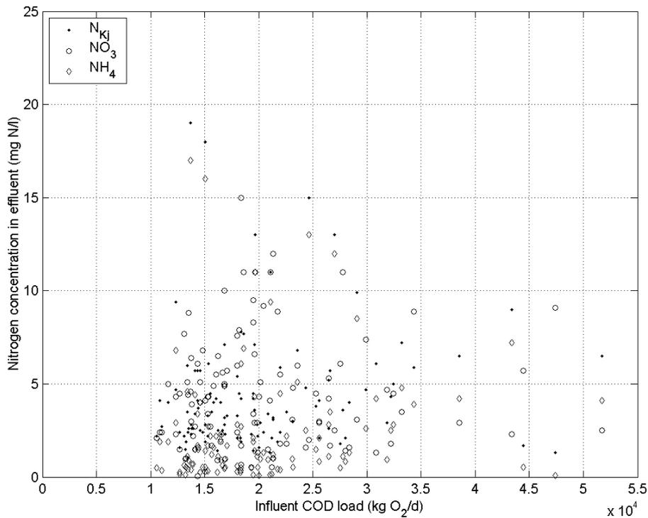
**Figure I.3** Wwtp Wervershoof. Influent COD load vs effluent nitrogen concentrations. Average dwf loading is  $17,000 \text{ kg COD}/\text{d}$ .
