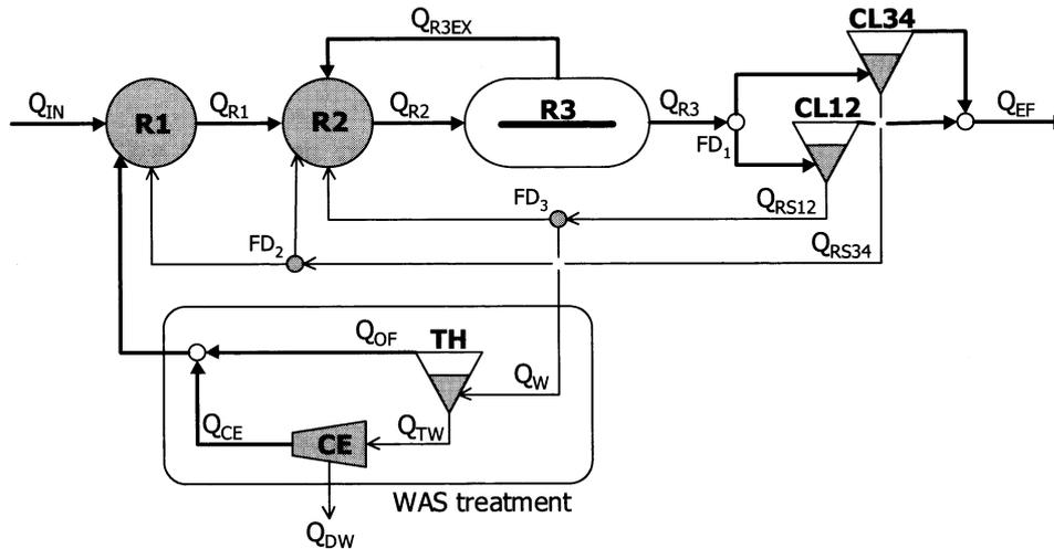
**Figure 3.17** Lay-out of wwtp Katwoude. R1: selector reactor, R2: anoxic reactor, R3: aerated carousel reactor, CL: secondary clarifiers, TH: sludge thickener, CE: sludge dewatering centrifuge, FD: flow dividers. Reproduced with permission from [Meijer (2004)]. Aeration is controlled by oxygen setpoints in the aeration tank.
