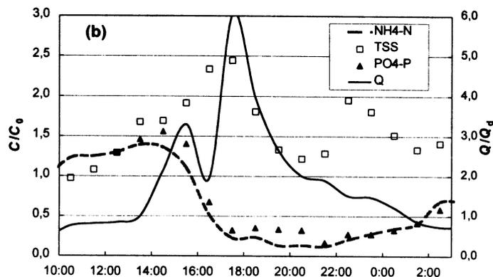
**Figure 2.5** Fluctuations during wwf of flow rate, ammonia, TSS and PO<sub>4</sub> concentration normalised with daily averages. [Reproduced with permission from: Krebs *et al.* (1999)].
