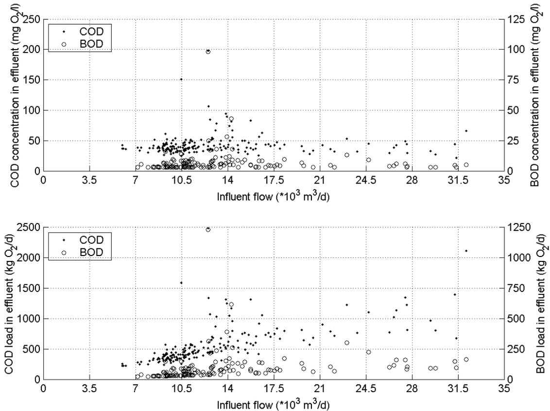
**Figure 3.2** Influent flow vs. effluent concentrations BOD and COD (upper graph) and loads of BOD and COD in the effluent (lower graph), measured in 24 h flow proportional 24 hour samples. The effluent load of COD increases with the influent flow, although this effect is only due to the increased effluent flow, as the effluent concentrations do not increase with the flow.
