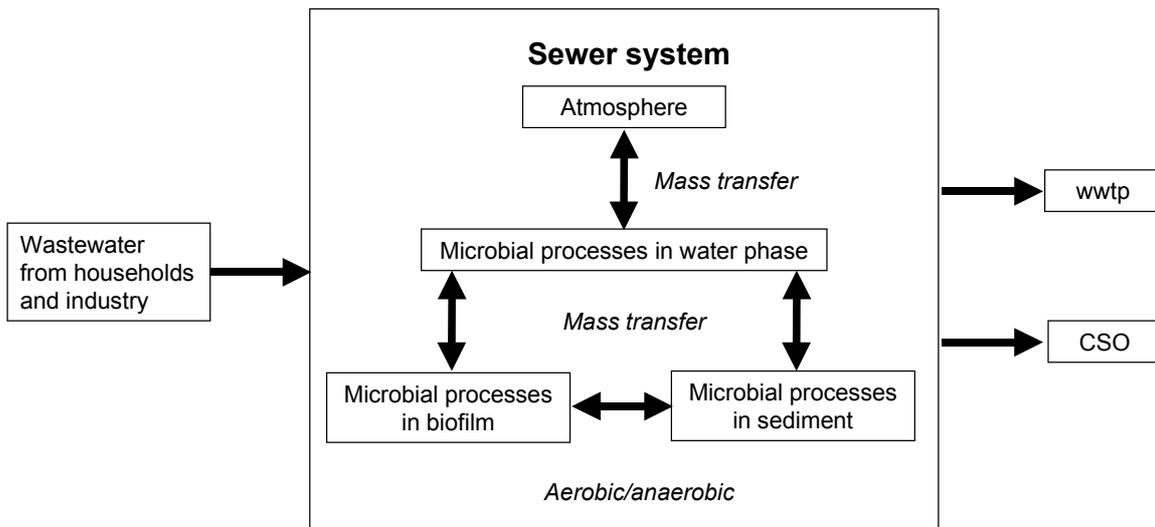
**Figure 2.9** Processes within the sewer system (after: [Tanaka (1998)]).
