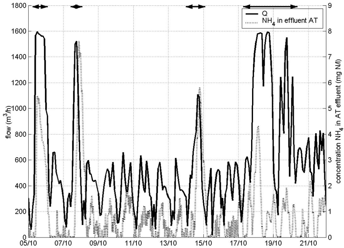
**Figure 3.12** Influent flow ( $\text{m}^3/\text{h}$ ) and ammonium concentration ( $\text{mg N/l}$ ) in effluent aeration tank (AT). The arrows indicate storm events. Peaks in flow seem to coincide with peaks in AT effluent concentration. However, the decrease in the ammonium concentration in the AT effluent during the large storm event of 18 October can not be explained by flow records only.
