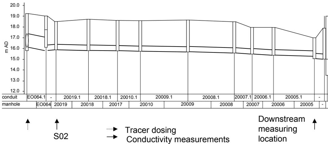
**Figure 4.15** Loenen, 454 m reach (distance between measuring locations),  $\varnothing$  0.5 m. The numbers of the gauges refer to figure 4.1.
