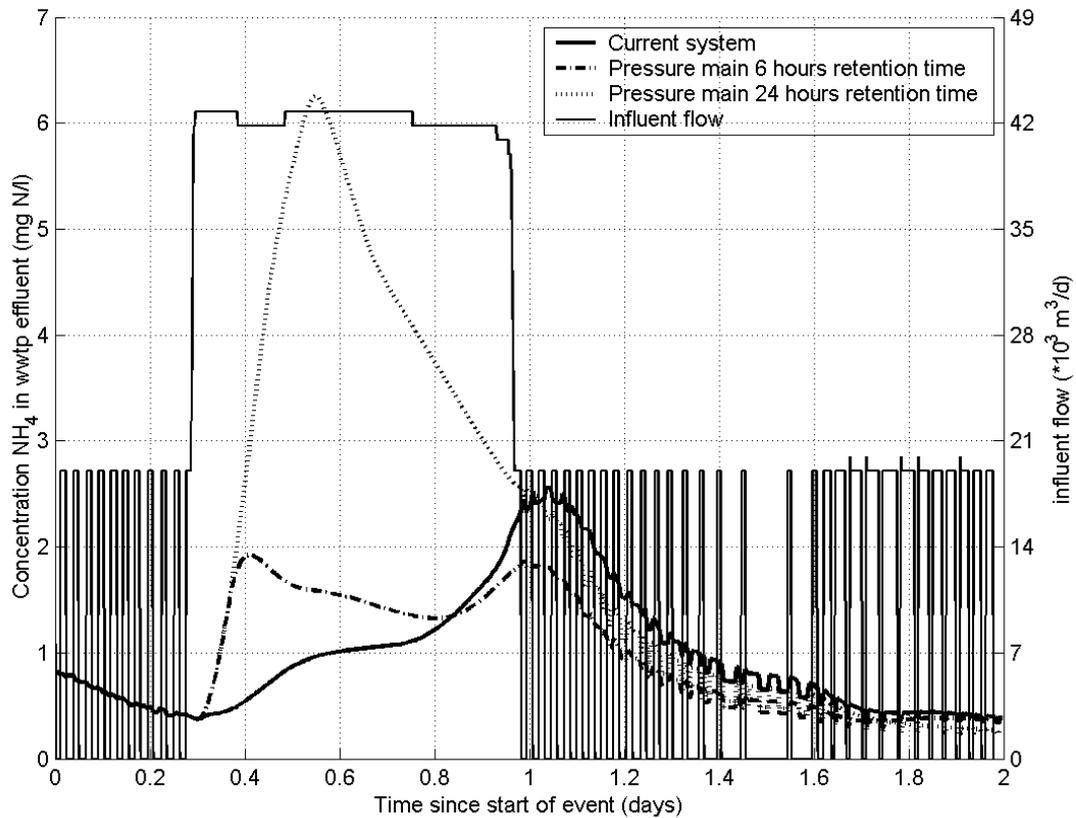
**Figure 6.22** Effect of pressure main induced peak loading of the wwtp on the ammonium concentration in wwtp effluent. This effect is due to the fact that wastewater with a dwf concentration arrive at the wwtp with wwf flow rate at the onset of a storm event. Consequently, the longer the hydraulic retention time of the pressure main, the stronger the effect. Storm event A, starting at 22:30 hour.
