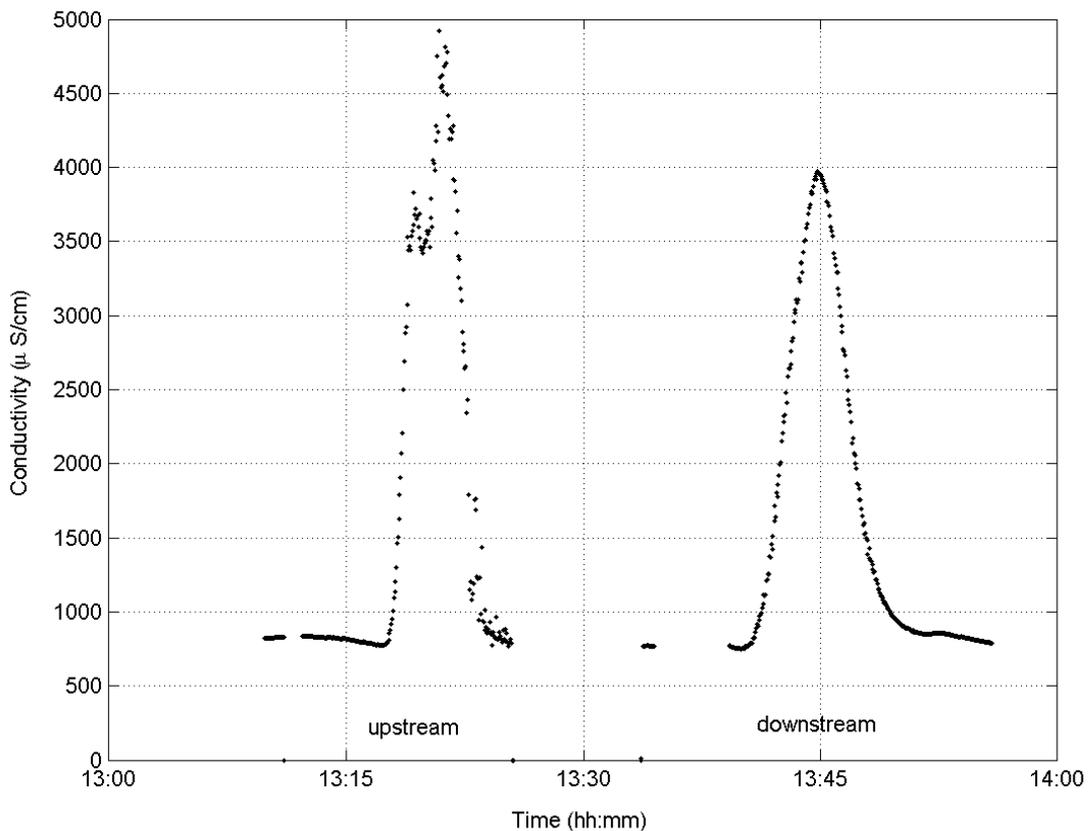
**Figure 4.18** Measured conductivity tracer experiment Loenen 14 December 2001, reach 233 m. In the upstream measurements two peaks can be distinguished. This is due to the fact that the tracer was dosed two times within 3 minutes time. At the downstream measuring location the two peaks are not distinguishable anymore.
