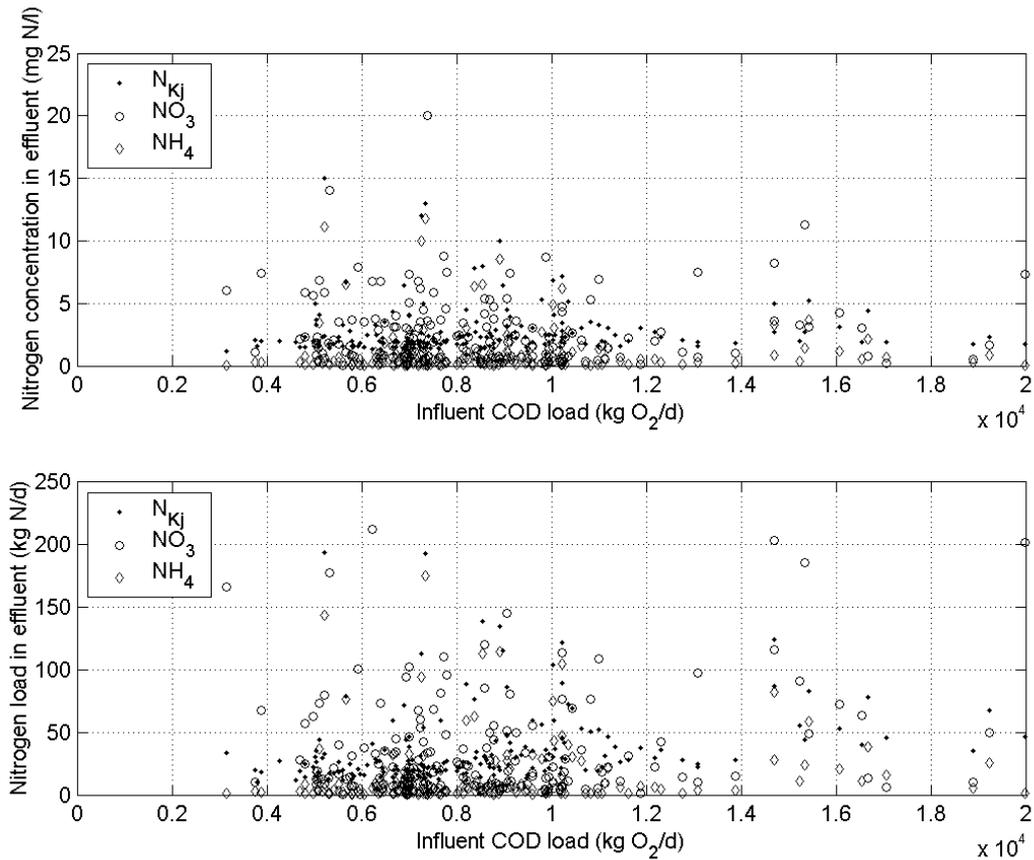
**Figure 3.6** Influent COD load vs. effluent nitrogen concentrations (upper graph) and effluent nitrogen loads (lower graph). Concentrations are measured as 24 hour flow proportional composite samples. Again, high nitrogen concentrations in the effluent cannot be explained by a high influent load.
