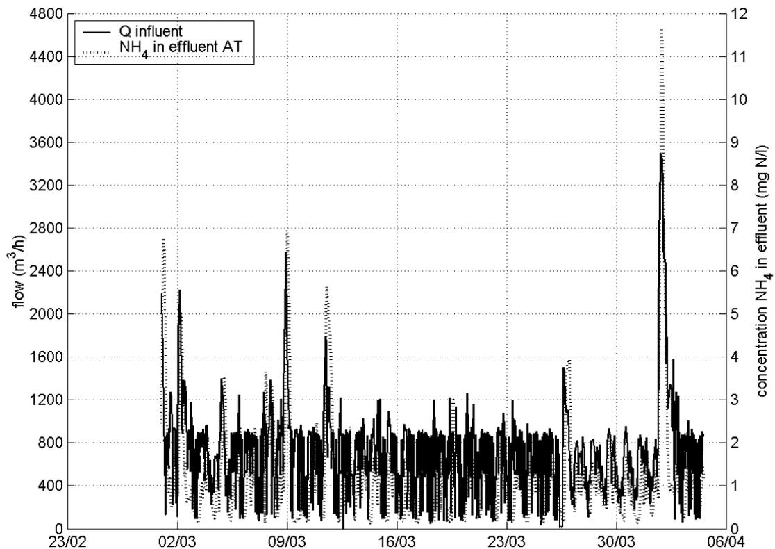
**Figure 2.7** Effluent ammonium concentration vs. influent flow, measured at wwtp Hoek van Holland, 28 February to 4 April 2003. Fluctuations in effluent quality for ammonium seem to be correlated to high influent flows as each time the influent flow rises above  $1200 \text{ m}^3/\text{h}$  the ammonium concentration in the effluent rises. Data from [Veldt, van der (2003)].
