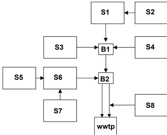
**Figure 5.5** Lay out of the waste water system of combined sewer systems, interceptor sewers, booster pumps and WWTP. Table 5.1 lists the most important system characteristics.
