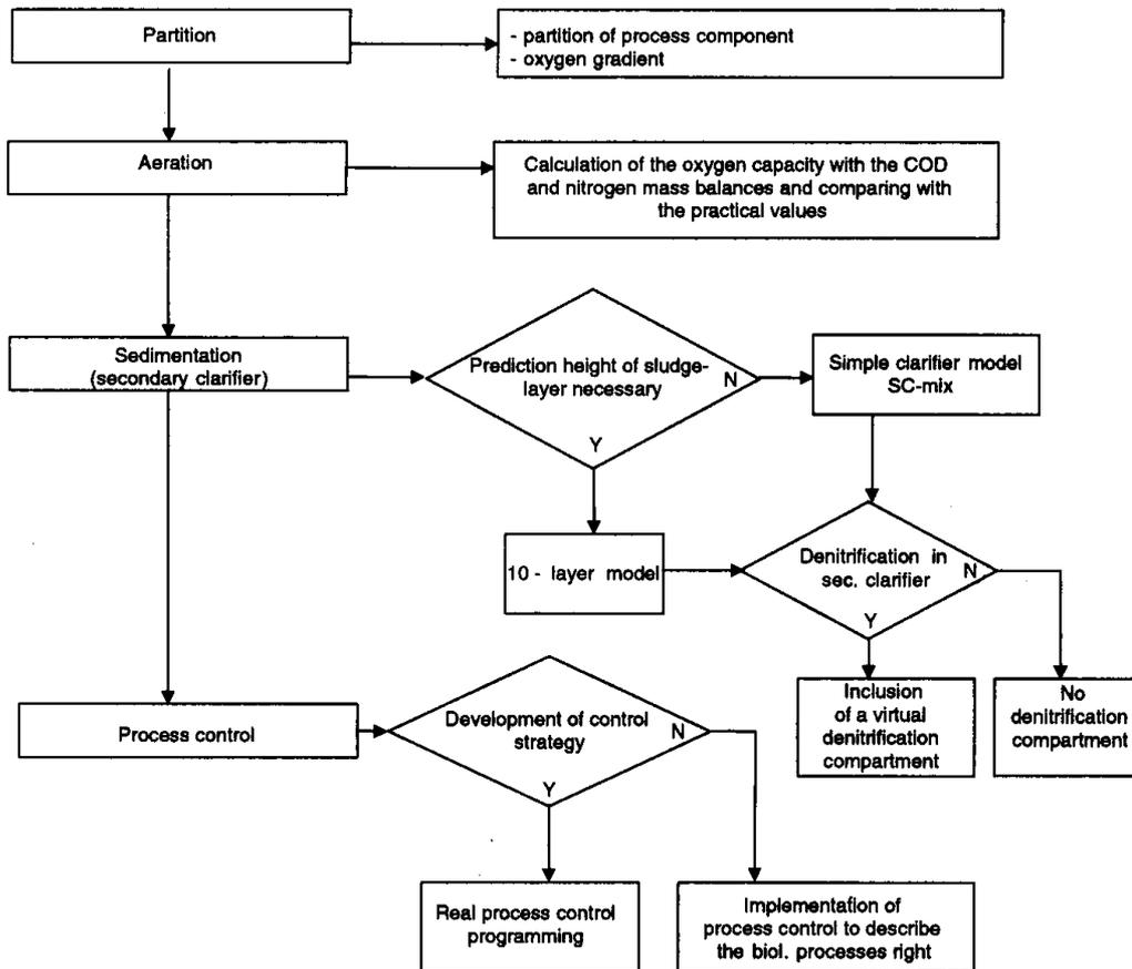
Figure IV.4 Phase IV. Model structure.
