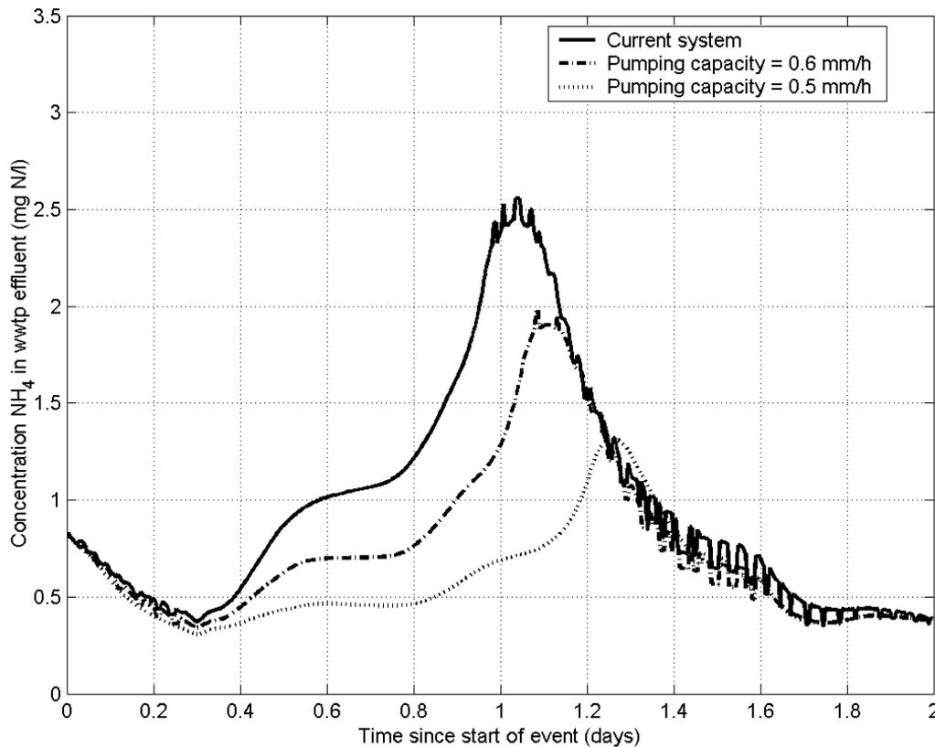
**Figure 6.19** Effect of decreasing the pumping capacity on ammonium concentration in wwtp effluent. Storm event A, ( $T = 1 \text{ y}^{-1}$ ), starting time of storm event 22:30 hour.
