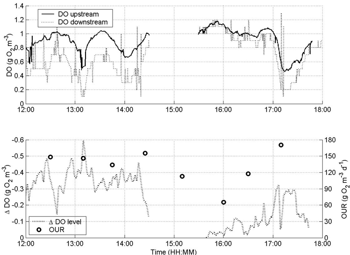
**Figure 4.44** Experiment Beekbergen, reach Wippenpol, 16/09/03. Oxygen levels in upstream and downstream manhole (top) and the decrease in oxygen level and the OUR of the sewage (down). The measured values of the downstream manhole were plotted with a time shift equal to the calculated mean travel time. The horizontal lines of the downstream dissolved oxygen concentration are due to the downstream oxygen sensor saving the oxygen concentration with only one decimal.
