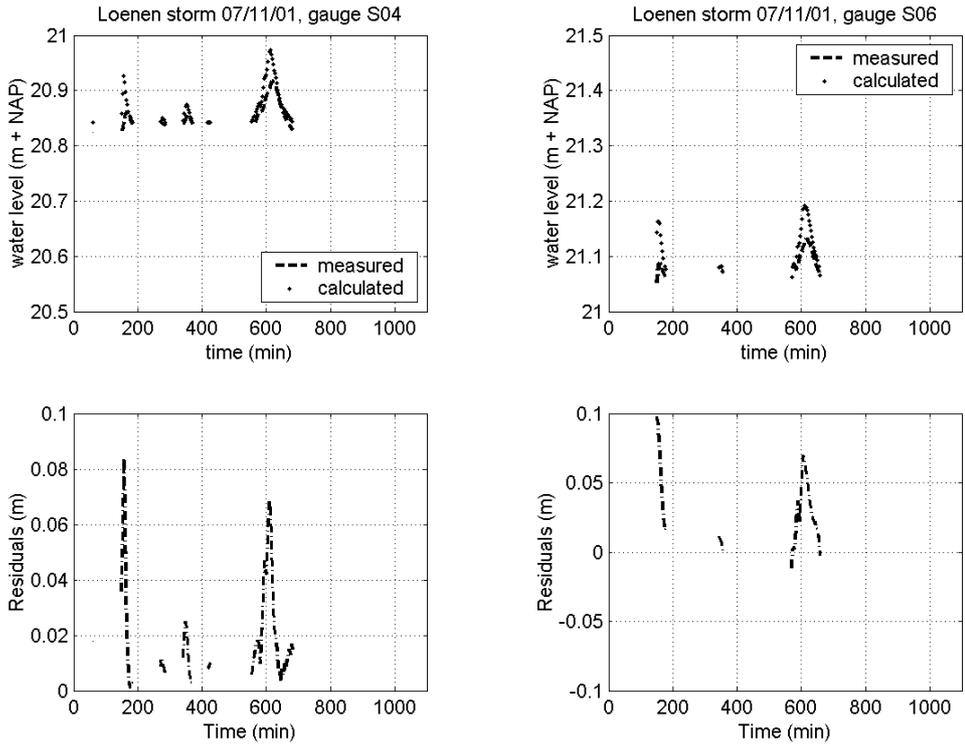
**Figure X.47** Residuals storm 07/11/01, gauge S04 (left) and gauge S06 (right).
