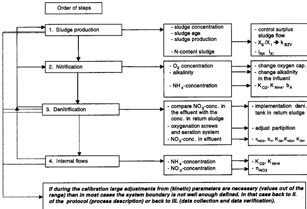
Figure IV.6 Phase VI. Calibration.
