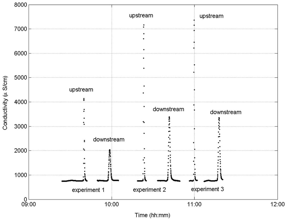
**Figure 4.16** Measured conductivity tracer experiments Loenen 14 December 2001, reach 454 m. The dosed NaCl solution causes distinctive peaks above the background conductivity of approximately 700  $\mu$ S/cm
