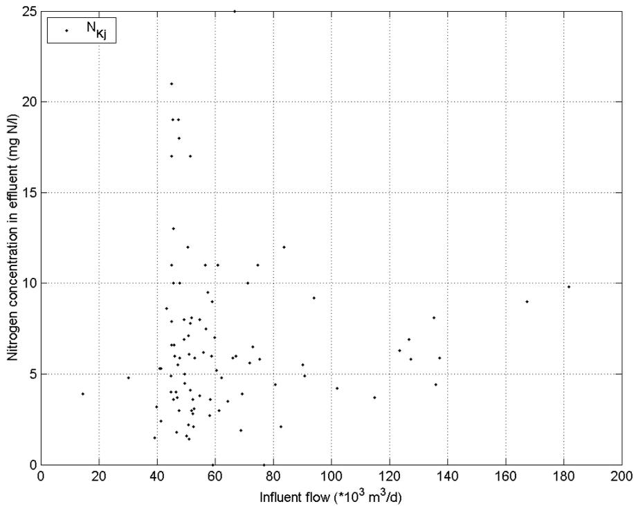
**Figure I.9** Wwtp Utrecht. Influent flow vs effluent nitrogen concentration. Average dwf is 45,000 m<sup>3</sup>/d.
