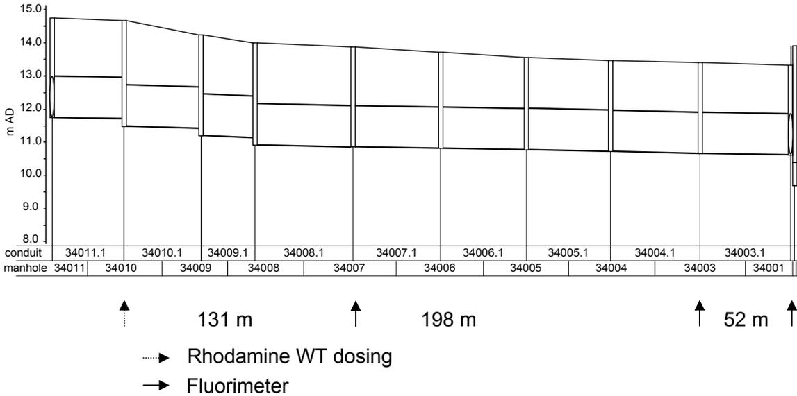
**Figure 4.20** Tracer experiment Beekbergen, reach 'Wippenpol',  $\varnothing$  1.25 m.
