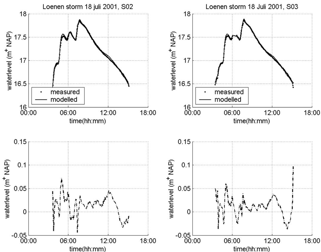
**Figure 4.4** Measured and modelled water levels during the storm of 18/07/01 in Loenen. The numbers of the measuring locations refer to the sites shown in figure 4.1.
