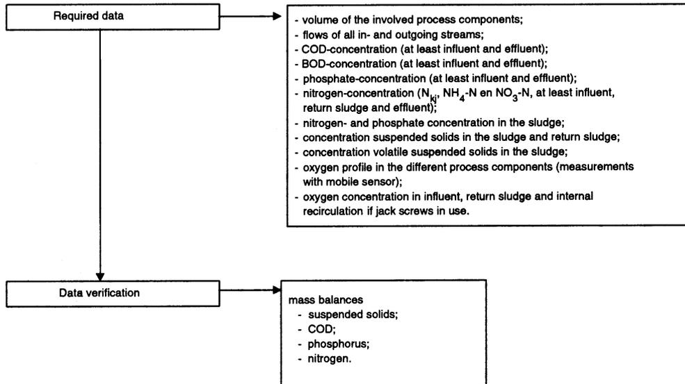
Figure IV.3 Phase III. Data collection and verification.
