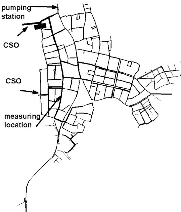
**Figure 4.24** Sewer system (schematic) of Ulvenhout with the measuring location.
