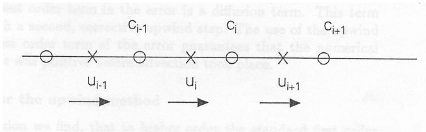
**Figure XIII.1** Staggered grid used. Arrows indicate fluxes at cell boundaries.
