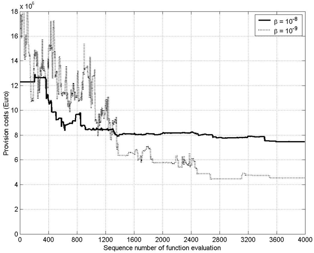
Figure 5.8 Optimisation results simulated annealing.
