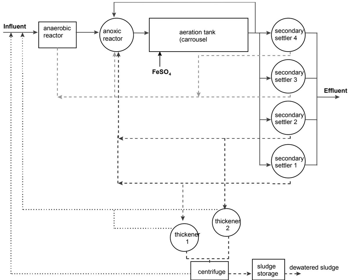
**Figure 3.3** Schematic layout of wwtp 'Katwoude'.
