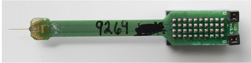
Figure 4.11: NeuroNexus a1x32-5mm-25-177 Electrode Array used for in vitro measurements of the prototype PCB.
