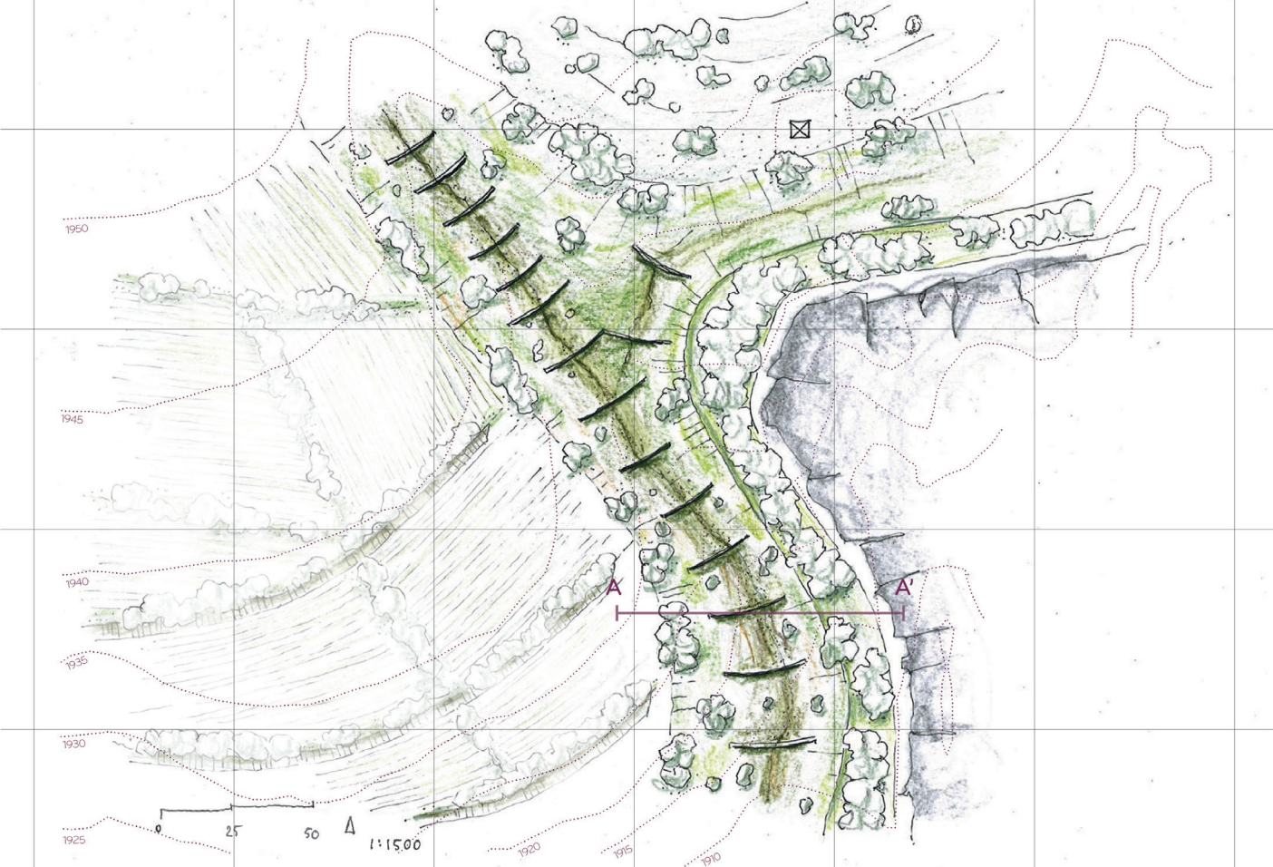
[Figure 135.] Map of proposed gully rehabilitation next to the dump, visualized during wet and dry season.
