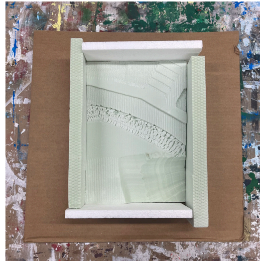
[Figure 174.] Developing a negative mold for the model.
