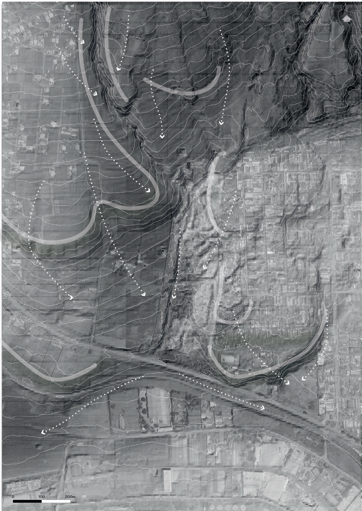
[Figure 114.] Schematic overview of the natural depressions in the upstream area, that will guide the final design outcome
