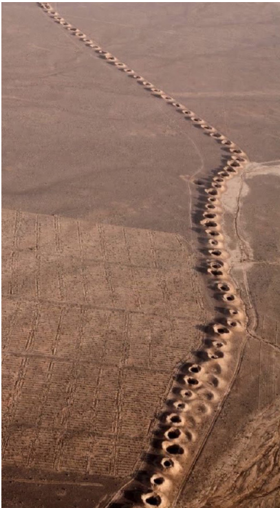
[Figure 1.] Ancient irrigation system Qanat in arid landscapes to transport groundwater from underground aquifers to human settlement at surface-level over long distances (by author); [Figure 2.] Qanat system visible at the surface; photo by Alireza Teimoury (Watson, 2019).
