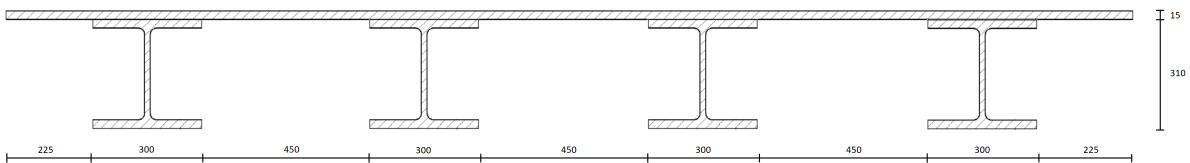
Figure 5.1: Cross section of footbridge used in thesis. Cross beams may be needed, but not considered at this stage except for increase in self weight
