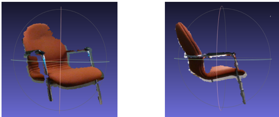
Figure 4.9: Point clouds of a chair captured from camera1 (left) and camera2 (right)
