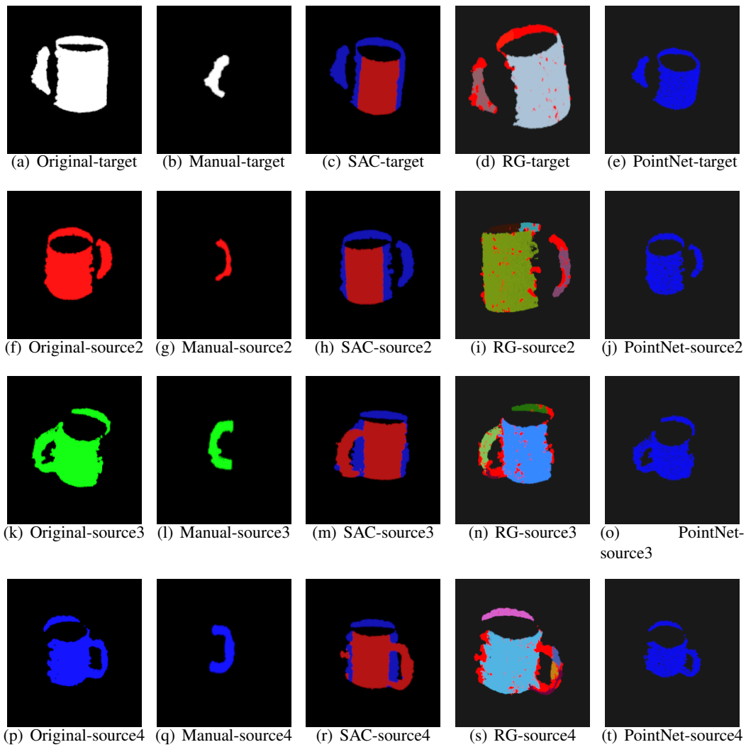
Figure 5.9: Mug Point Cloud Segmentation Results. The point clouds in each column from left to right are original, manual segmentation, plane model-based SAC segmentation, region growing, and PointNet++ segmentation results.
