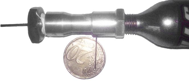
Fig. 18. Prototype in pneumatic configuration connected to a 16 grams  $CO_2$  cartridge and a 20 Euro Cent coin for comparison.
