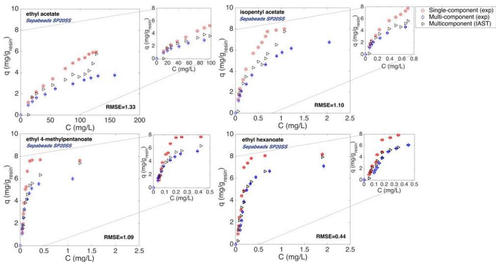
Figure 5.2. Comparison of experimental single-component adsorption isotherms with Experimental multi-component adsorption isotherms and IAST prediction; Adsorption on Sepabeads SP20SS at  $T=284.15$  K
