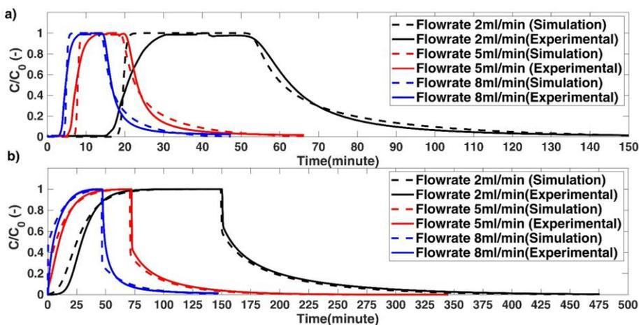
Figure 6.3. Influence of flow-rate on single-component adsorption of ethyl acetate on a 3 cm column; a) Sepabeads SP20SS b) Amberlite XAD16N
