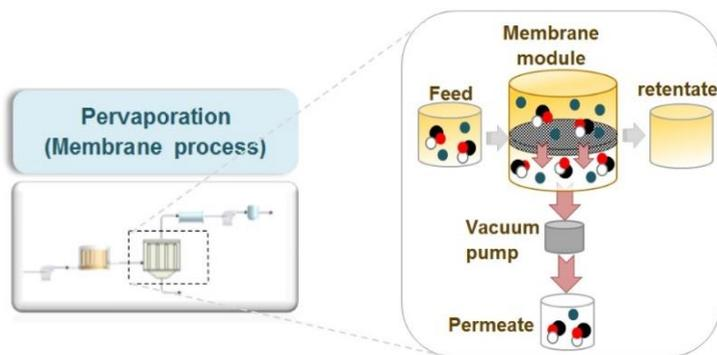
Figure 2.5 Pervaporation membrane technique based on vapor/liquid equilibrium
