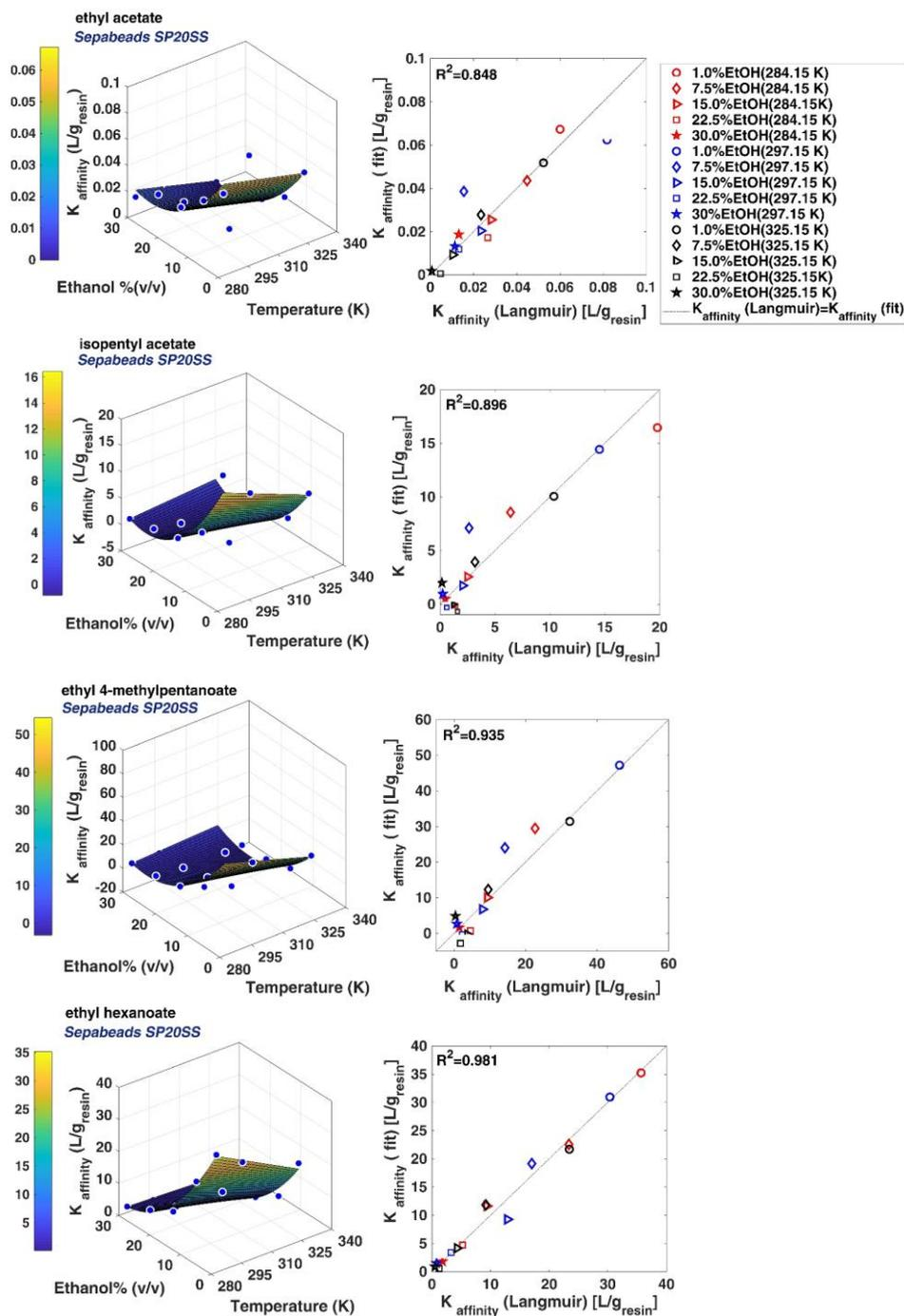
Figure 4.9.  $K_{\text{affinity}}$  as function of temperature and ethanol% (v/v), adsorption on Sepabeads SP20SS
