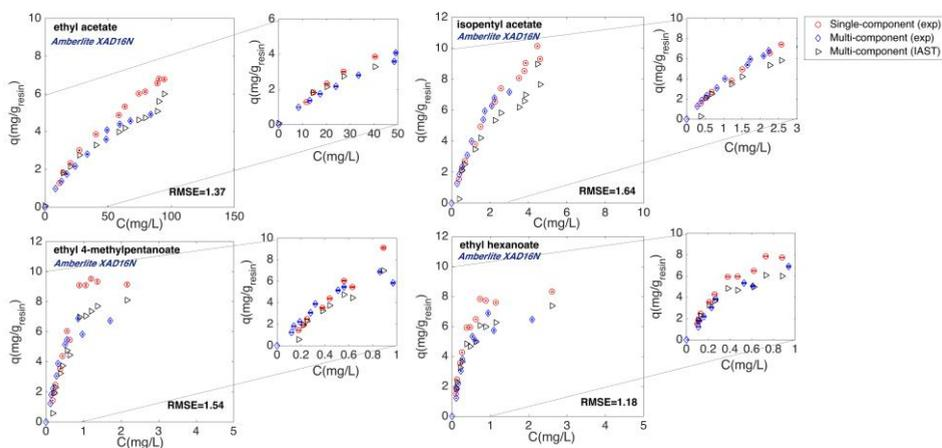
Figure 5.3. Comparison of experimental single-component adsorption isotherms with Experimental multi-component adsorption isotherms and IAST prediction; Adsorption on Amberlite XAD16N at  $T=284.15$  K
