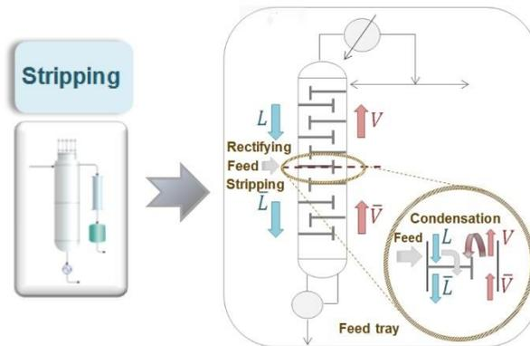
Figure 2.3 Distillation/Stripping technology based on vapor/liquid equilibrium
