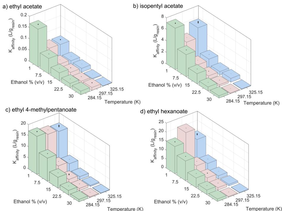
Figure 4.8.  $K_{\text{affinity}}$  as function of temperature and ethanol concentration, adsorption on Amberlite XAD16N; a) ethyl acetate b) isopentyl acetate c) ethyl 4-methylpentanoate d) ethyl hexanoate
