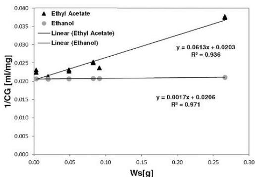
Figure A.5. Reciprocal of concentration in the gas phase vs. Mass of the resin; SPRV method
