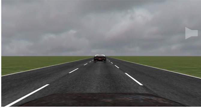
Figure 1. Driving simulator screen shot taken during the car following divided attention task. The divided attention stimulus is the gray symbol shown on the right hand side.
