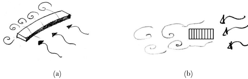
Figure 2. 14 (a) VIV on a section of the bridge Tacoma Narrows. (b) VIV on a cross-section of the bridge Tacoma Narrows.
