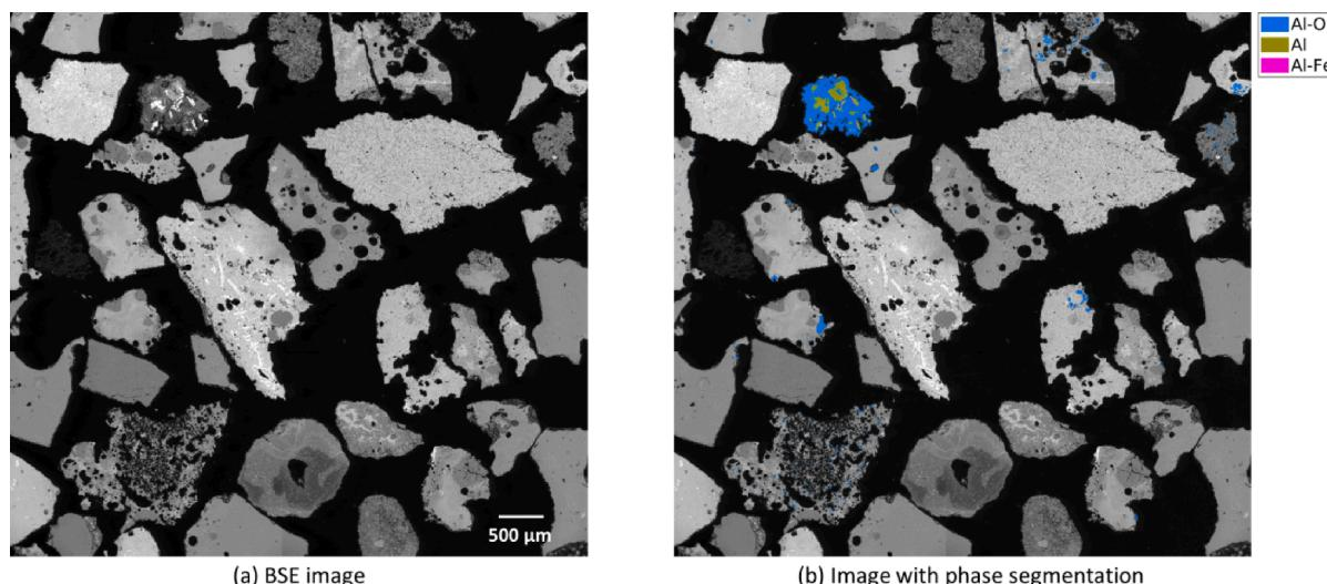
**Fig. 4.** A representative overview of weathered MSWI bottom particles in the 0.5–1.6 mm size fraction, covering an area of 36 mm<sup>2</sup>: (a) BSE image; (b) Image obtained after phase segmentation. In this image, labels are as follows: “Al-O” for oxidized Al, “Al” for metallic Al, and “Al-Fe” for Al-Fe alloy.
