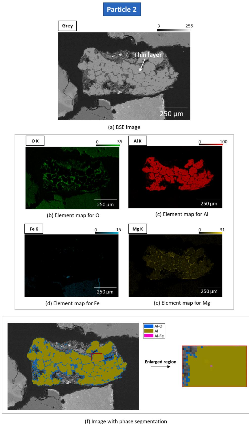
**Fig. 6.** Typical morphology of weathered MSWI bottom ash particle containing metallic Al (particle 2): (a) BSE image (pixel scan field  $512 \times 340$ , area:  $0.7 \text{ mm}^2$ ); (b)–(e) EDS element maps; (f) Image obtained after phase segmentation. In this image, labels are as follows: “Al-O” for oxidized Al, “Al” for metallic Al, and “Al-Fe” for Al-Fe alloy.
