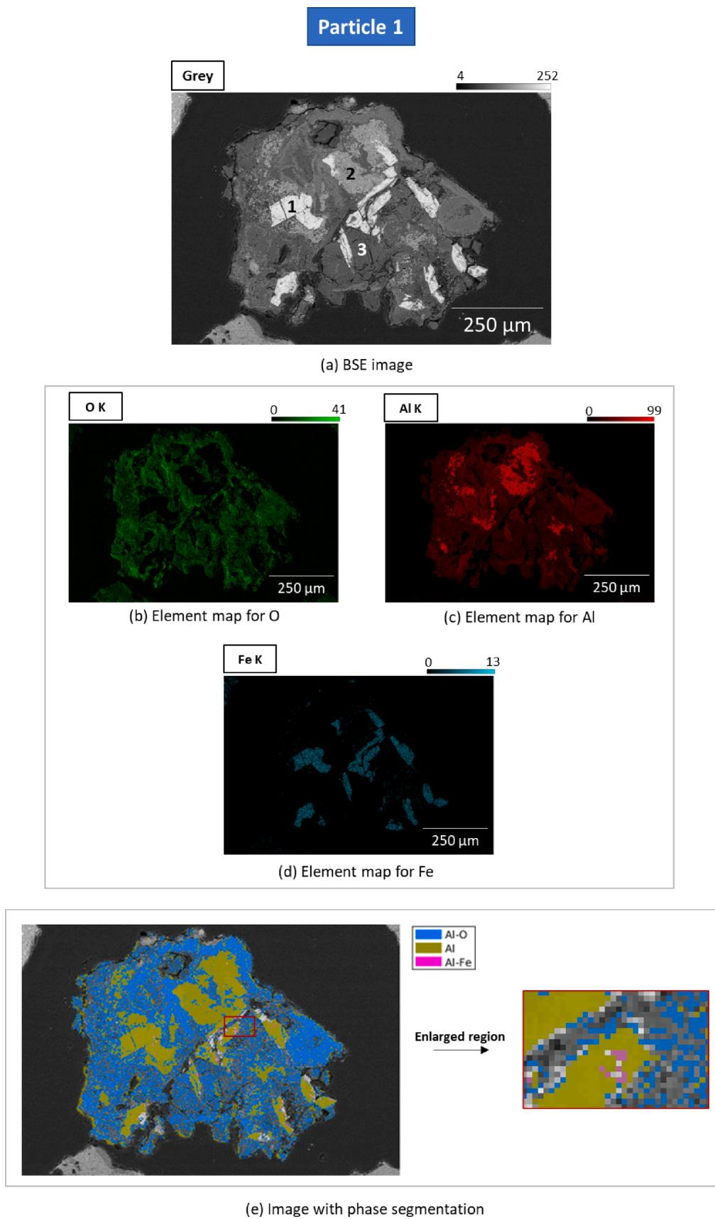
**Fig. 5.** Typical morphology of weathered MSWI bottom ash particle containing metallic Al (particle 1): (a) BSE image (pixel scan field  $512 \times 340$ , area:  $0.7 \text{ mm}^2$ ); (b)–(d) EDS element maps; (e) Image obtained after phase segmentation. In this image, labels are as follows: “Al-O” for oxidized Al, “Al” for metallic Al, and “Al-Fe” for Al-Fe alloy.
