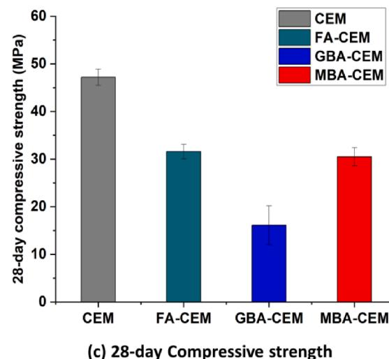
**Fig. 8.** (a) Blended cement paste samples prepared with ground weathered MSWI bottom ash (GBA-CEM); (b) Blended cement paste samples prepared with mechanical-treated weathered MSWI bottom ash (MBA-CEM); (c) 28-day compressive strength of plain cement (CEM) and blended cement paste samples. FA-CEM is blended cement paste prepared using class F coal fly ash as SCM.
