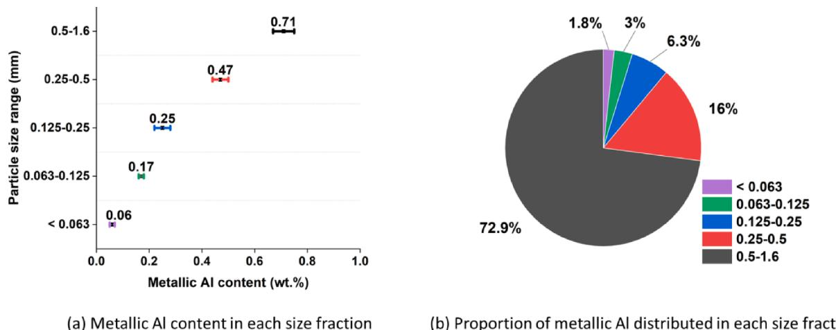
**Fig. 3.** Comparison among different size fractions of weathered MSWI bottom ash regarding (a) metallic Al content measured by water displacement method; (b) proportion of metallic Al calculated by considering the metallic Al content in each size fraction and the respective weight percentage of that size fraction in weathered MSWI bottom ash.
