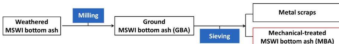
Fig. 2. Flow chart of mechanical treatments.
