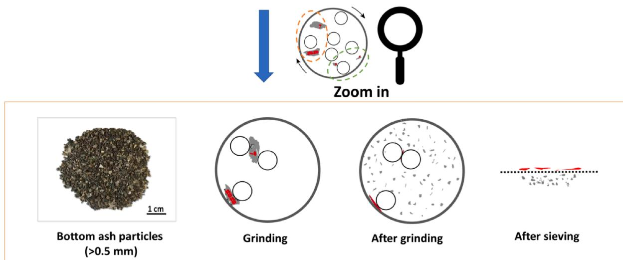
(b) Effects of mechanical treatments on large particles in weathered MSWI bottom ash
