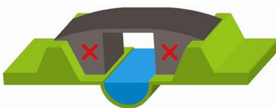
Figure 16: Removal of hydraulic obstacles
