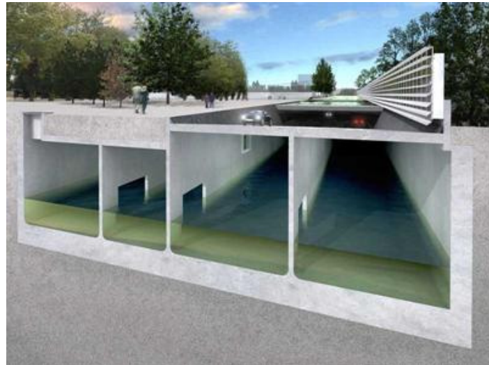
Figure 17: Underground water retention
