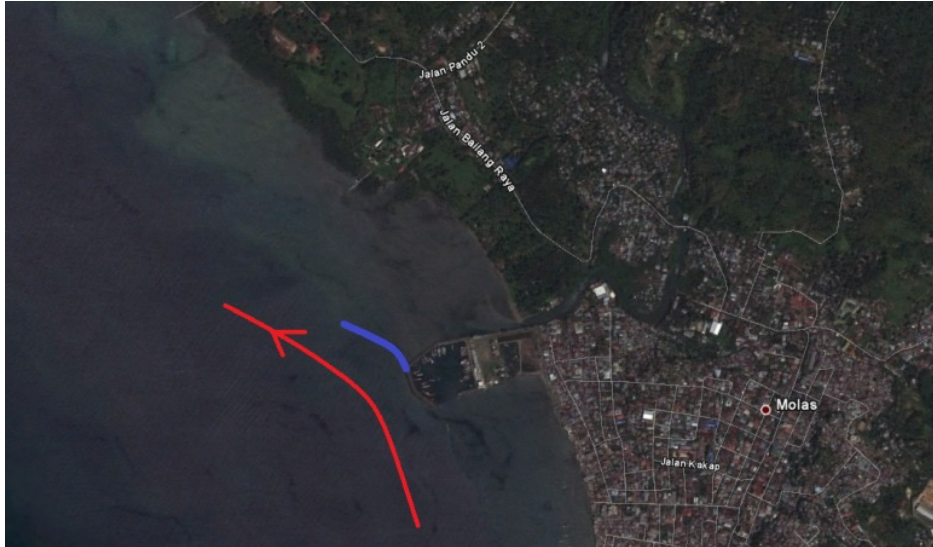
Figure 14: Rubble breakwater (bleu) and the change in current (red arrow)
