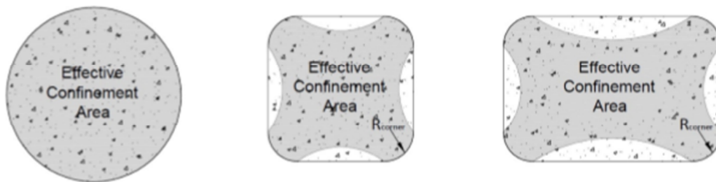
Figure 3-5 Effective confinement areas in circular, square and rectangular columns (Parvin & Brighton , 2014).
