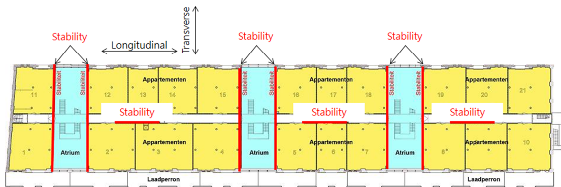
Figure 4-32 Jobsveem – Location of the stabilizing frameworks in the transverse and the longitudinal directions
