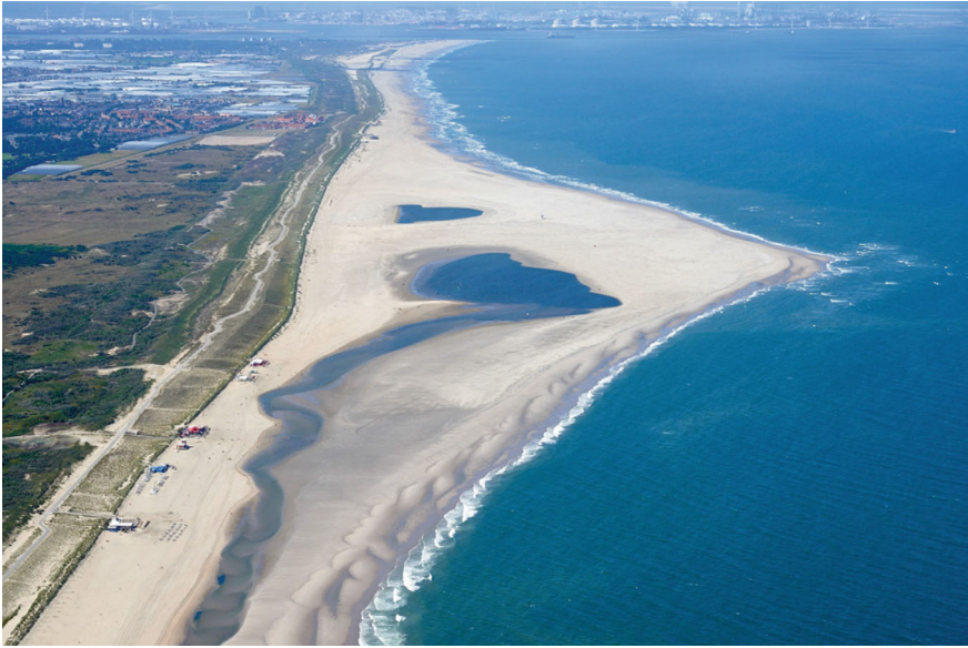
Fig. 24 Sand engine: a mega sand nourishment of more than 20 million m 3 , following the principles of Building with Nature: ocean currents, wind and waves are gradually spreading the sand along the coast and into the dunes. Source https://dezandmotor.nl
