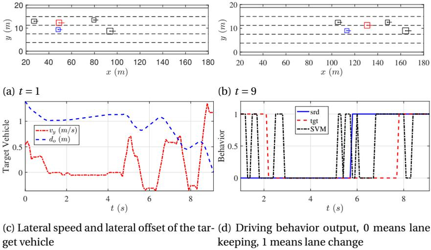
Figure 5.5: An example of the proposed behavior estimation method. The red vehicle is the target vehicle.  $d_0$  is the lateral distance of the target vehicle. The time point of a “partial” lane change of the target vehicle at  $t = 9$  s is actually considered as the ending of its lane change intention. We assume the true lane change will happen after this moment and this work is trying to do a prediction as early as possible before this moment.
