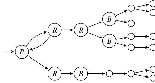
Figure 4.5: Red-Blue Framework: Starting at the root, the algorithm tries to find the smallest consistent state machine. Already identified parts of the target are marked *red*, and direct neighbors of those states as *blue*. The heuristic focuses on the fringe of the marked states, instead of having to check all possible combinations of states.
