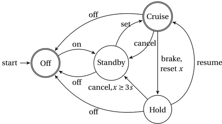
Figure 2.5: A timed deterministic finite state automaton models a simplified cruise controller. The transition from *Hold* to *Standby* relies on the additional time guard checking. The controller will stay at *Hold* when *Cancel* is executed but for no more than 3 seconds.
