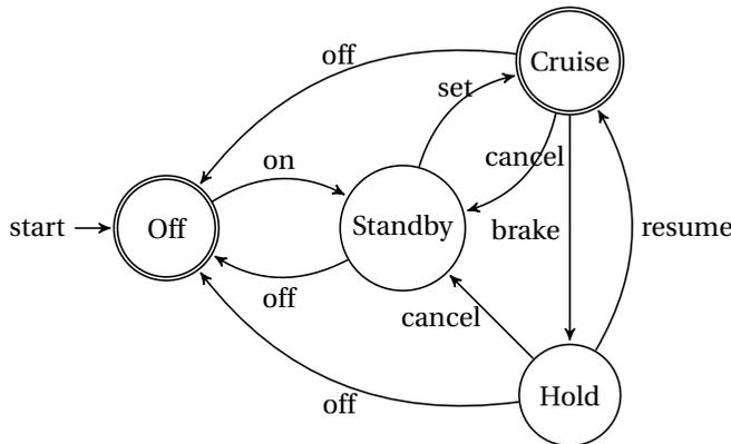
Figure 2.2: A deterministic finite state automaton models a simplified cruise controller. This example is adopted and revised from (Aström and Murray, 2010) by adding the transition from *Hold* to *Standby*.
