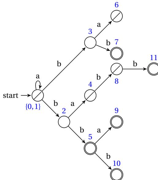
Figure 2.10: Resulting DFA after merging the states 0 and 1. We use a curly brace to represent a block merging multiple states.
