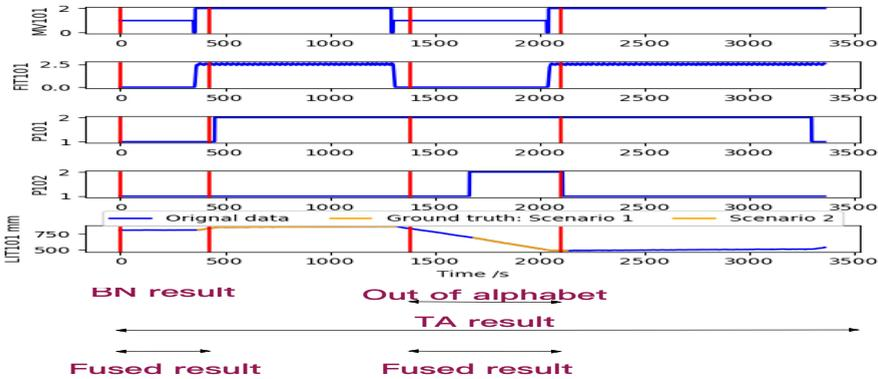
Figure 6.13: An example of fused results. The timed string of this example is (3,420)(2,960)(1,720)(3,1260), which is not fired by the TA as a whole sequence. The probability of the aligned event  $P(LIT = 3)|(MV = 1, P101 = 1) = 0$ . The actuator P102 is never seen to be open in the training data.
