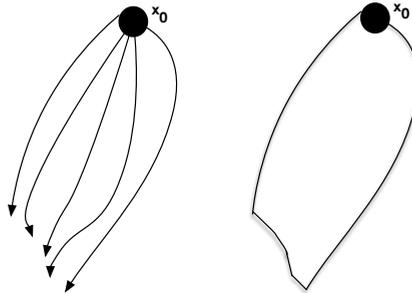
Figure 2.17: Trajectories of simulation and reachable set.
