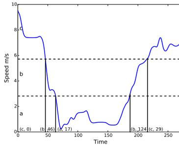
Figure 2.1: A speed record from a vehicle. The value of speed's state space is partitioned into three zones named  $a$ ,  $b$ ,  $c$ . In this case the partition is based on Voronoi cells, where in each zone, all its values are closest to its own cluster's centroid. Any clustering or discretization methods can serve as plug-and-play approaches to partition the continuous values here. The time information besides the event is the time difference between successive events.
