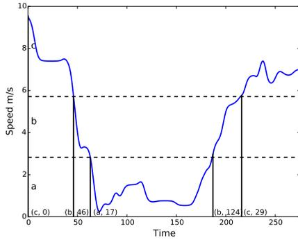
Figure 3.5: Discretization of time series data in l80-1. Instead of using complete symbolic strings with total length 275, the timed string has 5 tuples as input:  $(c,0)(b,46)(a,17)(b,124)(c,29)$ . The number next to the symbol in each tuple denotes the time difference since the last event.
