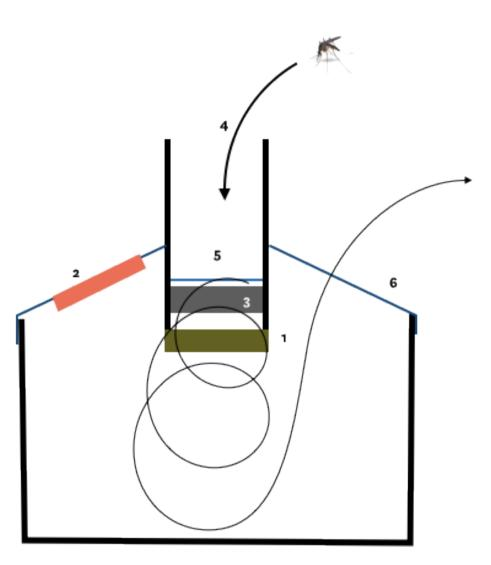
1. An odour strip is suspended in the trap, luring mosquitoes from the long (10-100m) distance.
