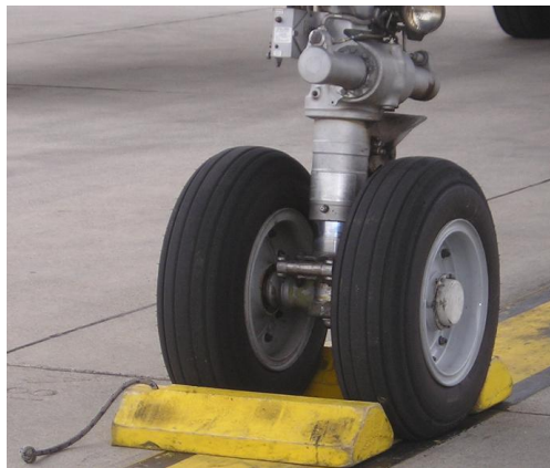
Figure 2.3: Wheel chocks placed around a nose landing gear. 2
