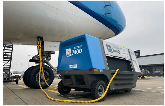
Figure 2.5: E-GPU Connected to an aircraft [29]
