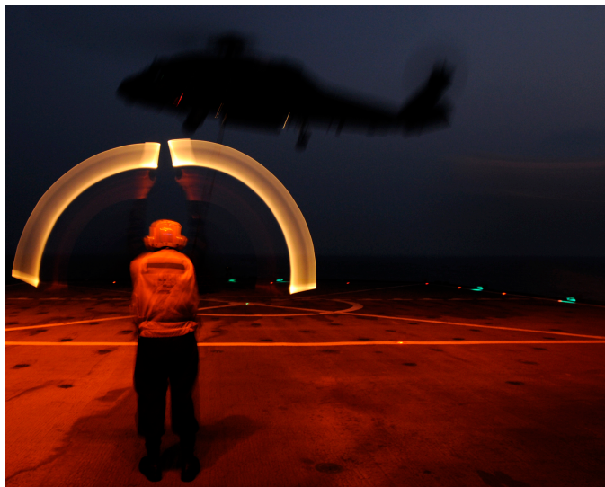
Figure 2.15: A long exposure of the usage of marshalling wands, directing a SH-60F Sea Hawk to take off
