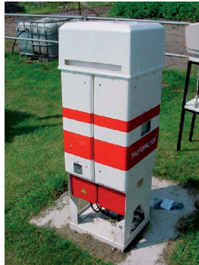
Figure 3.5: LD40 cloud height meter (photo: KNMI [2006])
