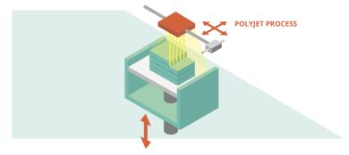
The photopolymerization group also comprises the **polyjet process** because this process contains the hardening of a low viscous photopolymerizable resin. Instead of a vat with resin, the resin is dropped
