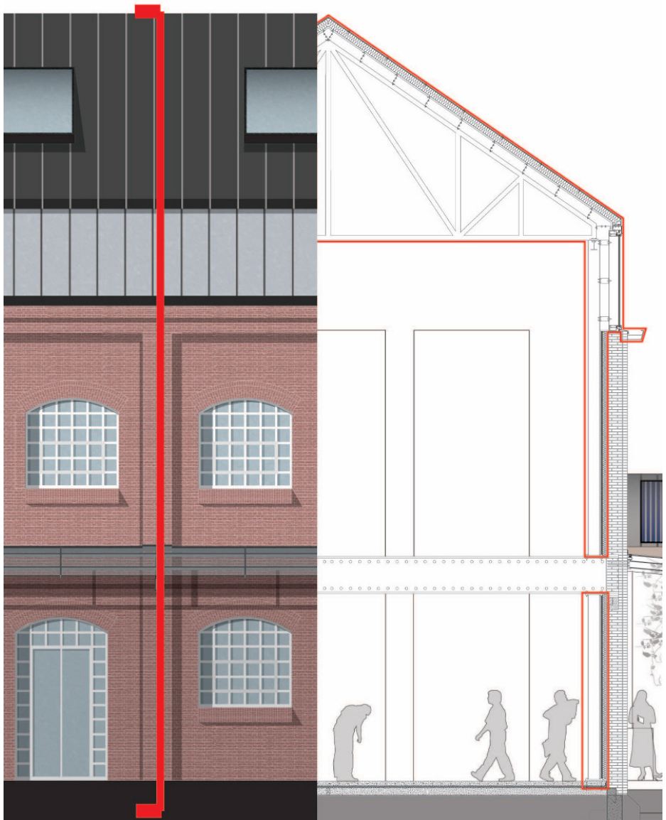
fig-33: Cathedral new insulation
