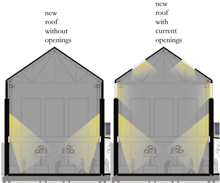
fig-47: daylighting diagram of the Cathedral
