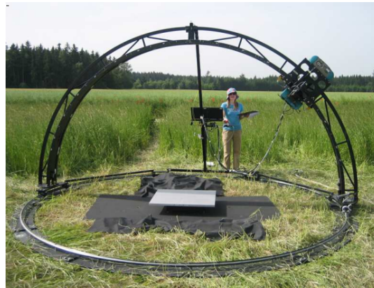
Figure 2.15: Dual-view goniometer system used to take field BRDF measurements. Adapted from [40].
