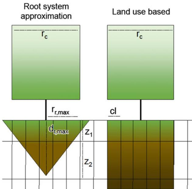
**Fig. 3** 2D-view of the applied root system approximation scheme in a raster environment. Where  $r_{c1}$  [m] is the diameter of the canopy,  $r_{r,max}$  [m] is the maximum radius of the root system,  $d_{r,max}$  [m] is the maximum depth of the root system,  $z_1$  and  $z_2$  [both m] are depths of soil layer 1 and 2 respectively and  $cl$  [m] is the length of a raster cell
