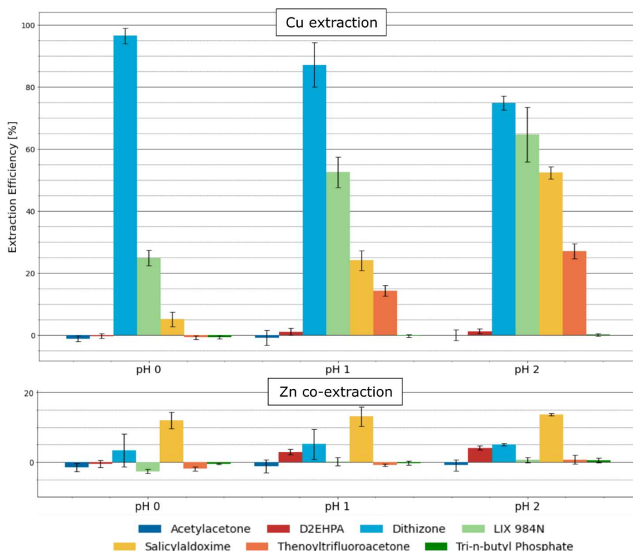
Figure 3.2: EE % of non-radioactive Cu (top) and Zn (bottom) for various chelating agents and pH values with 1 min vortexing time. All extractions were carried out with a 1 M \text{HNO}_3 solution containing 1 M \text{Zn}(\text{NO}_3)_2 and 0.1 M \text{Cu}(\text{NO}_3)_2 , and 0.2 M chelating agent in chloroform as organic phase, except for dithizone and SA. These were carried out with an aqueous solution containing 0.1 M \text{Zn}(\text{NO}_3)_2 and 0.01 M \text{Cu}(\text{NO}_3)_2 , and 0.02 M chelating agent in chloroform as the organic phase. Reported uncertainties represent one standard deviation of the mean ( n=3 ).
