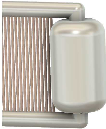
Figure 5.4: Visual representation of how the chosen catalyst bed dimensions could look like in practice.
