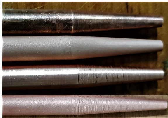
Figure 3.10: Photograph of the four conical support preparations. From top to bottom: Smooth, Sandblasted, Grooved, Grooved and Sandblasted.
