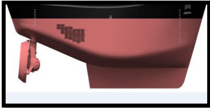
Figure 28: Vertical Lengthy Skeg in ASD's (Laan 2016, 1)
