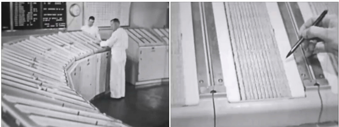
Figure 5.23 Monitoring station with live spectrogram plotting of underwater Sound Surveillance System (SOSUS) hydrophone seabed array on facsimile spectrograph plotters. Stills from "Watch in the Sea: Project Caesar", Navy and Marine Corps Productions 24458-DN, c. 1960.
