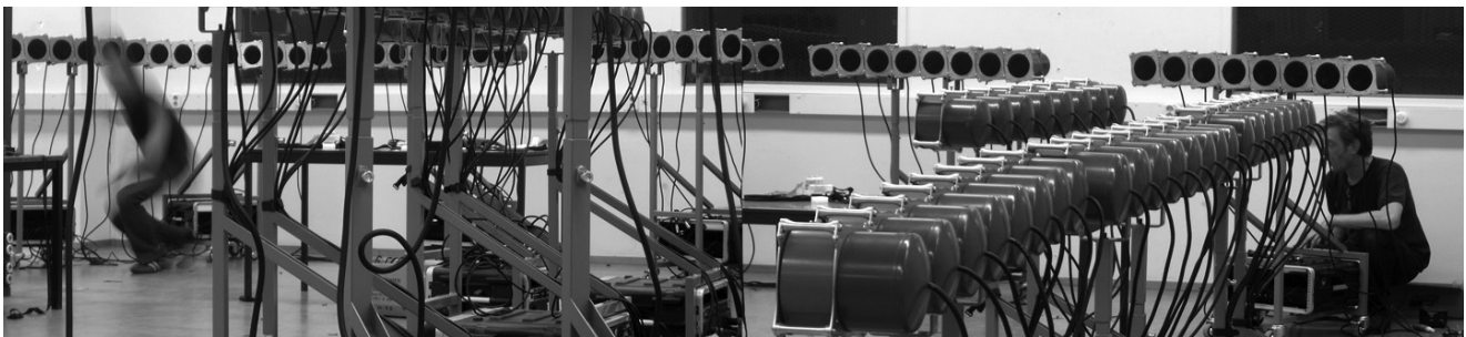
Figure 4.4 Wave Field Synthesis acoustic rendering setup, 192 loudspeaker array (Author's design)
