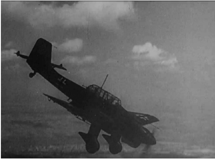
6.29 Propeller-driven sirens fitted on the main gear legs of the Luftwaffe dive-bombers, widely known as Jericho-Trompete (Jericho trumpet), accentuated plane dives with a distinctive wailing noise that become the signature sound of the German Blitzkrieg. Similar mechanical sirens can be found today in early-warning air-raid systems common to city infrastructures. Film still from a Luftwaffe dive-bomber sequence in The Battle for Oil (dir. S. Legg, 1942), National Film Board of Canada.
