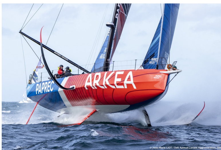
Figure 1.1: Fully foiling IMOCA 60 (Defi-Azimut, 2024)
