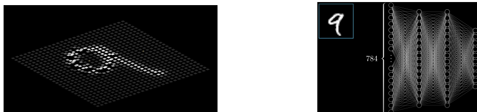
(a) Representation of the number "9" of the MNIST data-set [8]. (b) Feeding the 784-pixel vector to a neural network [9].
