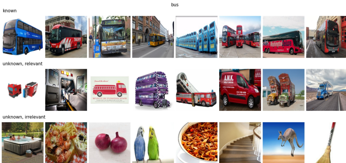
Figure 1.5: Based on examples of a relevant, known class (e.g., 'bus' - top row), our method can classify test images as either known or unknown, where the unknowns are divided into relevant (other vehicles, middle row) and irrelevant (non-vehicles, bottom row).
