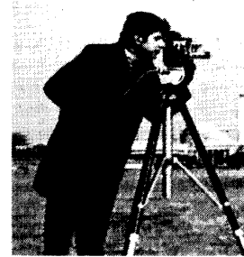
Fig. 27. Constrained adaptive restoration of the defocused cameraman image with noise added (SNR = 40 dB). SNR improvement is 8.1 dB.
