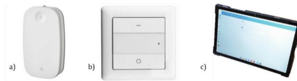
Fig. 4. Types of device interfaces used in the experiment: (a) analog light switch, (b) analogue roller shade switch, and (c) tablet interface controlling both lights and roller shades.
