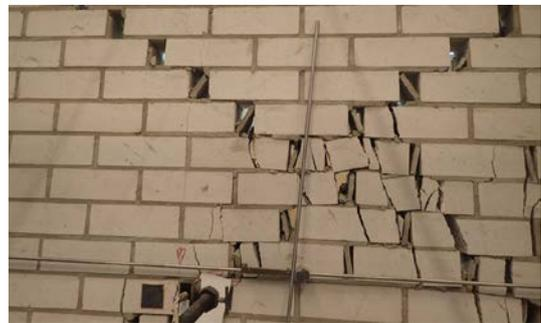
Figure 21. Example of experimental tensile, shear and compression (splitting) modes (Ravenshorst & Messali 2016a) to be reproduced numerically.
