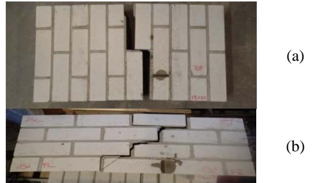
Figure 2. Crack patterns of calcium silicate masonry specimens subject to: (a) out-of-plane vertical bending test; (b) out-of-plane horizontal bending test (Esposito et al., 2016).
