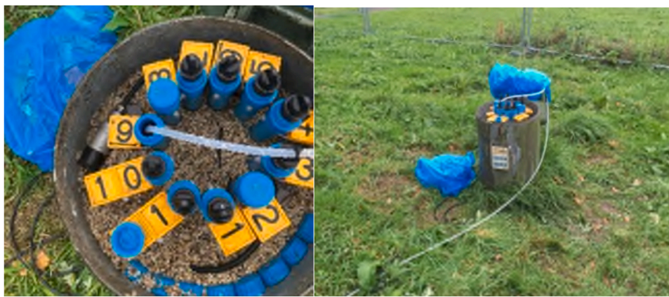
Fig. 2. The observation well that is used for the extraction of water for this experiment.
