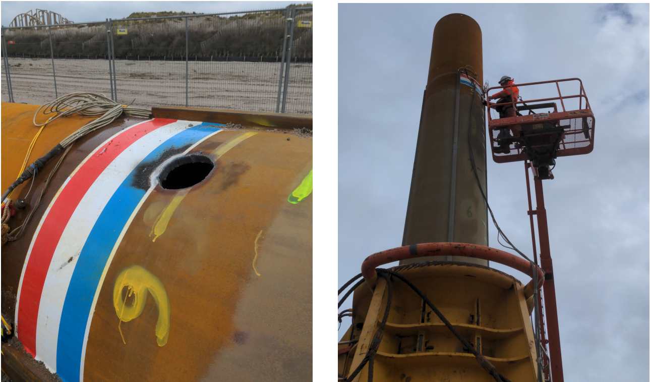
Figure 33: (a) Hole burnt in the pile around 9 meter (from pile tip) mark (b) Performing plugging measurement from aerial work platform
