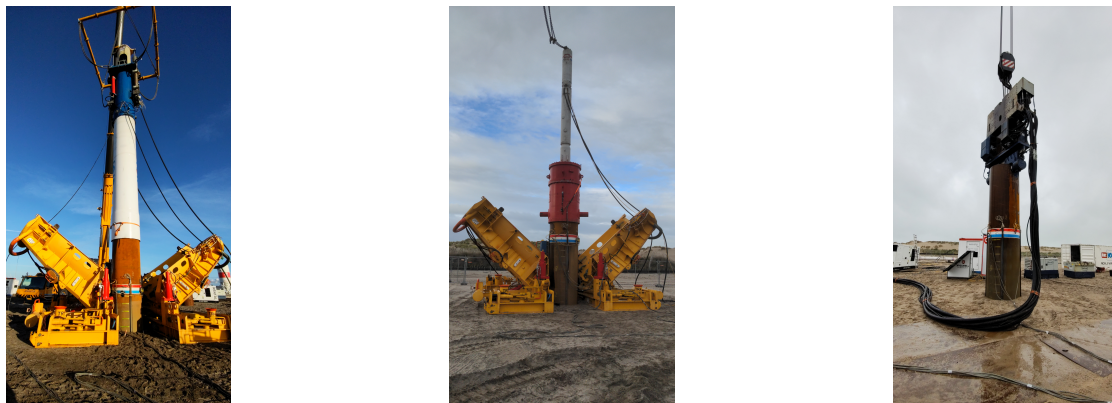
Figure 32: Test set-up of (a) Blue Piling Hammer (b) Hydro Hammer and (c) Vibratory driver
