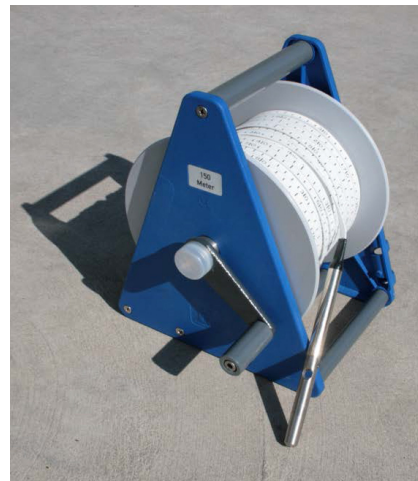
Figure 30: (a) Measuring the pile plug with respect to ground level (b) Used device (Tecso, n.d.)
