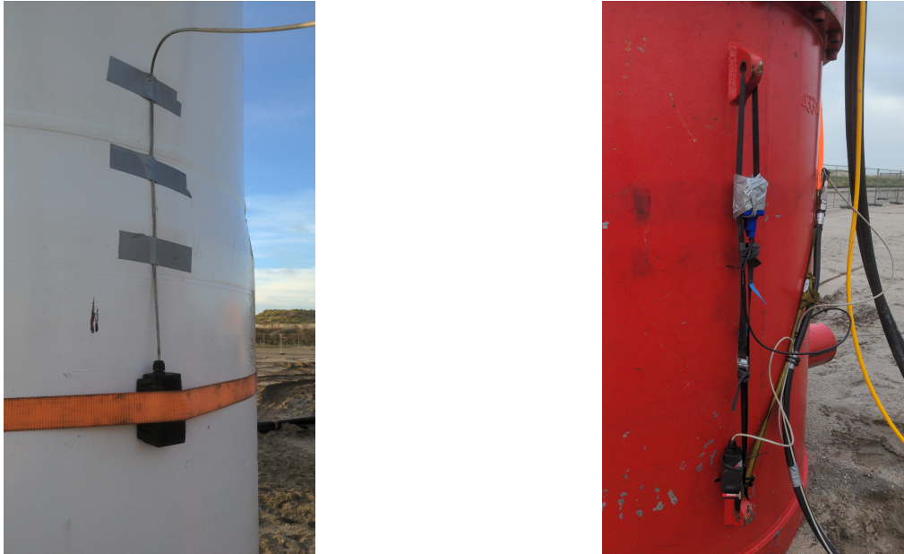
Figure 28: Laser displacement measurement installed on (a) the Blue Piling hammer (b) the S-30 Hydrohammer
