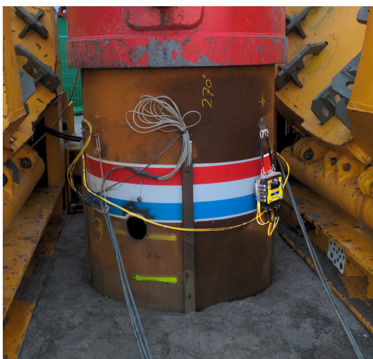
Figure 23: PDA (a) Receiver connected to module on 0° and 180° (b) Full bridge strain module with accelerometer
