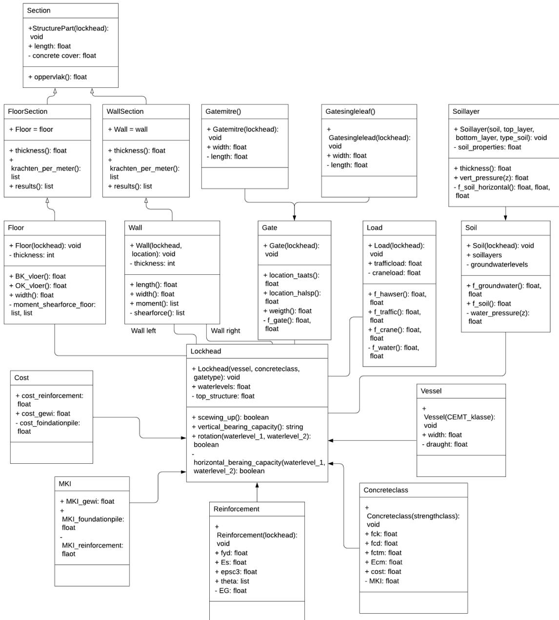
Figure 7.1: UML diagram of the parametric model
