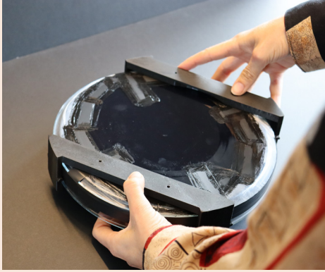
Placing the holders around the Petri dish
