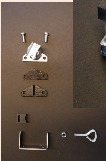
Fabricating a tilt lock on the tilt mechanisms to fixate the orientation of the Petri dish
