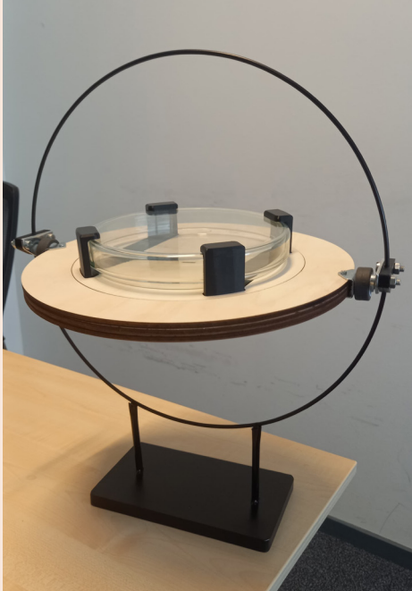
The first prototype with the Petri dish on top of the rotation disc, resulting in balance issues
