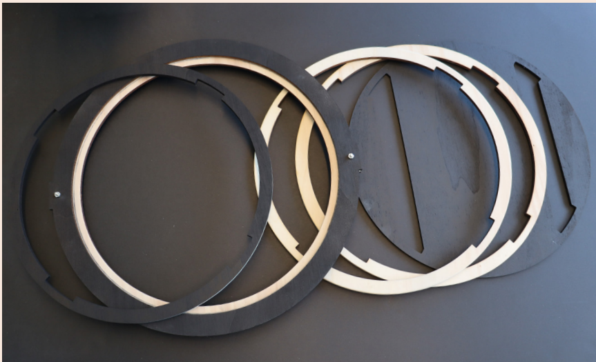
The layers of the rotation disc, enabling rotation while securing the Petri dish
