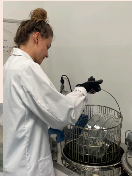
Sterilisation of Petri dishes in the autoclave
