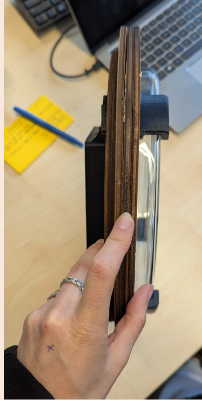
Redesigning the rotation disc to resolve balance issues by centring its centre of gravity
