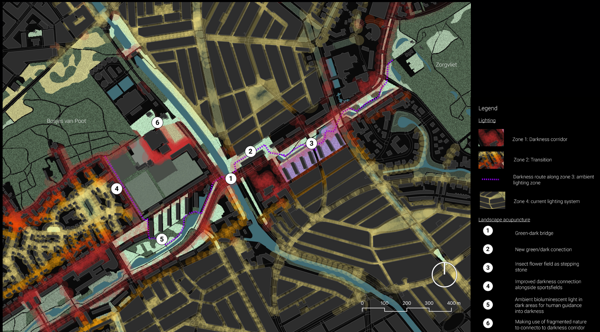
Figure 4.8. The design includes a warm-colored darkness corridor to minimize disturbance to nocturnal life, transition zones to gradually shift from a white to red spectrum, a new nocturnal flower meadow, and stronger green-blue-dark connections for animals and human experience. Overall, the design aims to improve the human experience at night and to create a more ecologically friendly nocturnal landscape through lighting zones and new interventions, based on the developed guidelines illustrated in this report
