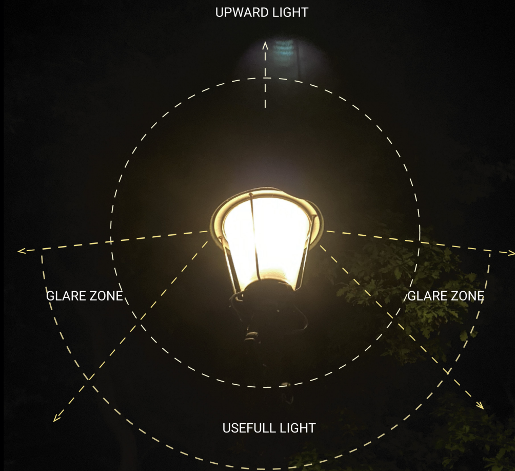
Figure 3.12. The effects of a single streetlight at night. Made by author
