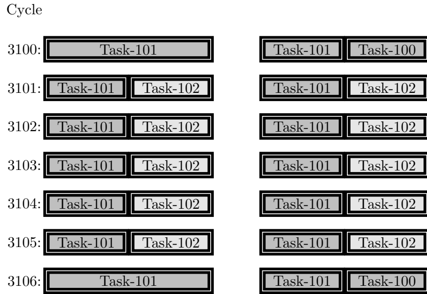
Figure 3.7: GB stealing resources from a task(left) or freezing it (right).
